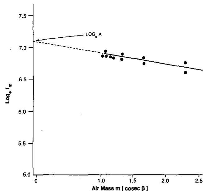
Fig. 1. Direct normal intensity as a function of air mass for each clear day.
