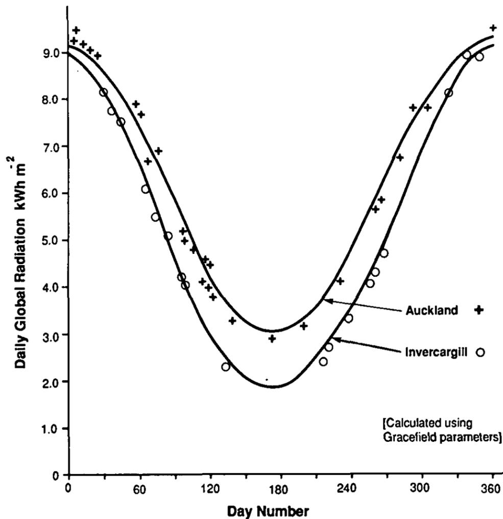
Fig. 4. Estimated and measured daily global radiation on the horizontal for Auckland and Invercargill.
