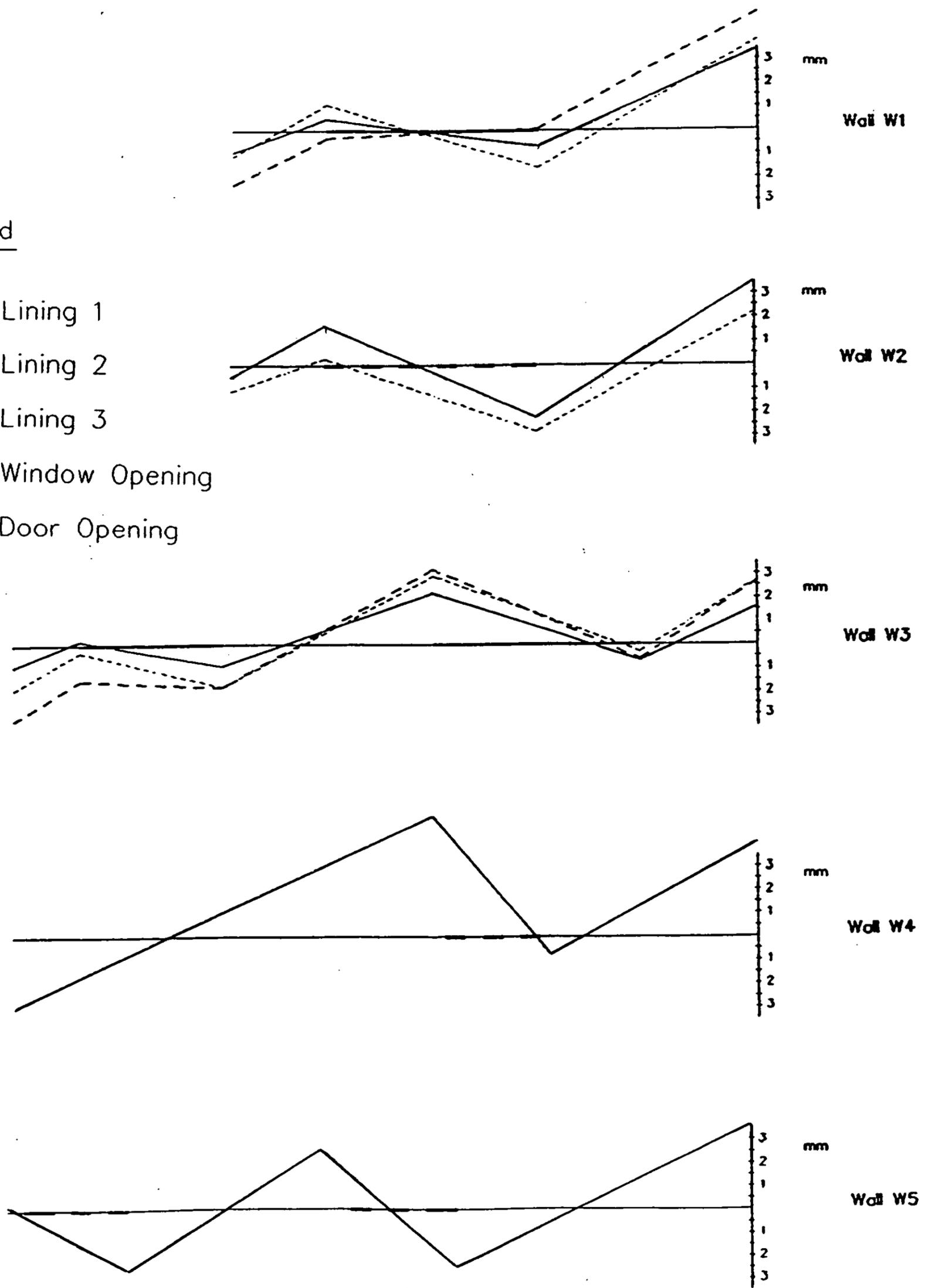
FIGURE 4 Wall Uplift Deflection Profiles
