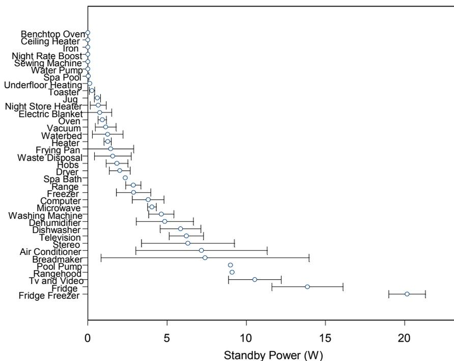
Figure 5. Average standby power of various appliance types. Error bars are  $\pm 1$  standard deviation.
