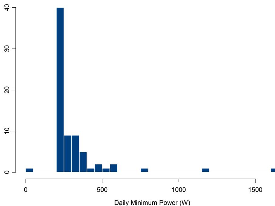
Figure 4. Example of baseload estimate. Baseload estimated at 215 W.
