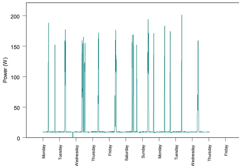
**Figure 1. Washing Machine example of Standby Power.**
