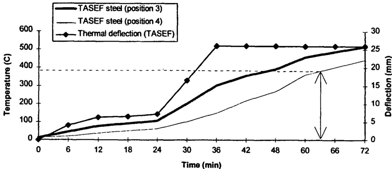
Figure 19. Predicted steel temperatures and thermal deflection (test 1).
