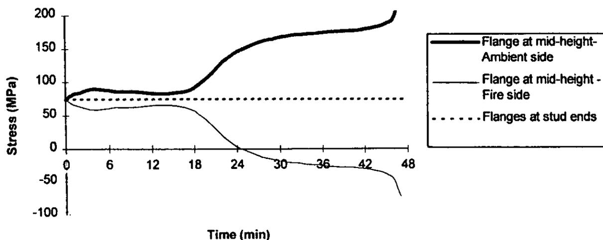
Figure 17. Variation in steel stud stresses with time for test 2.
