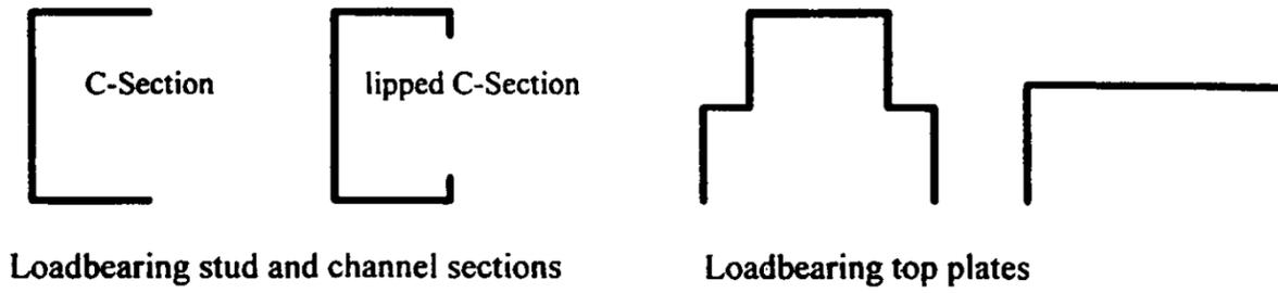
Figure 2. Common steel framing sections.
