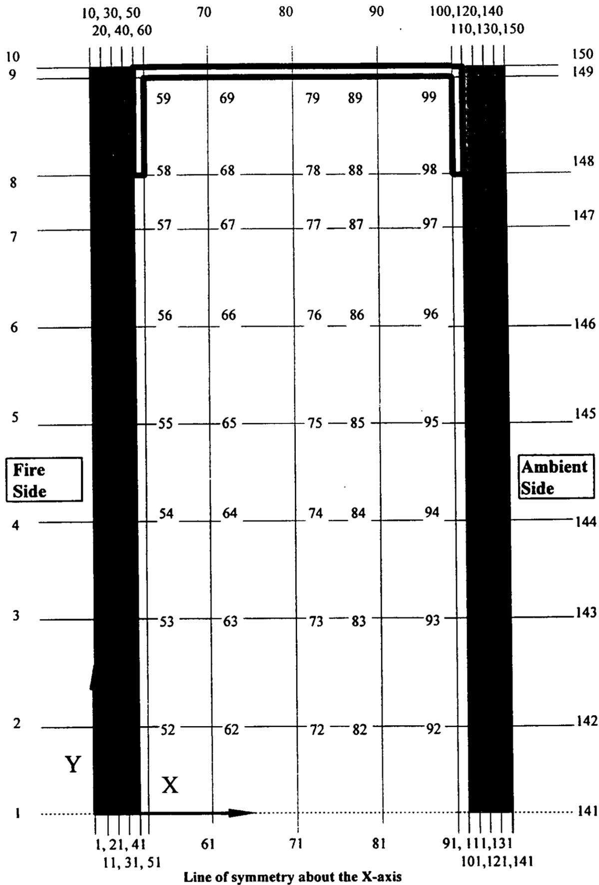
Figure 10. Typical finite element mesh for the thermal model using TASEF.
