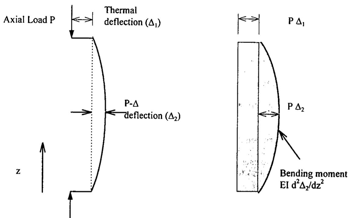
Figure 8. Total horizontal deflection for load-bearing systems.
