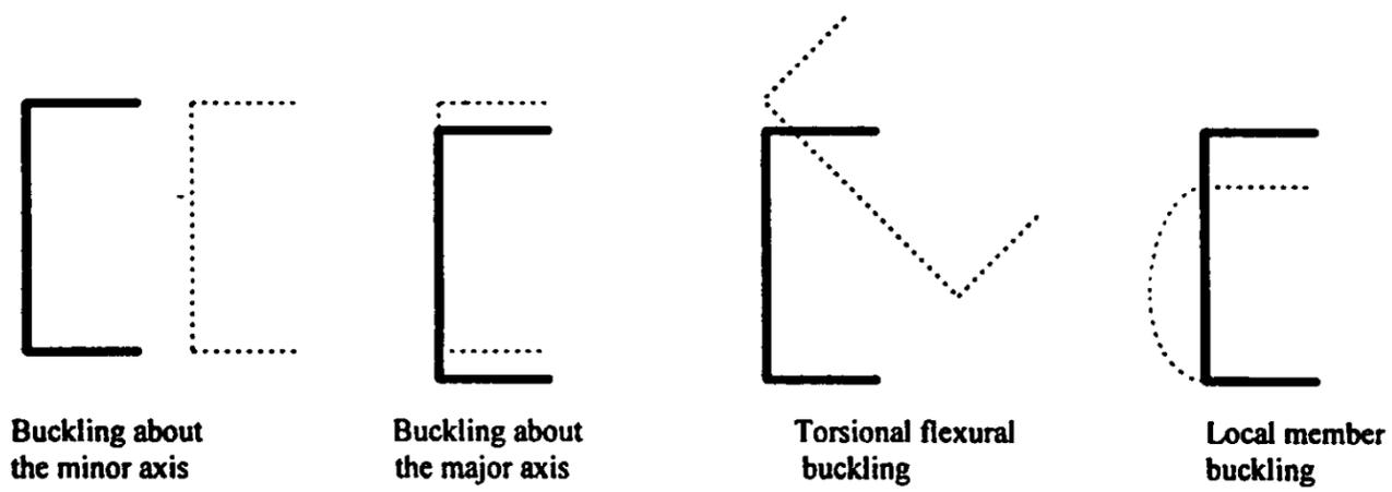
Figure 4. Buckling modes of cold-formed steel members.
