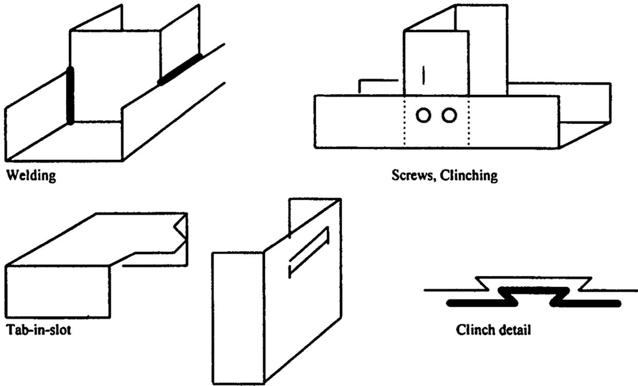
Figure 3. Typical stud to channel connections.
