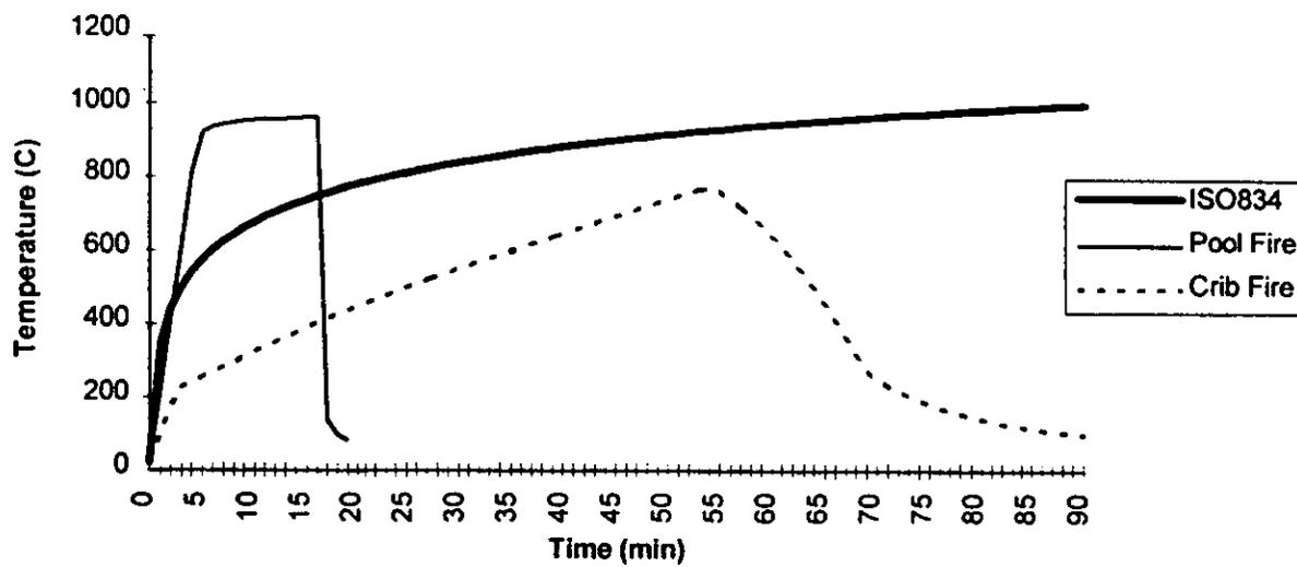
Figure 1. Comparison of possible real fires with the standard ISO 834 curve.
