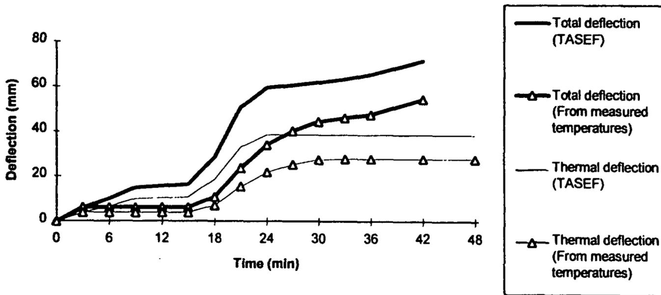
Figure 18. Comparison of calculated horizontal deflections based on TASEF and measured temperatures (test 2).
