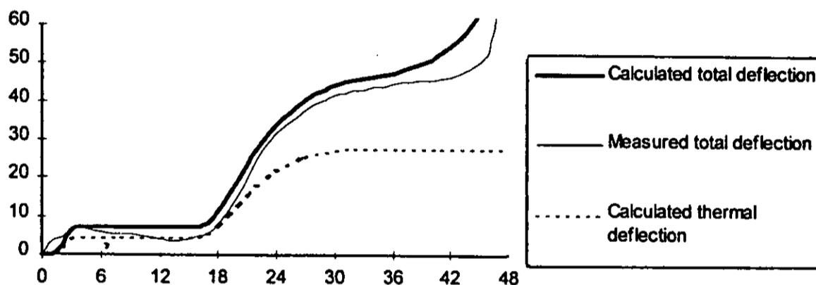
Figure 9. Comparison between calculated and measured horizontal deflections (test 2).
