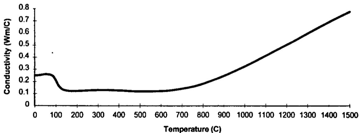
Figure 6. Thermal conductivity of gypsum plasterboard.
