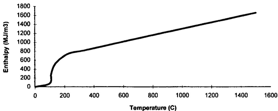
Figure 7. Specific volumetric enthalpy of gypsum plasterboard.
