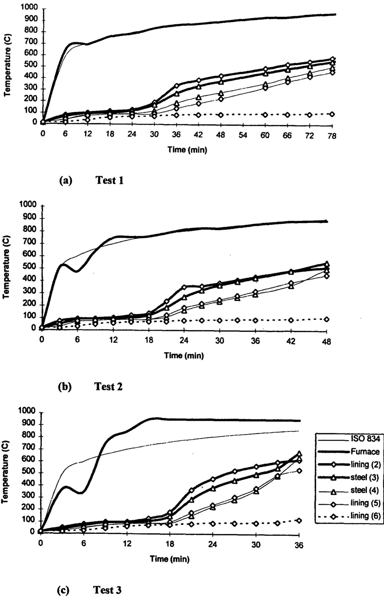
Figure 14. Measured temperatures within full-scale test specimens (numbers in brackets indicate temperature measurement position in accordance with Fig. 11).
