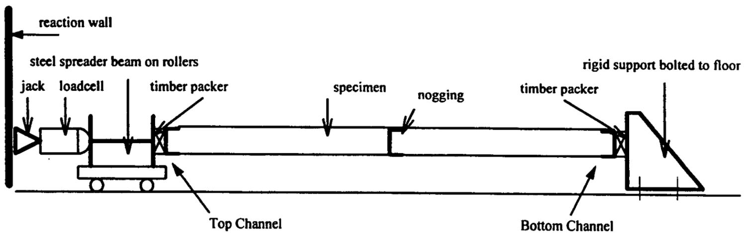
Figure 5. Test set-up for combined axial loading and bending.
