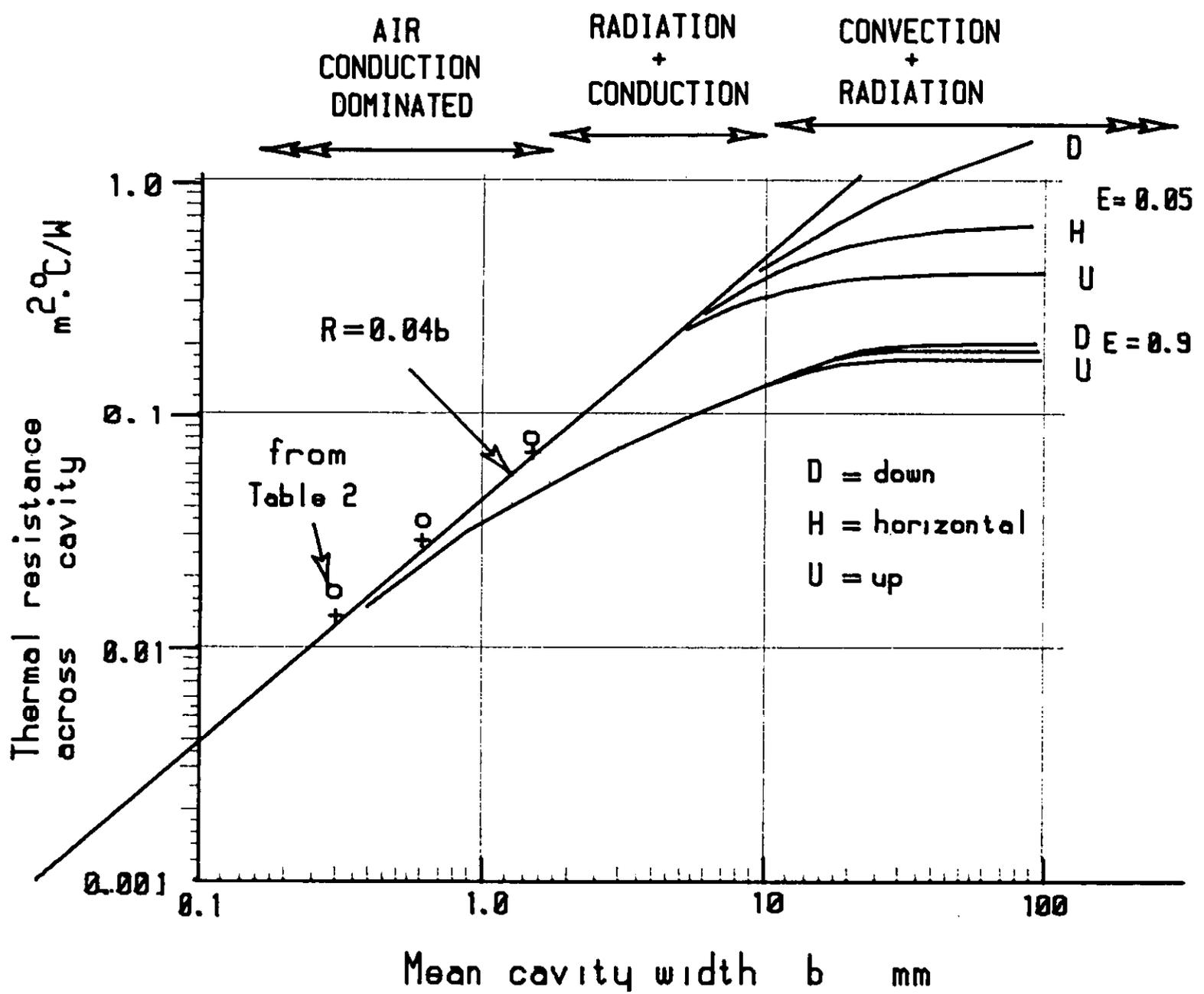
Figure 8 Thermal resistance across small cavities
