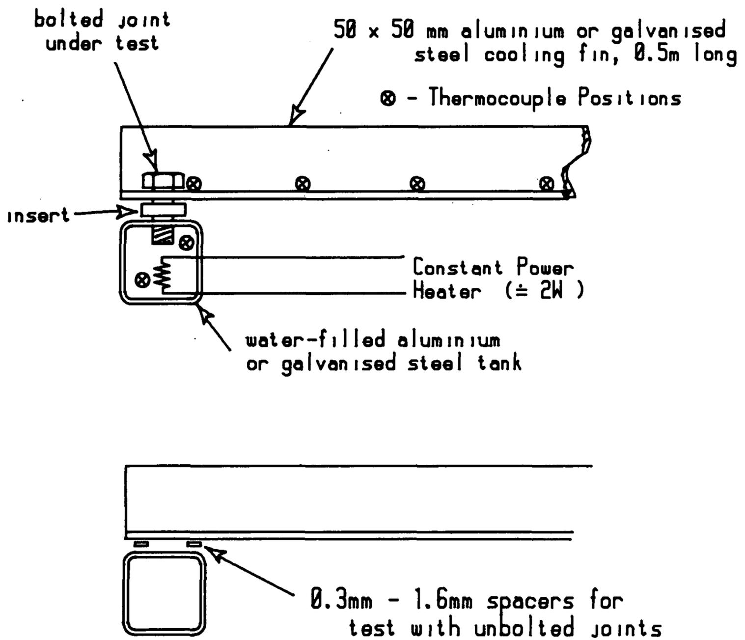
Figure 9 Sketch of equipment for test of contact resistance of joints
