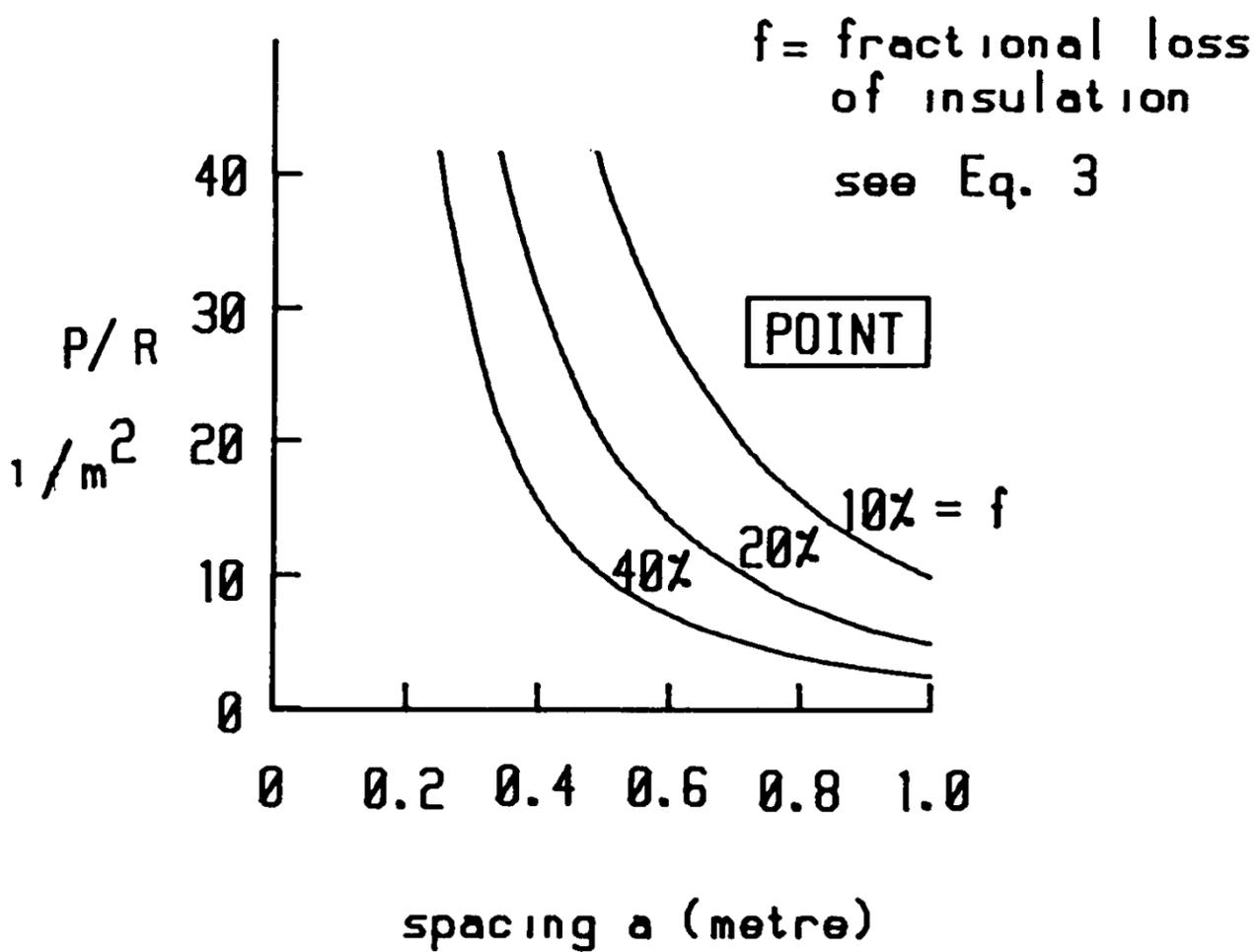
Figure 7 Joint resistance corresponding to various loss of insulation
