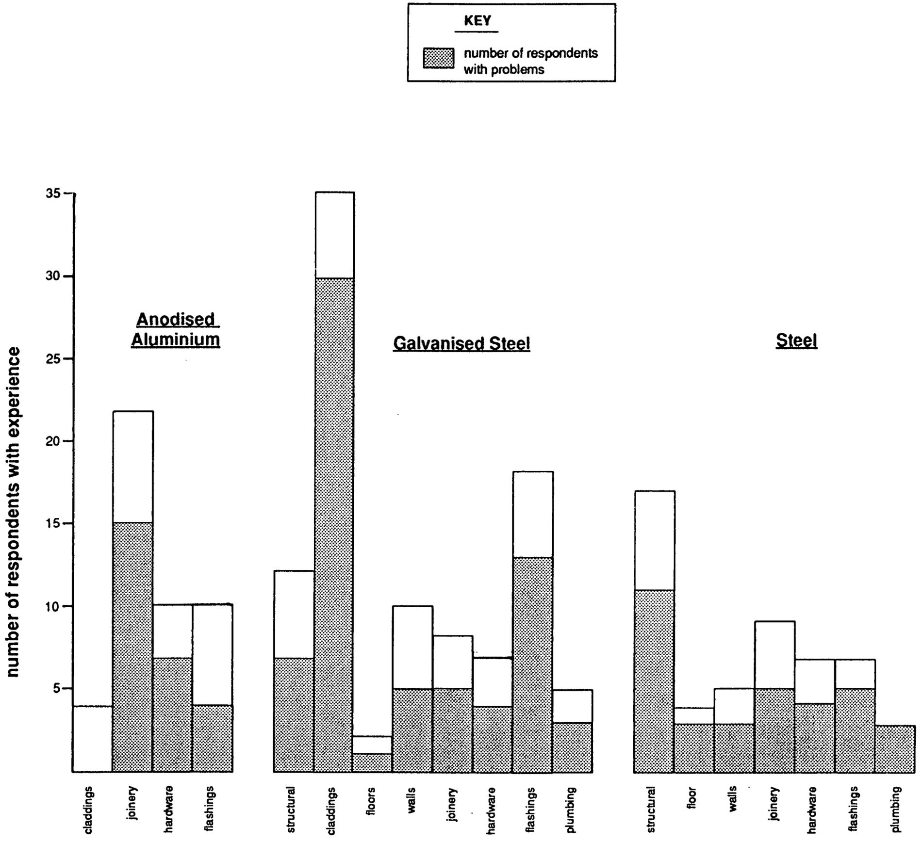
**Figure 2: Number of respondents claiming experience and problems with anodised aluminium, galvanised steel and steel**
