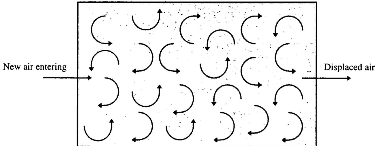
FIGURE A4: Fully mixed air in a space representing dilution ventilation.
