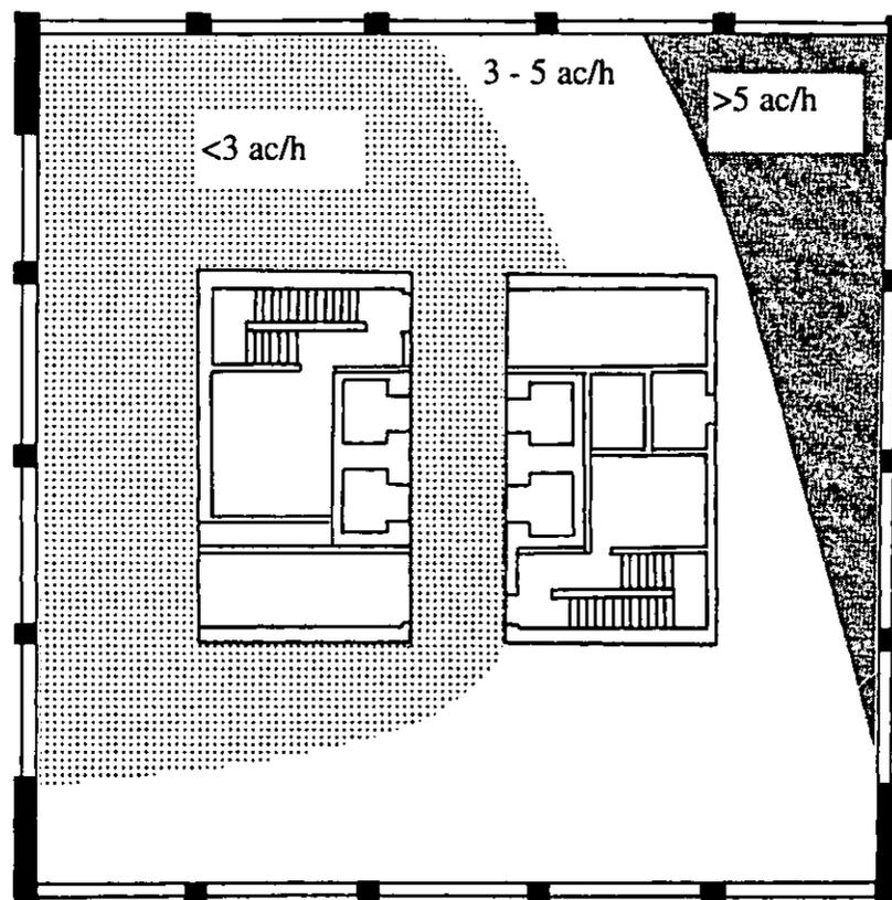
FIGURE 3: Approximate contours of effective ventilation rate in the breathing zones of building E.
