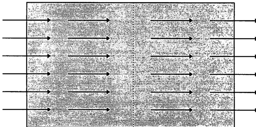
FIGURE A3: Displacement flow of air through a ventilated space.
