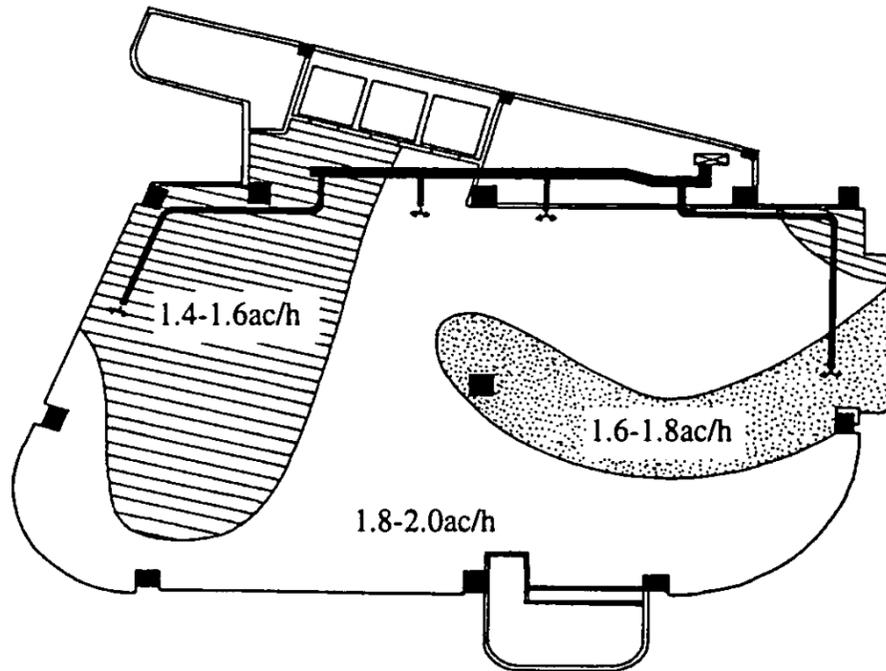
FIGURE 4: Approximate contours of effective ventilation rate in the breathing zones of building G.
