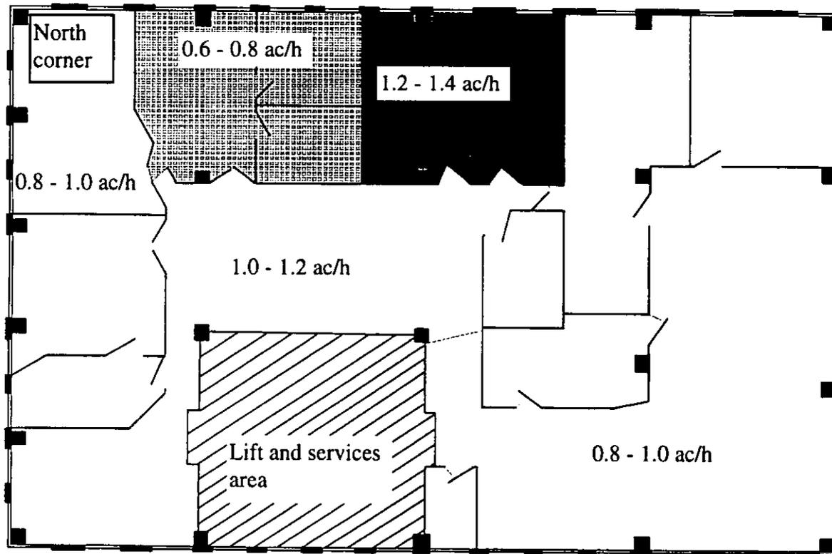
FIGURE 2: Approximate contours of effective ventilation rate in the breathing zones of building D level 6.
