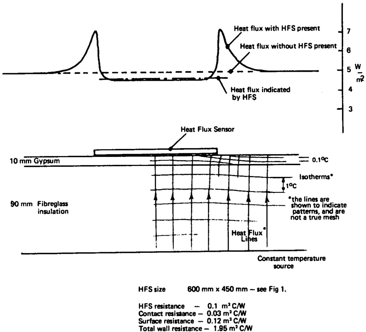
FIG. 2—Heat flow around a heat flux sensor (see Fig. 1) from a finite difference model.
