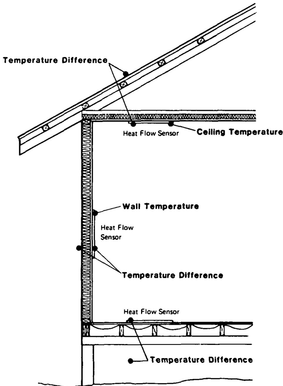
FIG. 1—The placement of sensors for the survey of in situ R-values.
