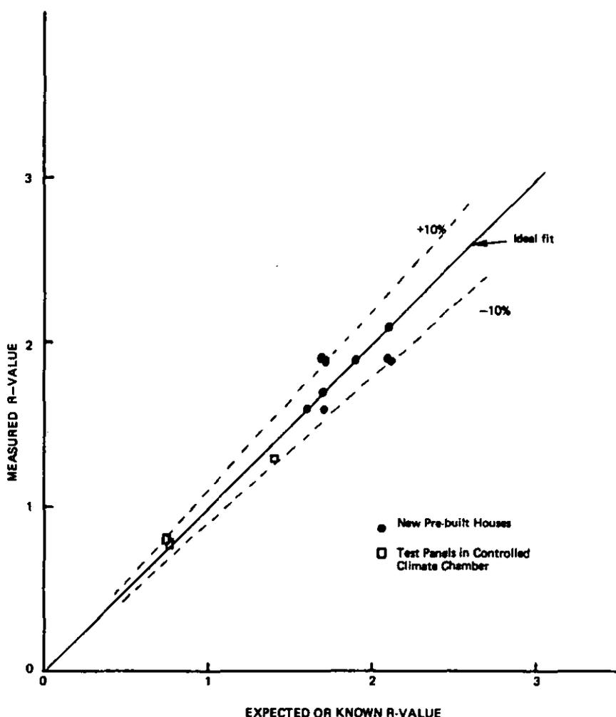
FIG. 3—The results of the tests showing the reliability of the survey procedures.
