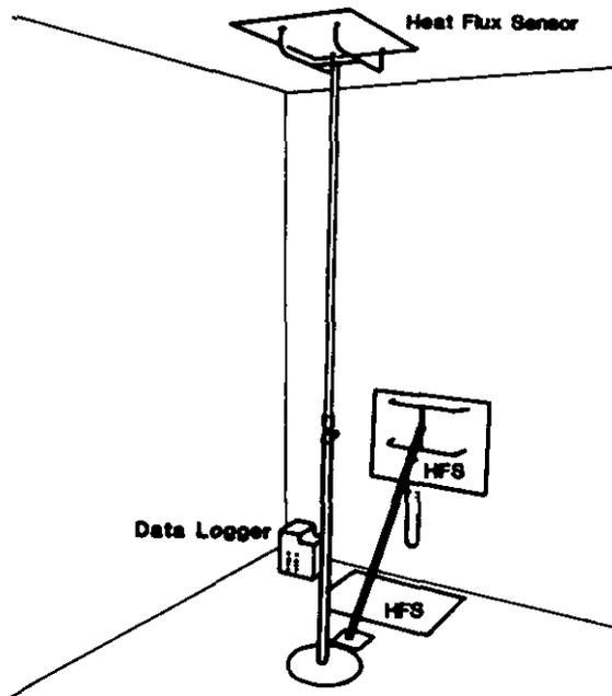
FIG. 2—The physical installation arrangement of equipment for the survey.
