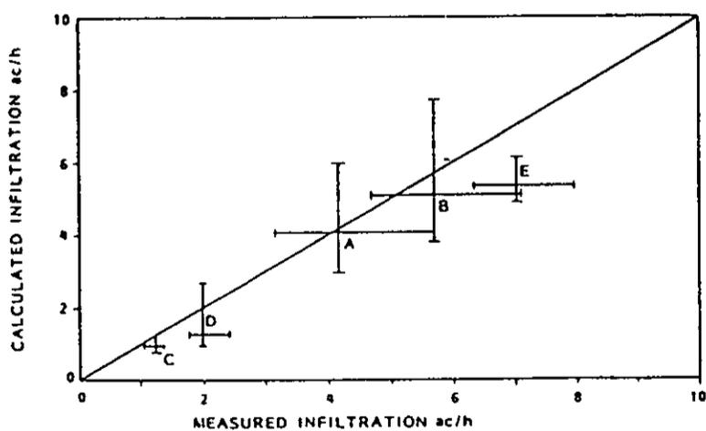
Figure 9 Mean measured and calculated infiltration in subfloors of five houses, A-E, survey 3 (from Bassett 1990).
