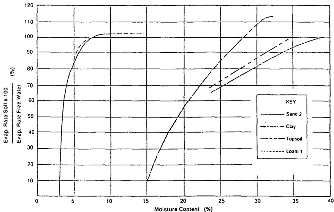
Figure 5 Relative evaporation rates over moist soils (survey 2).
