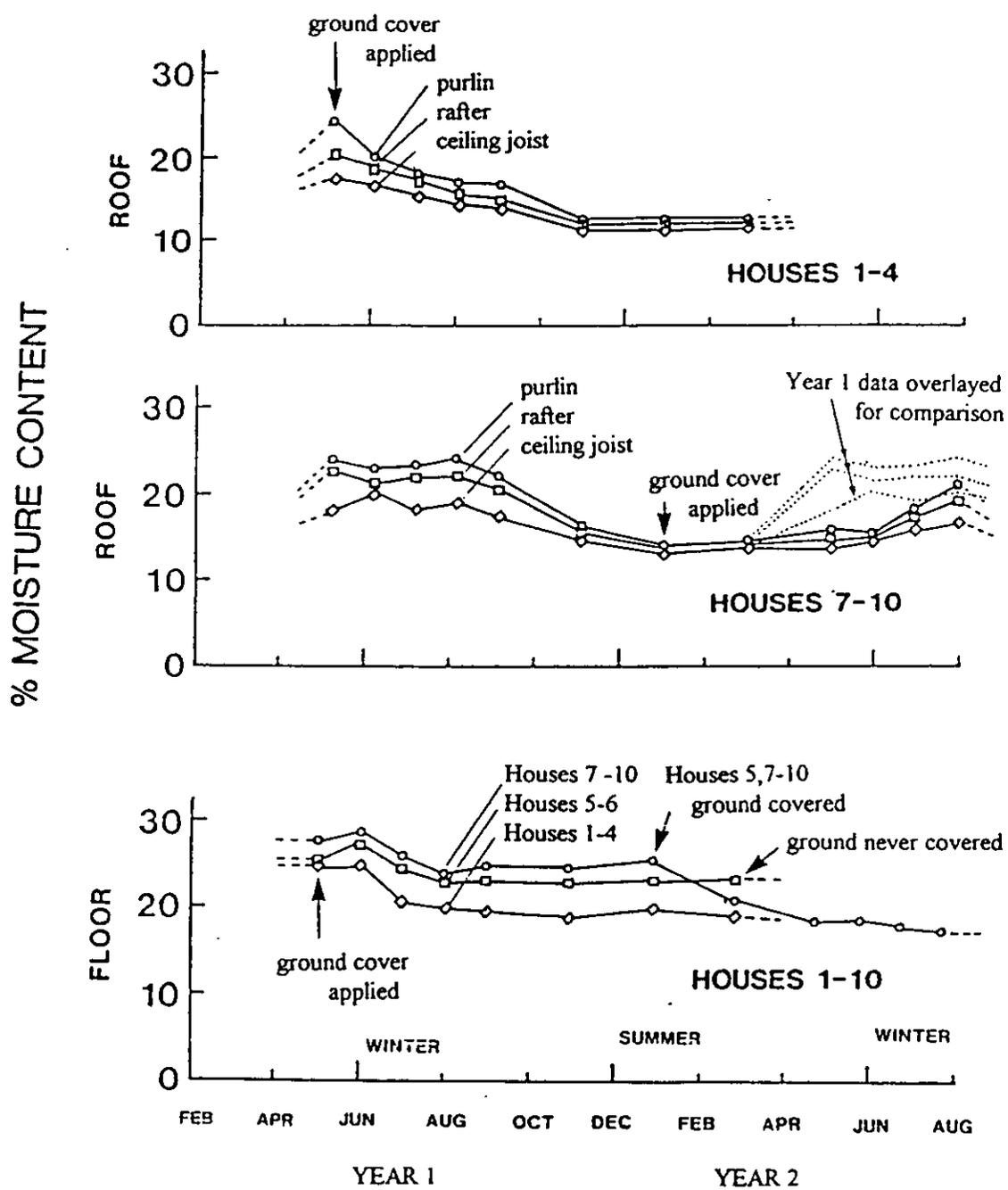
Figure 4 Average roof and floor timber moisture content (survey 1).
