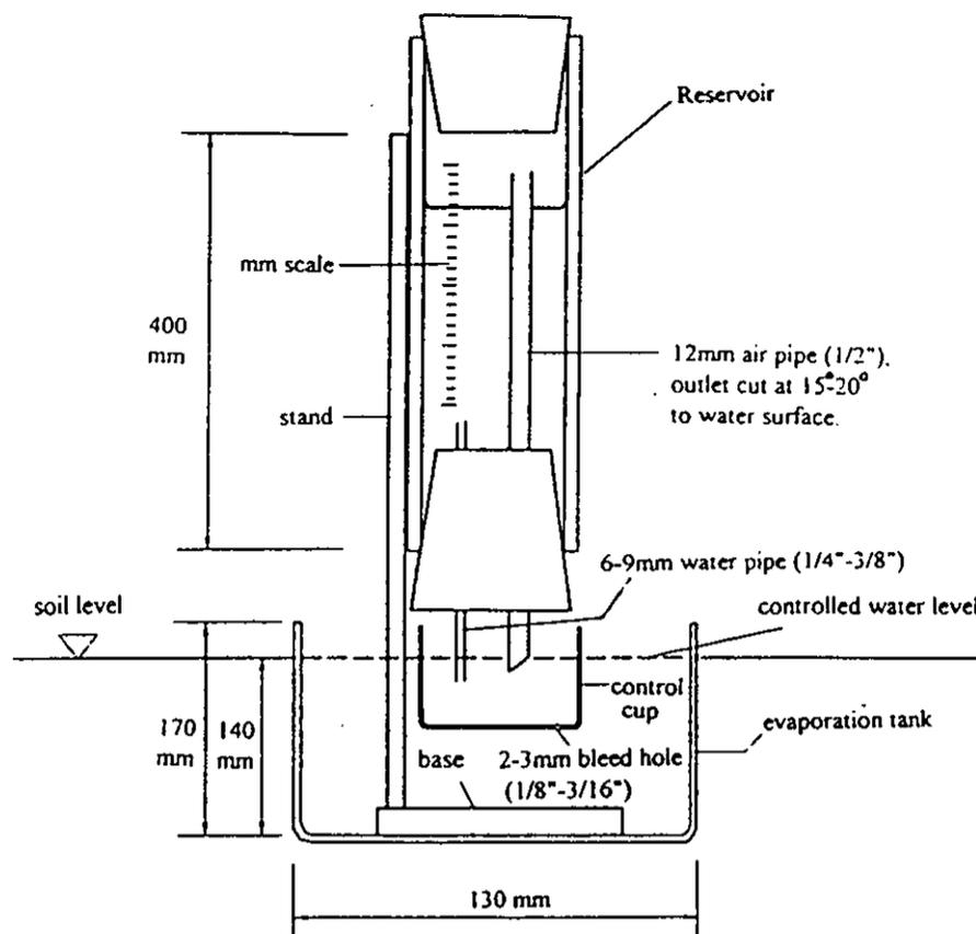
Figure 6 Details of "bird-bath" free-water lysimeter (survey 2).
