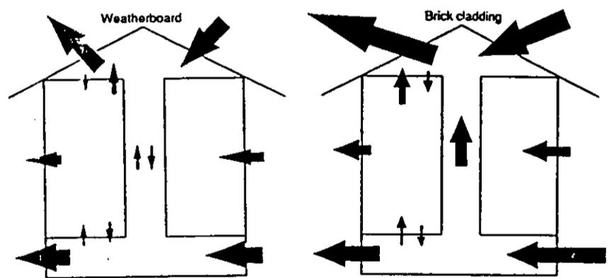
Figure 10 Approximate interzonal airflows in five houses, A-E, survey 3. The shaft through the center of the house represents the leakage paths that bypass the living space. The magnitude of the airflow is indicated by the arrow size (from Bassett 1988). See also Table 3.
