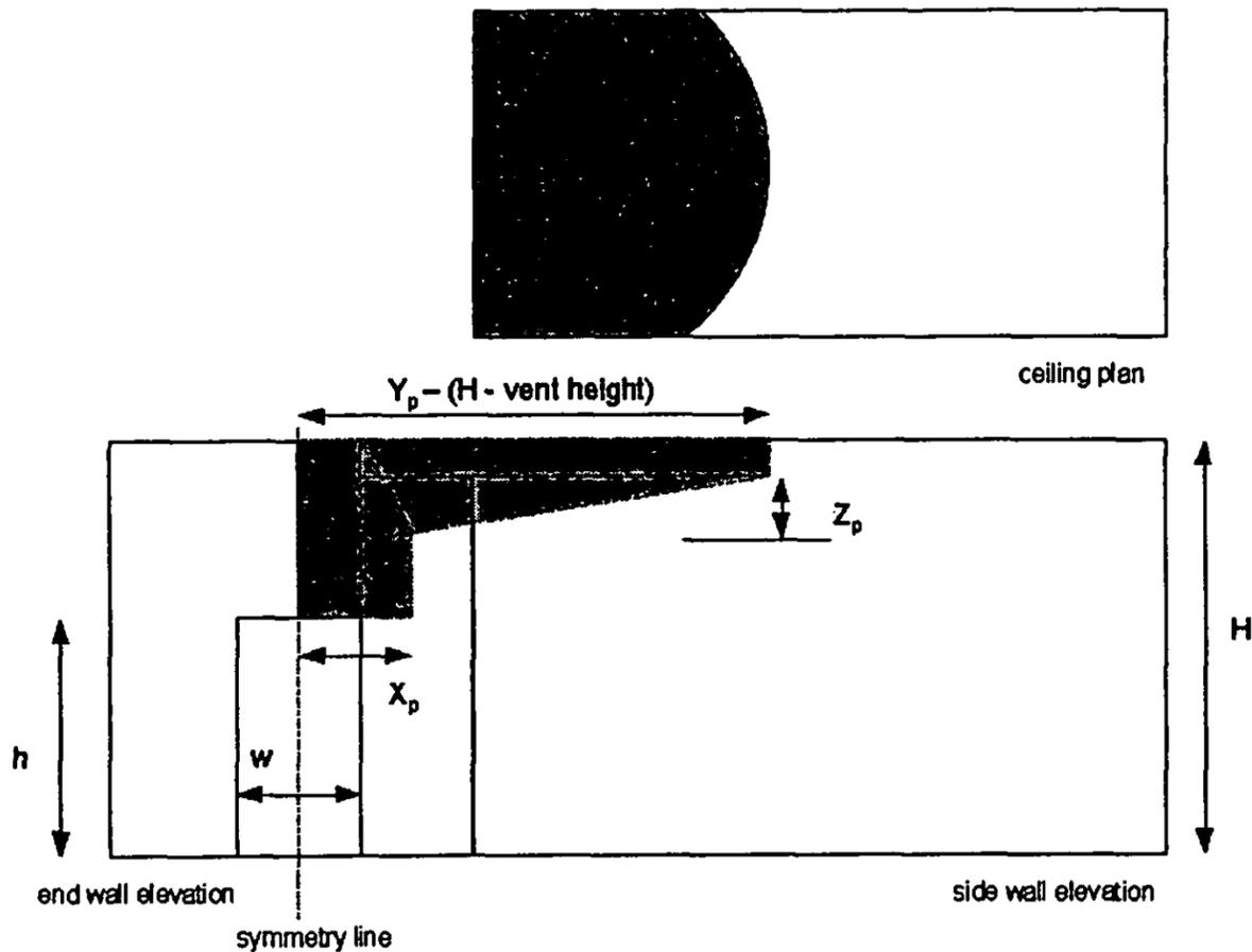
Figure 3: Wall above the vent has ignited; pyrolysis front has reached ceiling.
