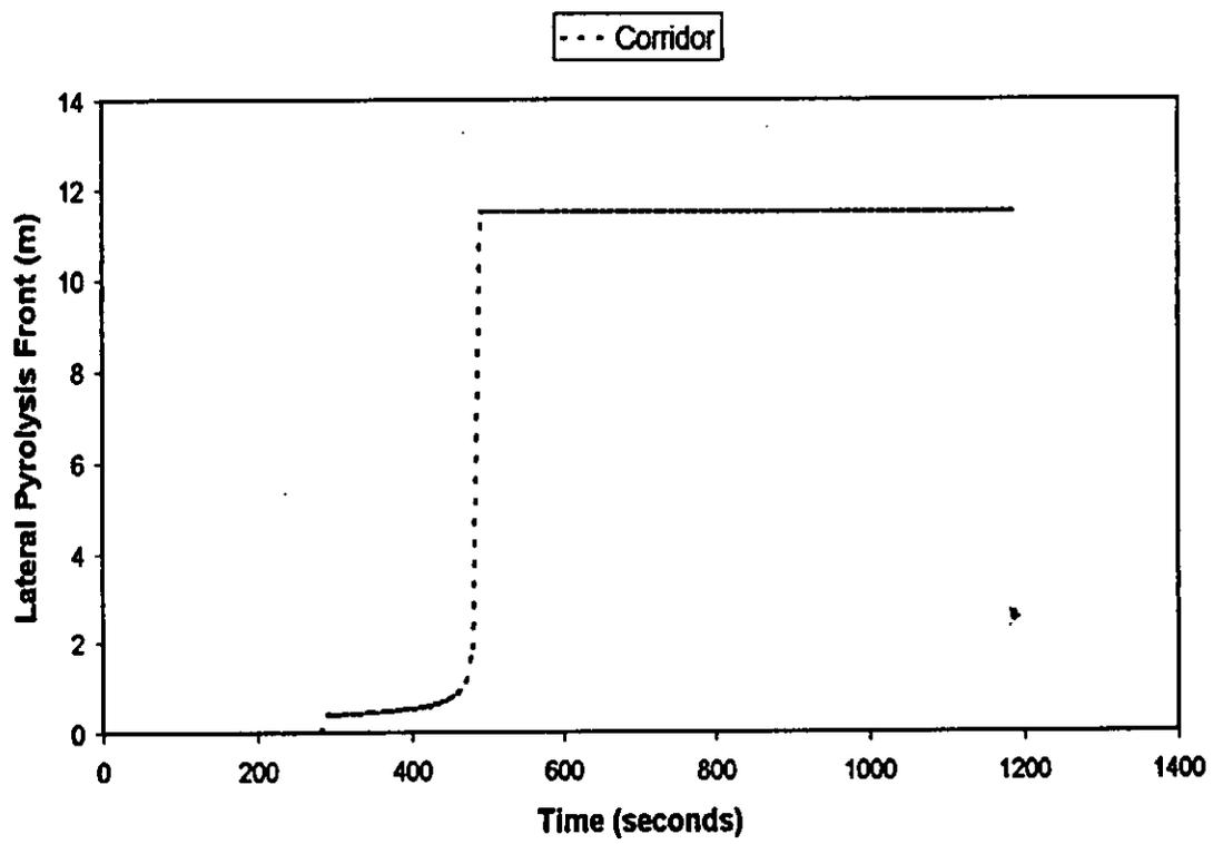
Figure 8: Position of lateral pyrolysis front in corridor.
