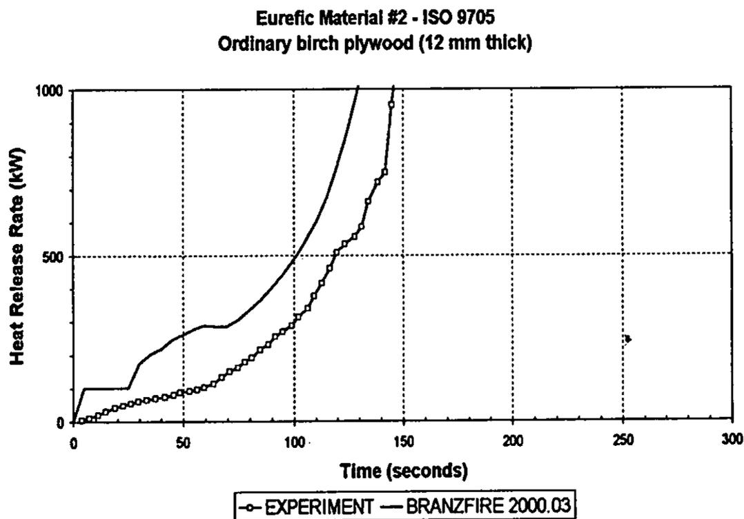
Figure 5: Heat release rate in standard ISO 9705 room corner test.
