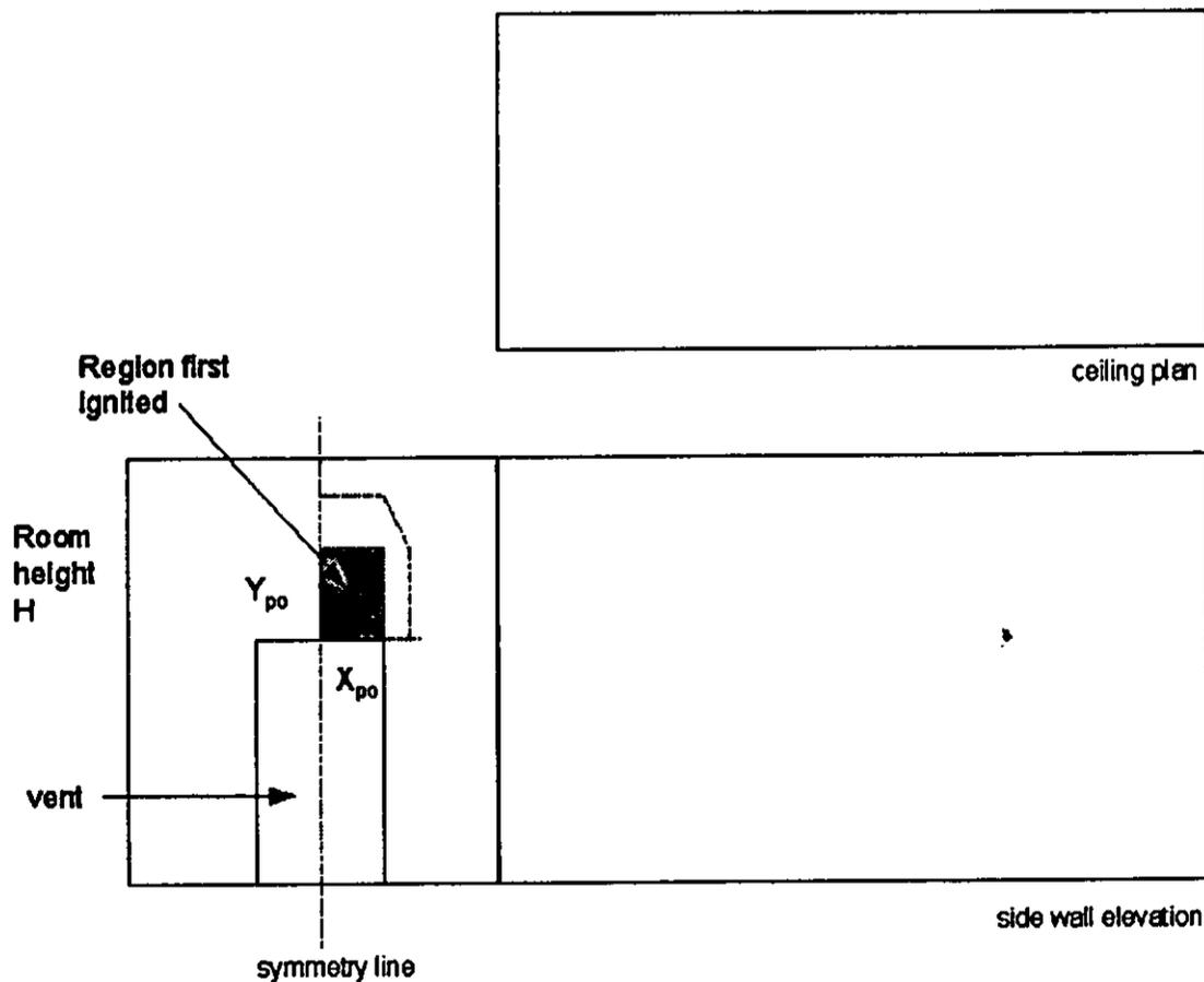
Figure 2: Wall above the vent has ignited; pyrolysis front not yet reached ceiling.
