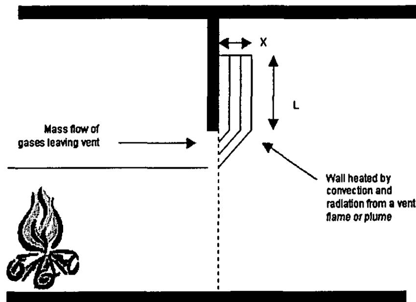
Figure 1: Flame dimensions for fire spread into an adjacent space.
