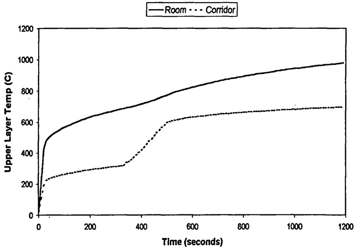
Figure 9: Upper layer temperature in room and corridor
