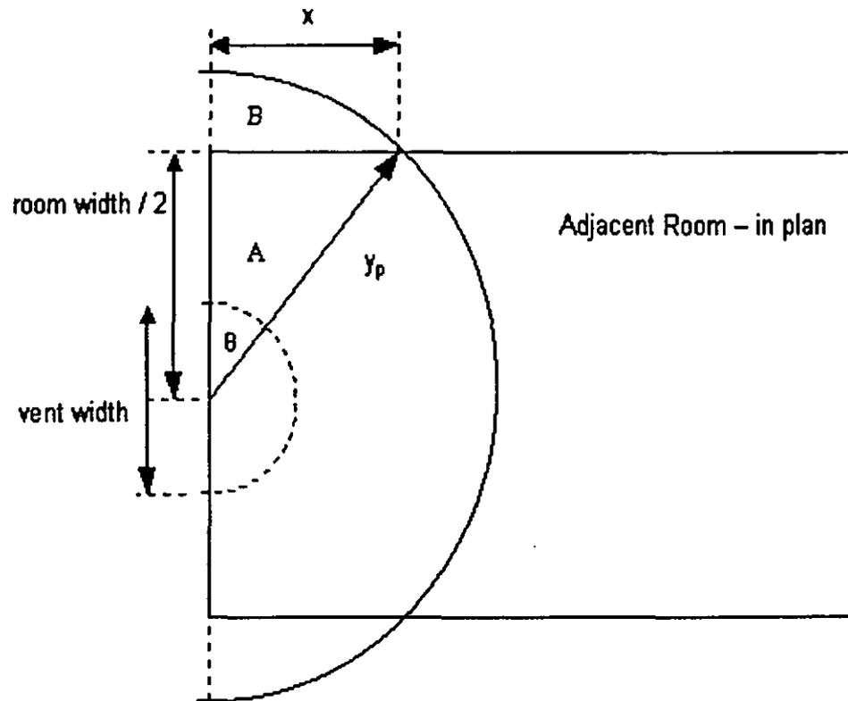
Figure 4: Pyrolysis front on ceiling in adjacent room or corridor.
