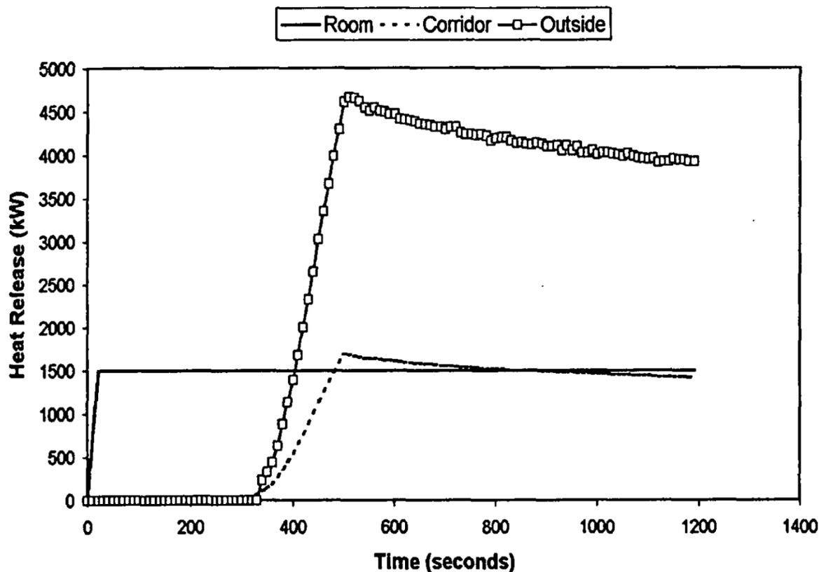
Figure 6: Heat release rate in room and corridor.
