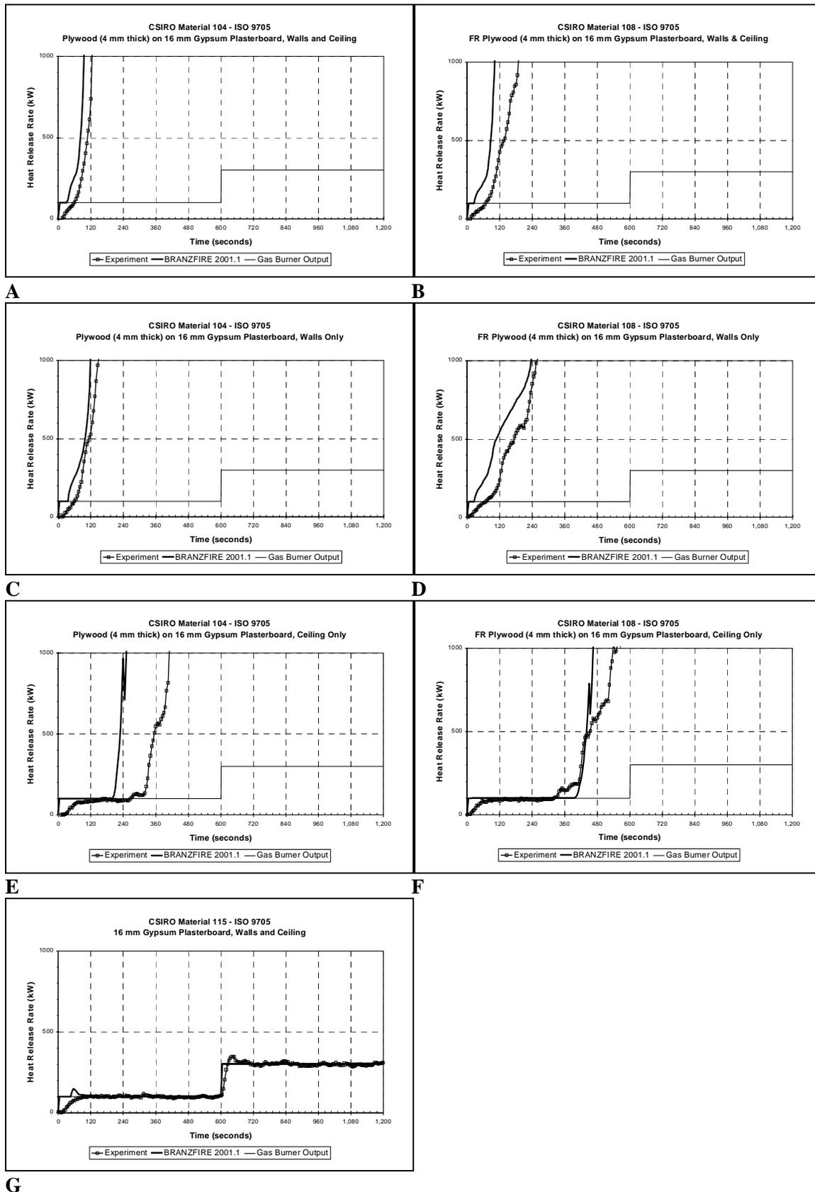
Figure 3: Comparison of Predicted and Measured Heat Release Rates from CSIRO Experiments
