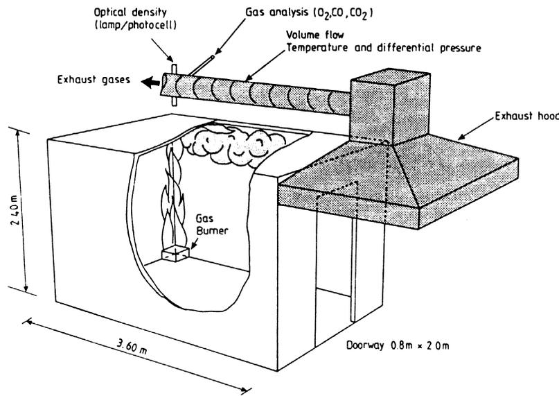
**Figure 1: The Standard Room Fire Test – ISO 9705**
