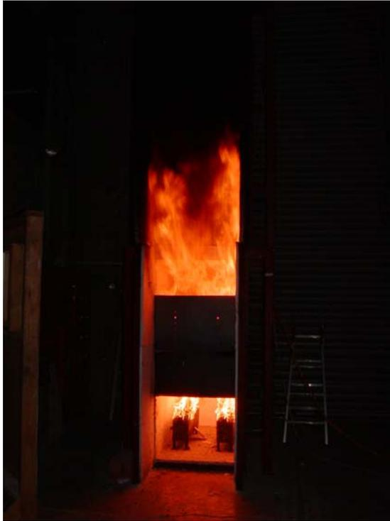
**Figure 5-10: Photograph of typical fire plume with extensions observed towards each side of the channel.**
