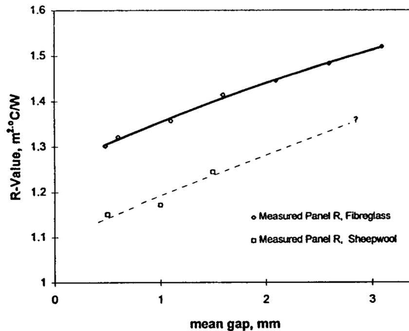
FIGURE 4. Measured R-Values at various mean contact gap (one face varied).
