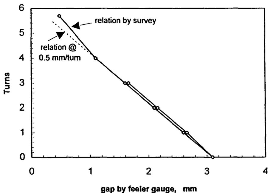
FIGURE 2. Calibration of screw turn control v thickness by survey.
