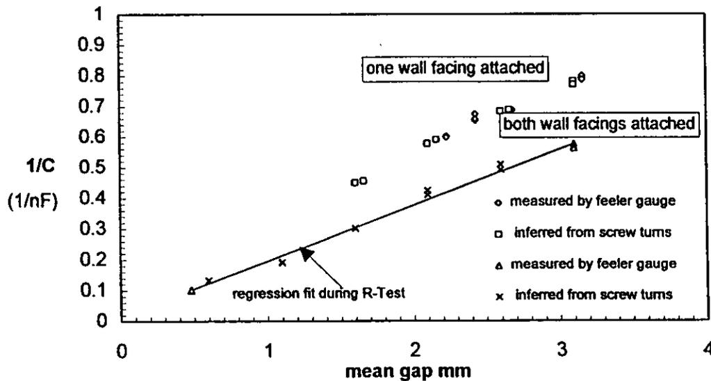
FIGURE 3. Electrical capacitance v mean gap (one face).
