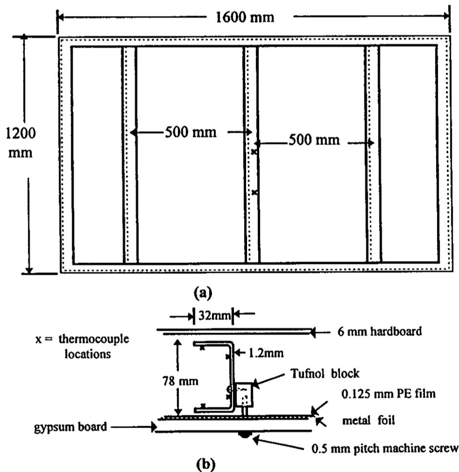
FIGURE 1. Layout of steel test frame.
