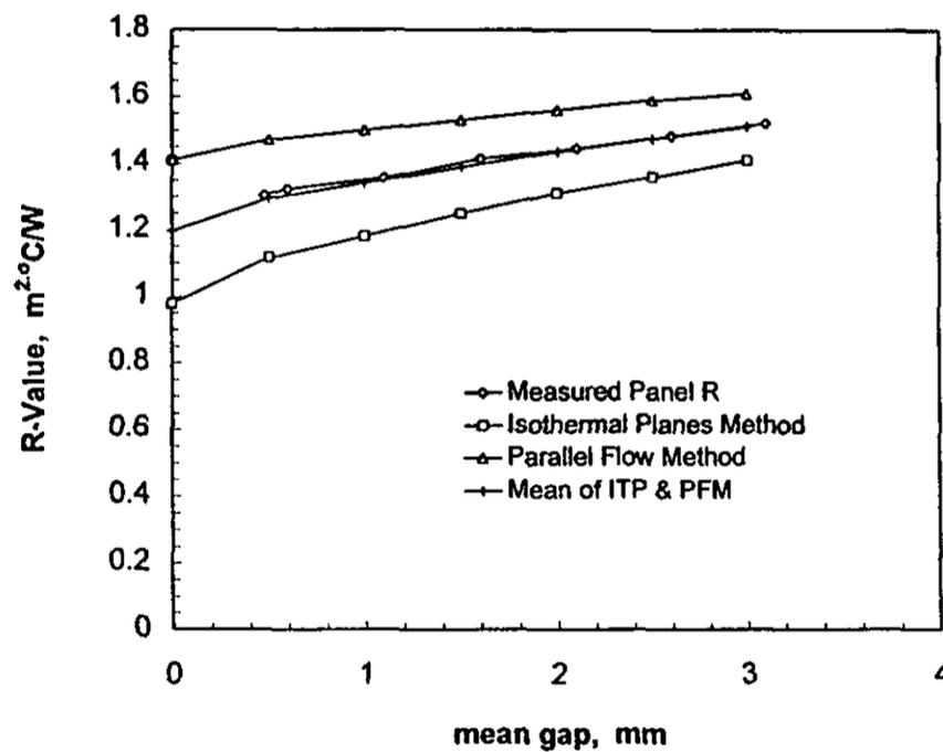
FIGURE 5. Comparison of calculated R-Values, fibreglass insulation (one face varied).
