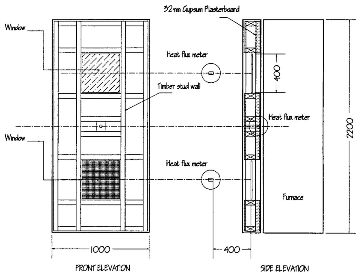
**Figure 3: Layout of fire-resistance test. The BRANZ pilot furnace was used to measure radiation from the furnace and radiation 400 mm in front of the glass windows. Note that only small panes of glass were needed for this test. Note also the locations of the heat flux meters.**
