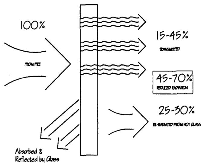
**Figure 1: Radiation model for fire-resistant glass exposed to a building fire.**
