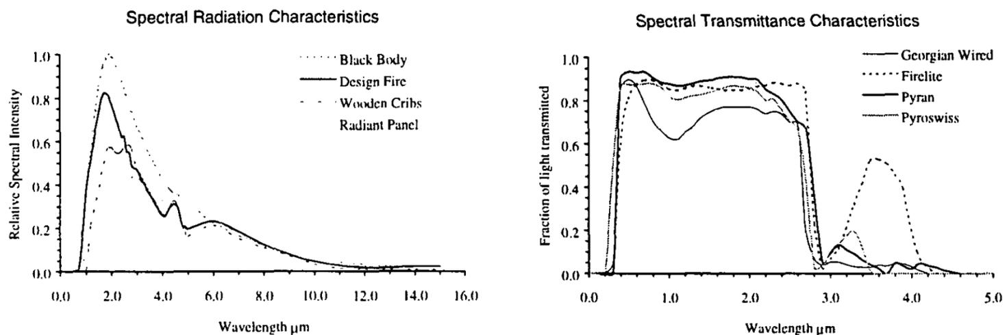
**Figure 2: The spectral radiation characteristic of the radiation sources studied and the spectral transmittance characteristics of each glass used.**
