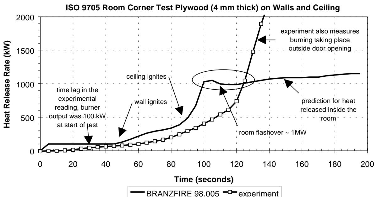
**Figure 10: Comparison with Experiment for Plywood**
