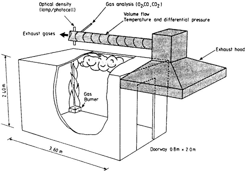
**Figure 3: ISO 9705 Room Fire Test**
