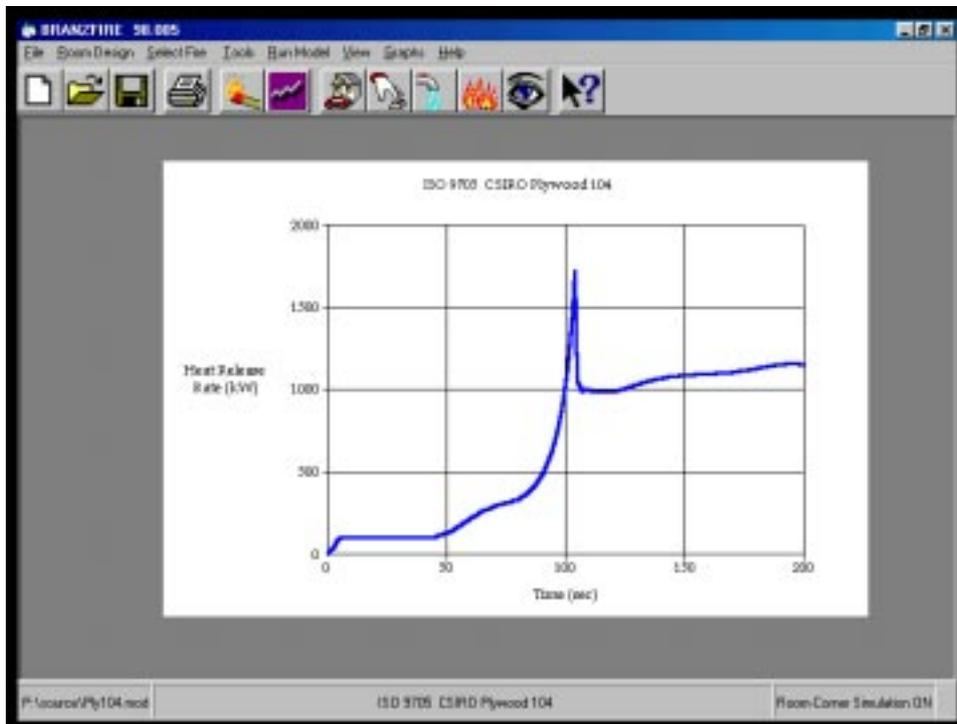
**Figure 7: Predicted Heat Release Rate Graph**
