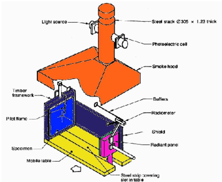
Figure 1: AS 1530 Part 3 Fire Test
