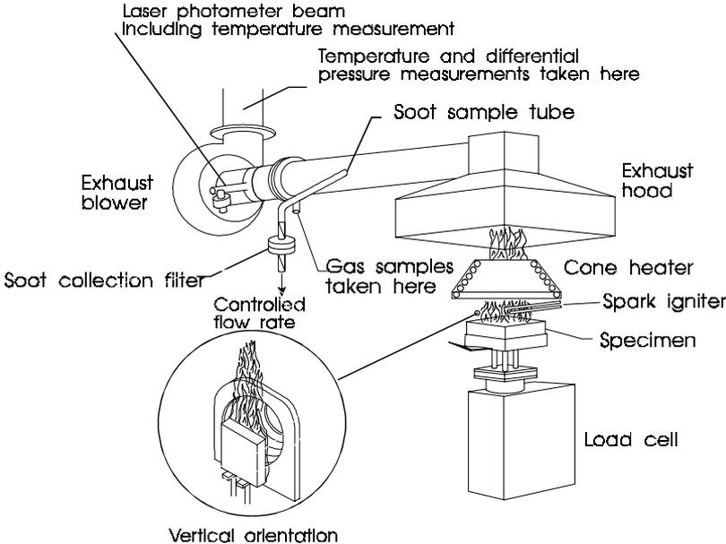
**Figure 2: Cone Calorimeter Apparatus**
