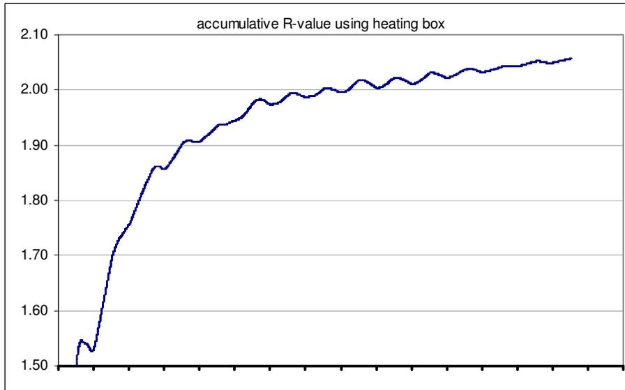
Figure 11: Fibrous polyester insulation – accumulative R-value using heating box (x-axis units = days, y-axis units = m<sup>2</sup>K/W)
