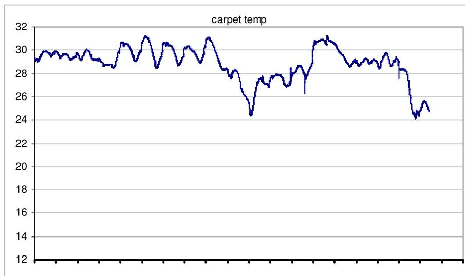
**Figure 21: Foil across bottom of joists – using heating box – carpet temperature (x-axis units = days, y-axis units =  $^{\circ}C$ )**
