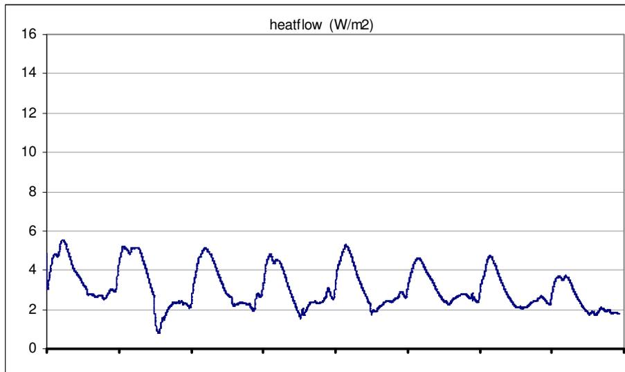
**Figure 19: Foil draped – using room heating – heat flow (x-axis units = days, y-axis units = W/m<sup>2</sup>)**
