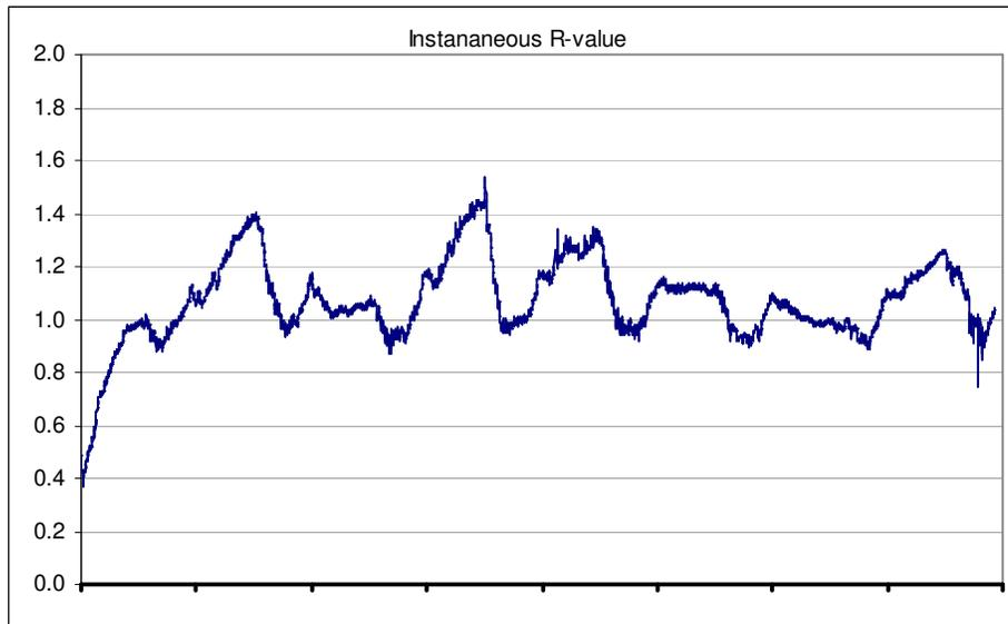
Figure 16: Foil draped – using heating box – instantaneous R-value (x-axis units = days, y-axis units = m<sup>2</sup>K/W)
