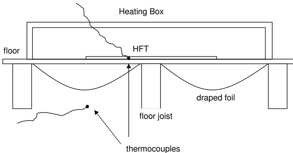
**Figure 1: Location of thermocouples**
