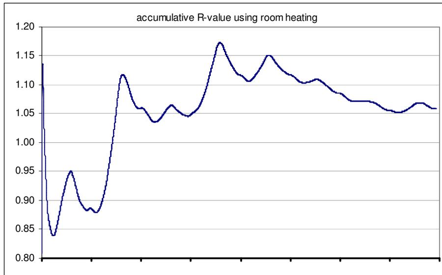
Figure 7: Foil draped – accumulative R-value using room heating (x-axis units = days, y-axis units =  $m^2K/W$ )
