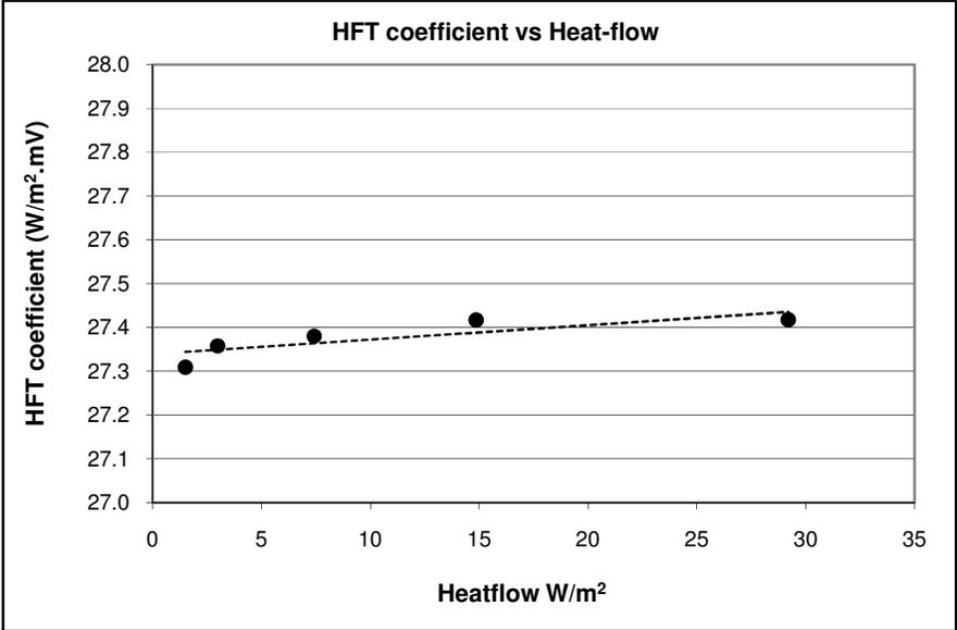
**Figure 3: Transducer output coefficient versus heat flow**
