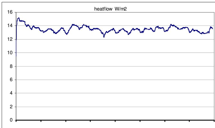
**Figure 15: Foil draped – using heating box – heat flow (x-axis units = days, y-axis units = W/m<sup>2</sup>)**
