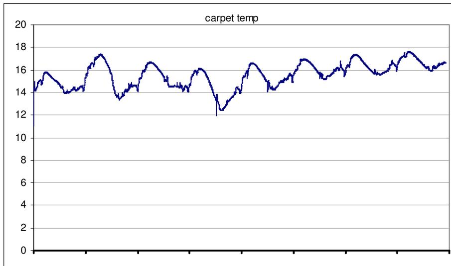
Figure 17: Foil draped – using room heating – carpet temperature (x-axis units = days, y-axis units = °C)
