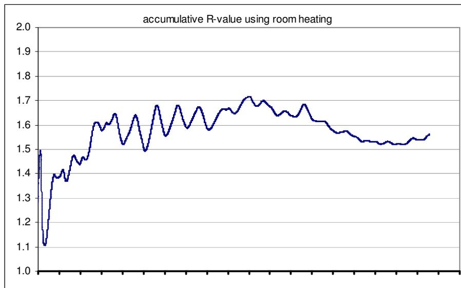
Figure 10: Foil across bottom of joists – accumulative R-value using room heating (x-axis units = days, y-axis units = m<sup>2</sup>K/W)
