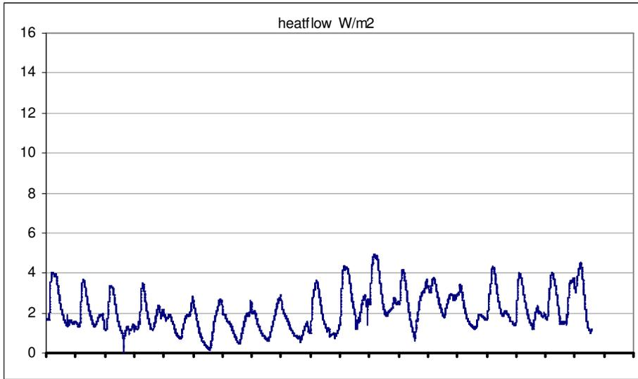
**Figure 28: Foil across bottom of joists – using room heating – heat flow (x-axis units = days, y-axis units =  $W/m^2$ )**
