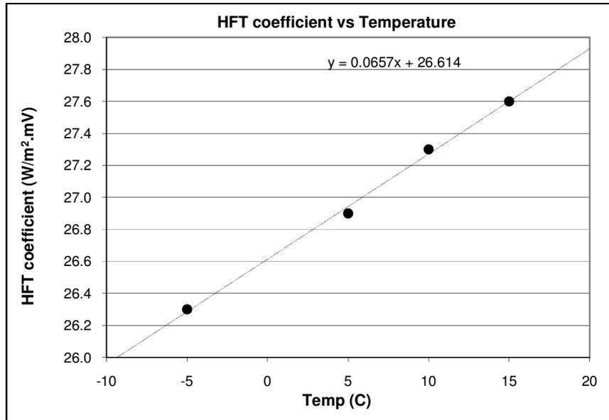
Figure 4: Transducer output coefficient versus temperature
