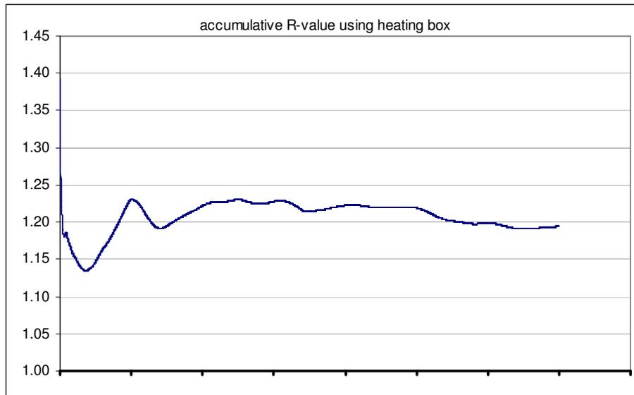
Figure 9: Foil across bottom of joists – accumulative R-value using heating box – after re-installation of measurement equipment (x-axis units = days, y-axis units = m<sup>2</sup>K/W)
