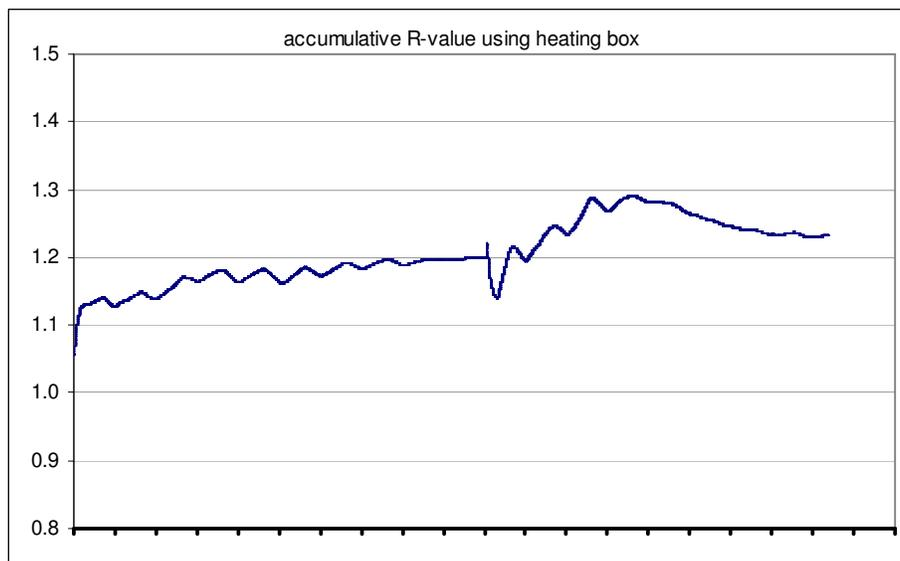
Figure 8: Foil across bottom of joists – accumulative R-value using heating box (x-axis units = days, y-axis units =  $m^2K/W$ )
