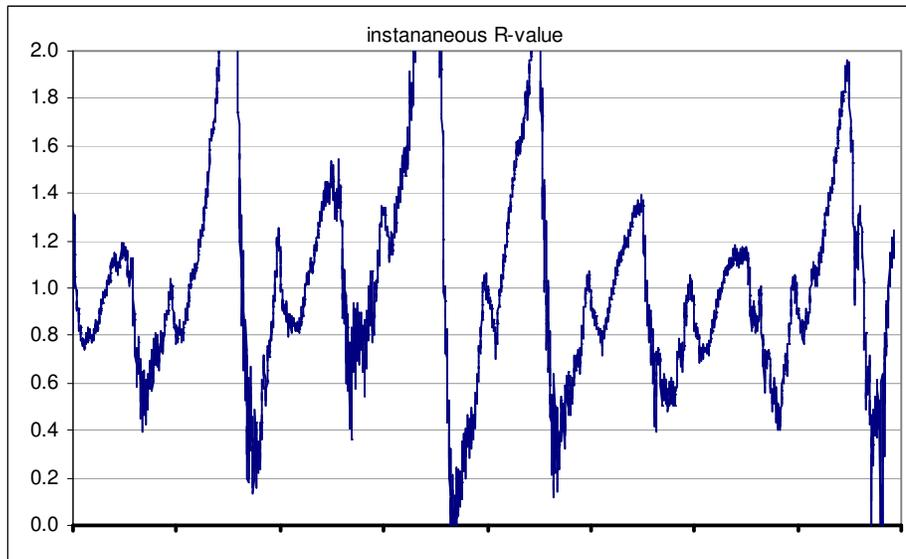
**Figure 20: Foil draped – using room heating – instantaneous R-value (x-axis units = days, y-axis units =  $m^2K/W$ )**
