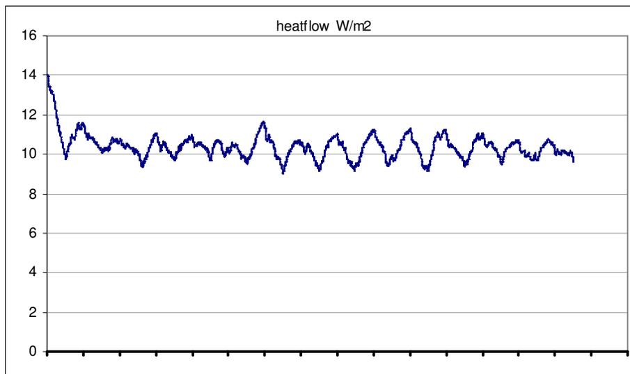
**Figure 33: Fibrous polyester insulation – using heating box – heat flow (x-axis units = days, y-axis units = W/m<sup>2</sup>)**
