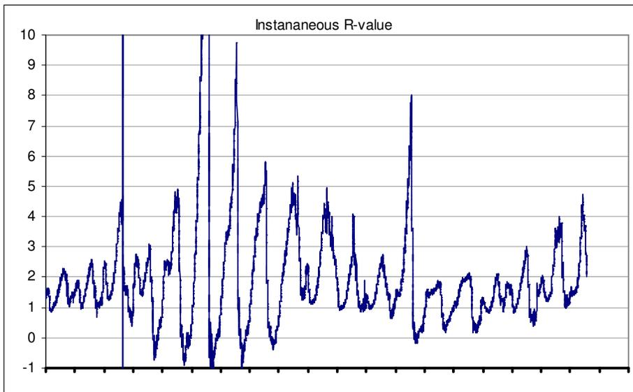
**Figure 29: Foil across bottom of joists – using room heating – instantaneous R-value (x-axis units = days, y-axis units =  $m^2K/W$ )**
