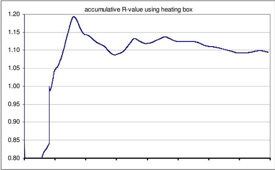
Figure 6: Foil draped – accumulative R-value using heating box (x-axis units = days, y-axis units = m²K/W)
