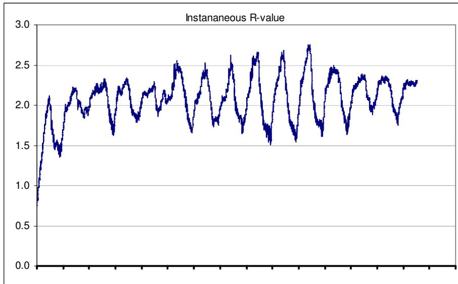
**Figure 34: Fibrous polyester insulation – using heating box – instantaneous R-value (x-axis units = days, y-axis units =  $\text{m}^2\text{K/W}$ )**
