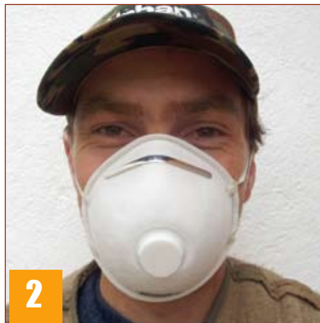
2 Valved P2 toxic dust mask – suitable for hardwood and softwood dust as well as welding and brazing fumes. Will not protect against gases, other vapours or paint spray.
