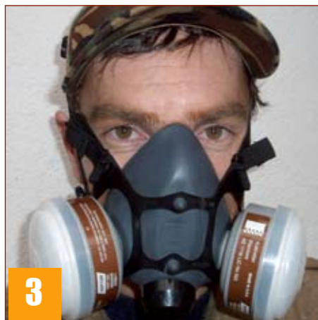
3 Half-mask respirator – with changeable filters and pre-filters for protection against paint mists and vapours. Use the appropriate filter for the job. Half-masks are not suitable for use in highly toxic areas or if the paints contain iso-cyanates. In these cases use a full mask with air supply.
