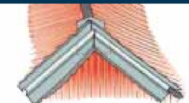
Lay hip ridges, lapping or cutting on an angle (mitre) to butt together. Trim underflashing to fit under hip ridges and fix ridge flashings to hip, dressing down soft edges.
