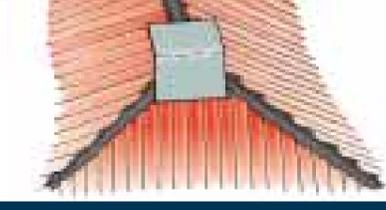
Lay a zinc, aluminium or butyl rubber underflashing (about 600mm x 300mm) over the ridge junction and fold centrally over the join.
