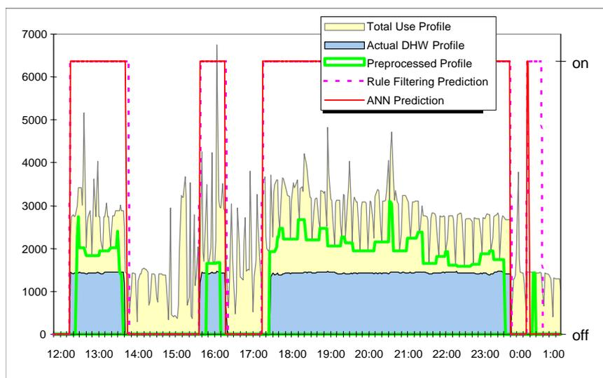
Figure 5. End-use disaggregation using a rule based algorithm and ANN.
