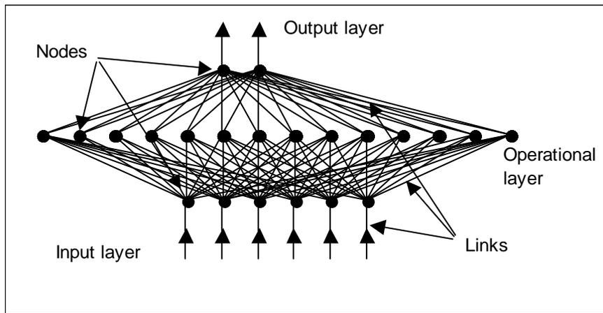
Figure 1. A diagram showing an example of an artificial neural network and the interactions between its three layers.
