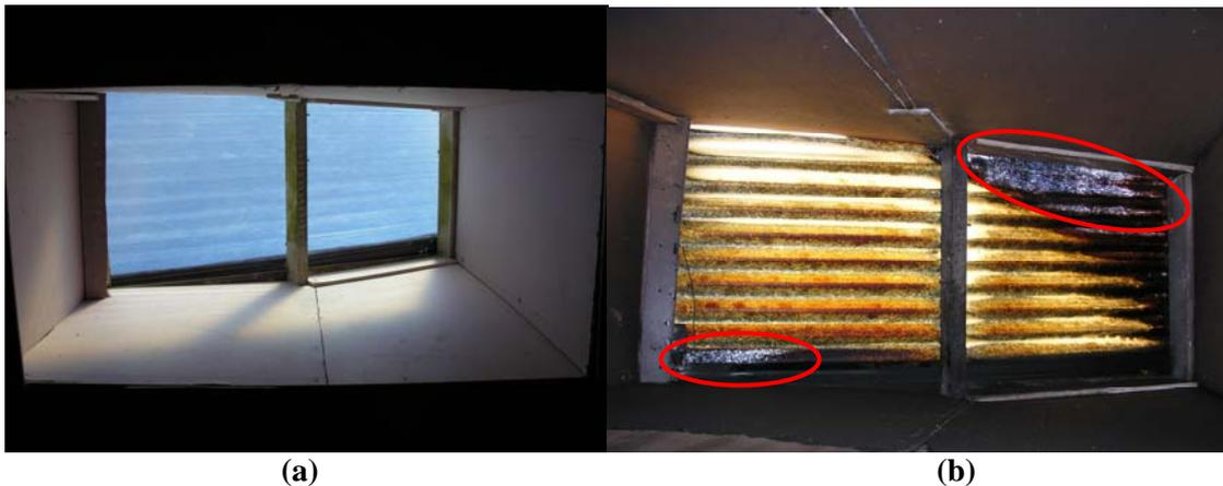
**Figure 3:** Photographs of the GRP vent from below (a) before and (b) after exposure to hot fire gases in a room. Areas of sheeting where the fibre mesh was exposed are indicated in red in (b).
