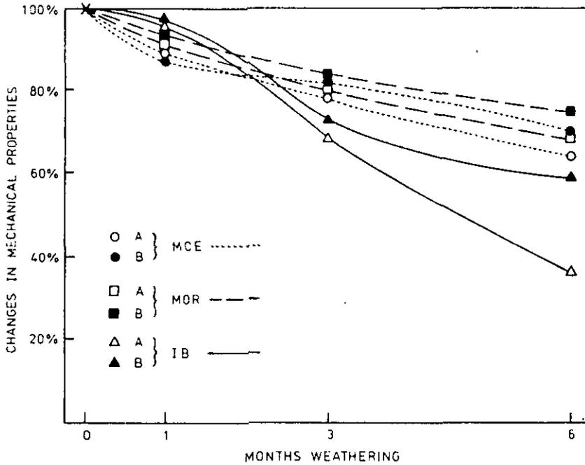
FIG. 1—Changes in properties with weathering (MOE and MOR are actual values measured after two sandings).
