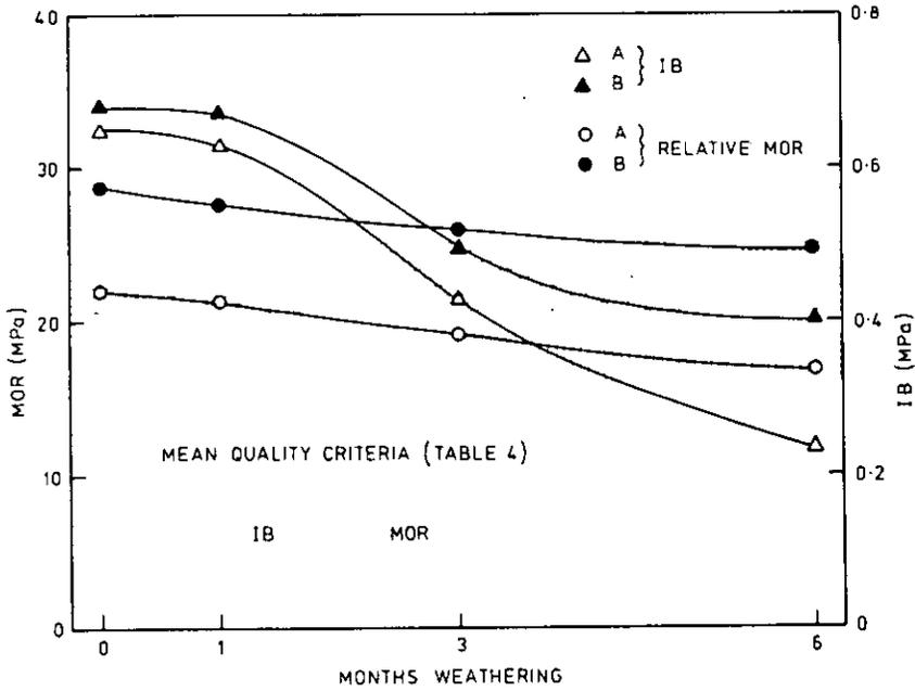
FIG. 4—The effect of weathering on relative MOR and IB.
