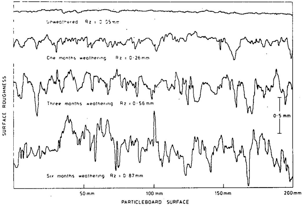
FIG. 3—Changes in surface roughness with weathering.
