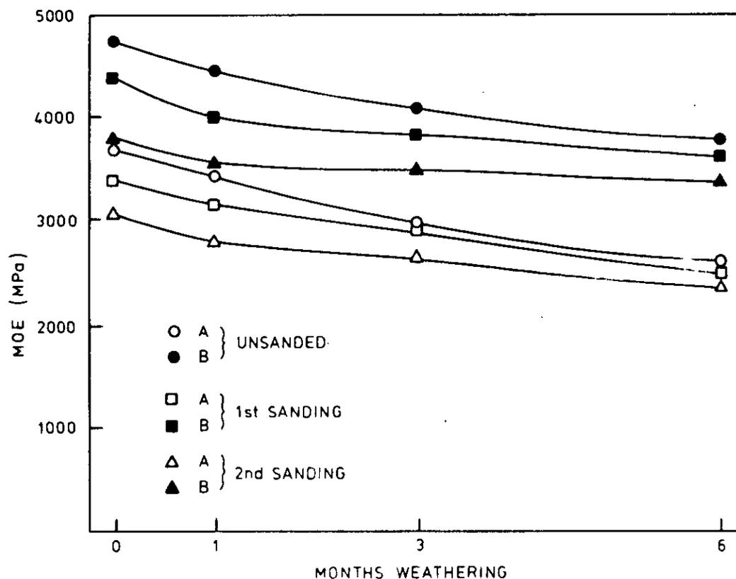
FIG. 2—The effect of sanding and weathering on relative MOE.
