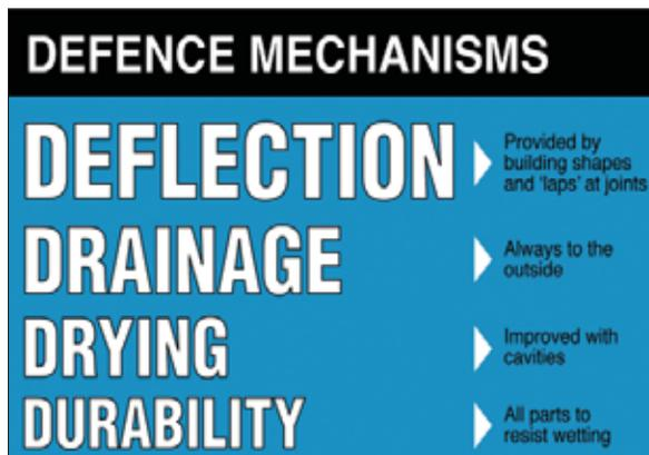
But the risk of penetrating the outer cladding defence is greater on exposed sites. So you need to improve the second defence – drainage – by using a cavity. The cavity, in turn, improves the third defence: drying (see Figure 2).
