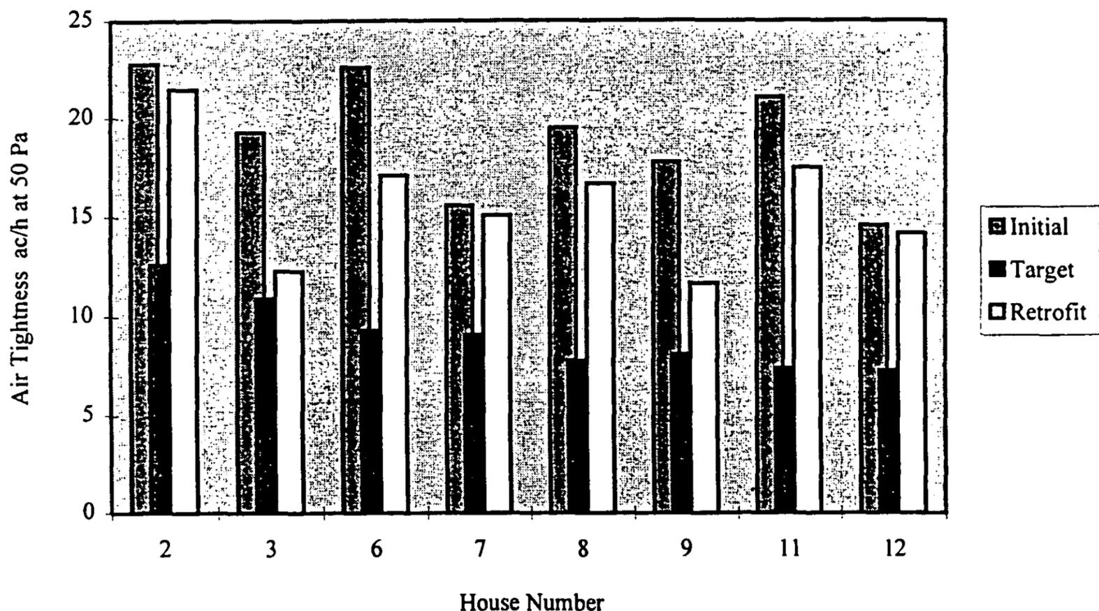
Figure 6: Airtightness of houses before and after retrofit compared with airtightness levels achieved with temporary upgrades
