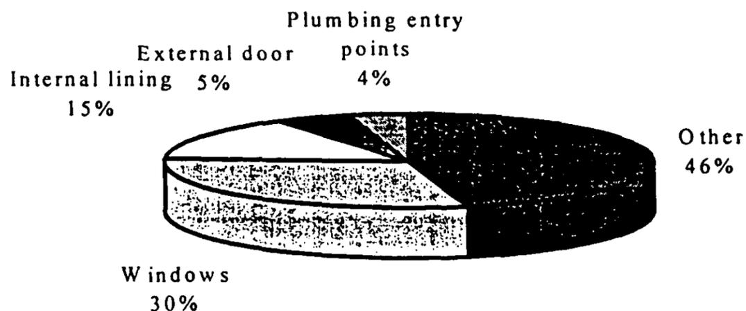
Figure 4: Average temporary airtightness improvements achieved in 15 houses. The residual air leakage is shown as "other"
