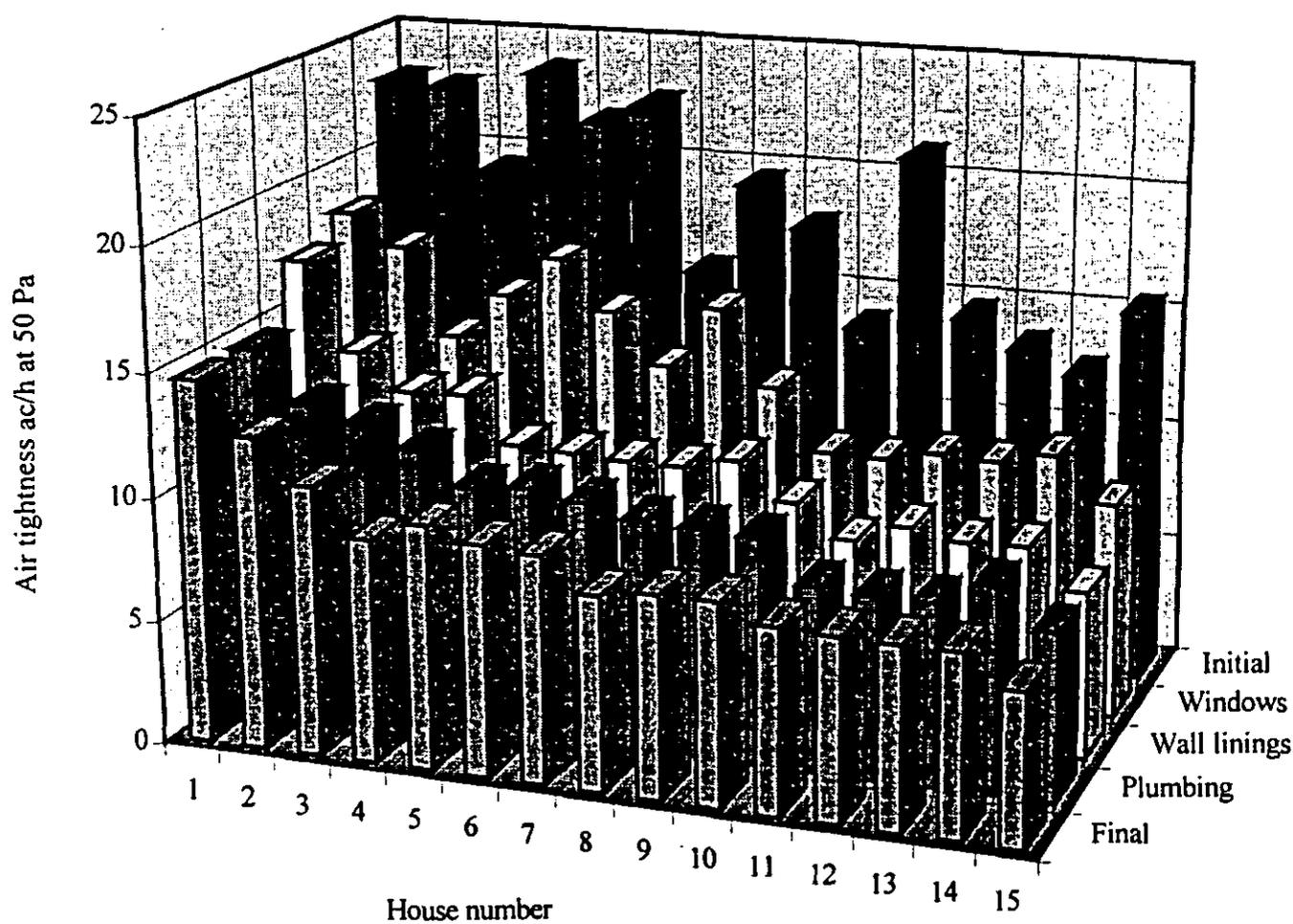
Figure 5: Four stages of temporary airtightening 15 pre 1950's houses
