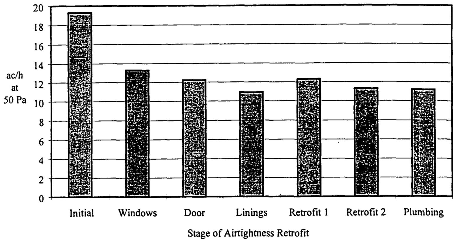
Figure 3: The airtightness of house 3 showing the temporary improvements and retrofit stages
