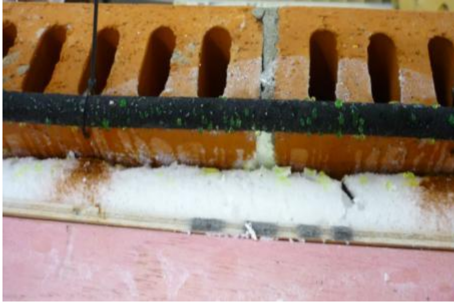
Figure 1: Water applied through a porous tube (D4864)
