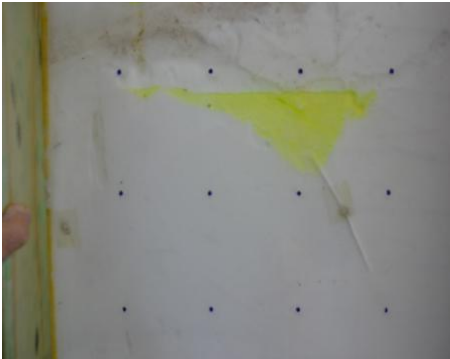
Figure 3: Leakage observed 6 minutes after start of test (D4864)
