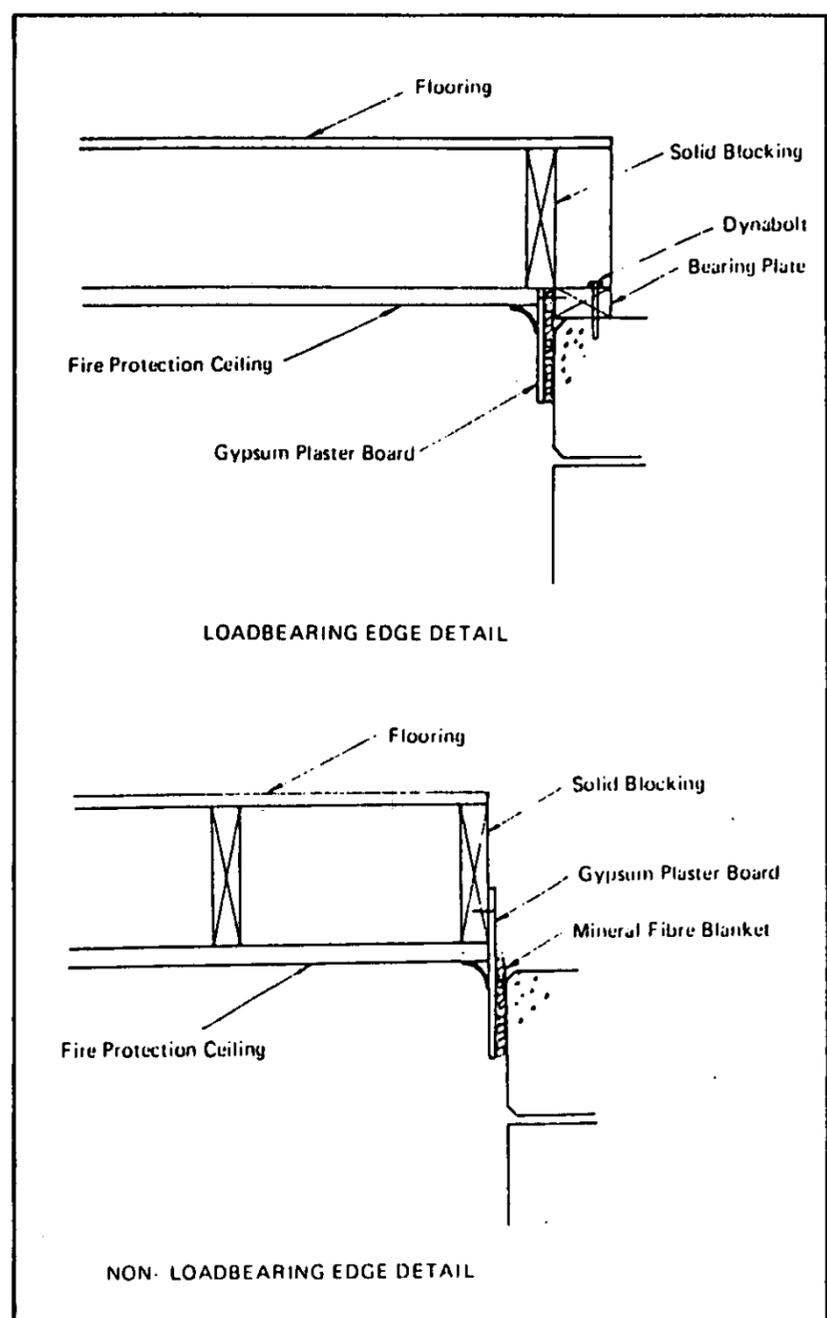
Figure 1: Specimen Edge Details.
