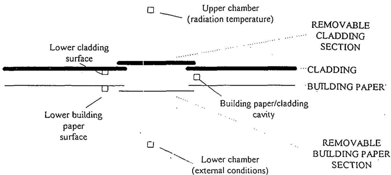
Figure 2: Location of sensor pairs (temperature and relative humidity) in roof samples
