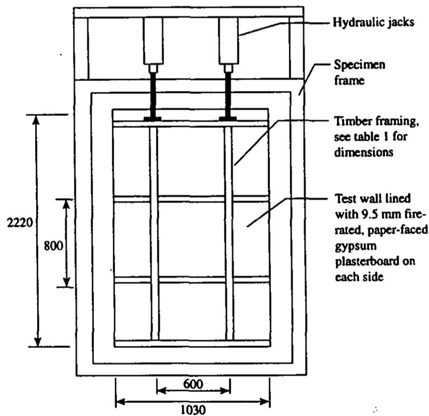
**Figure 2. Typical small-scale test specimen used in the testing program.**
