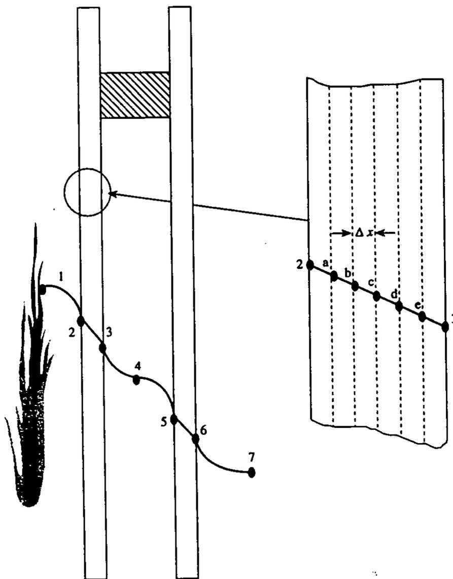
**Figure 3. Cavity wall section showing heat transfer nodes.**
