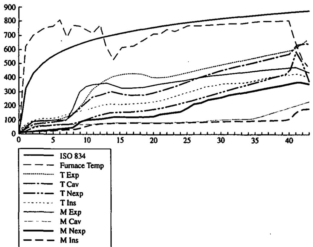
Figure 5. Test FP1583A comparison with model.
