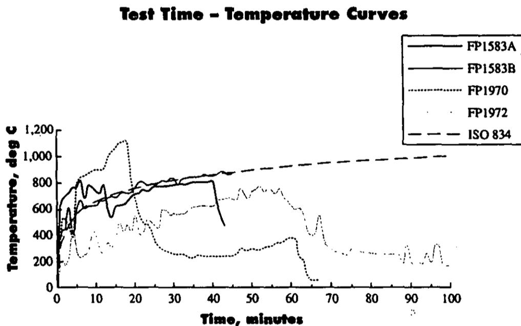
Figure 1. Comparison of test time-temperature curves.
