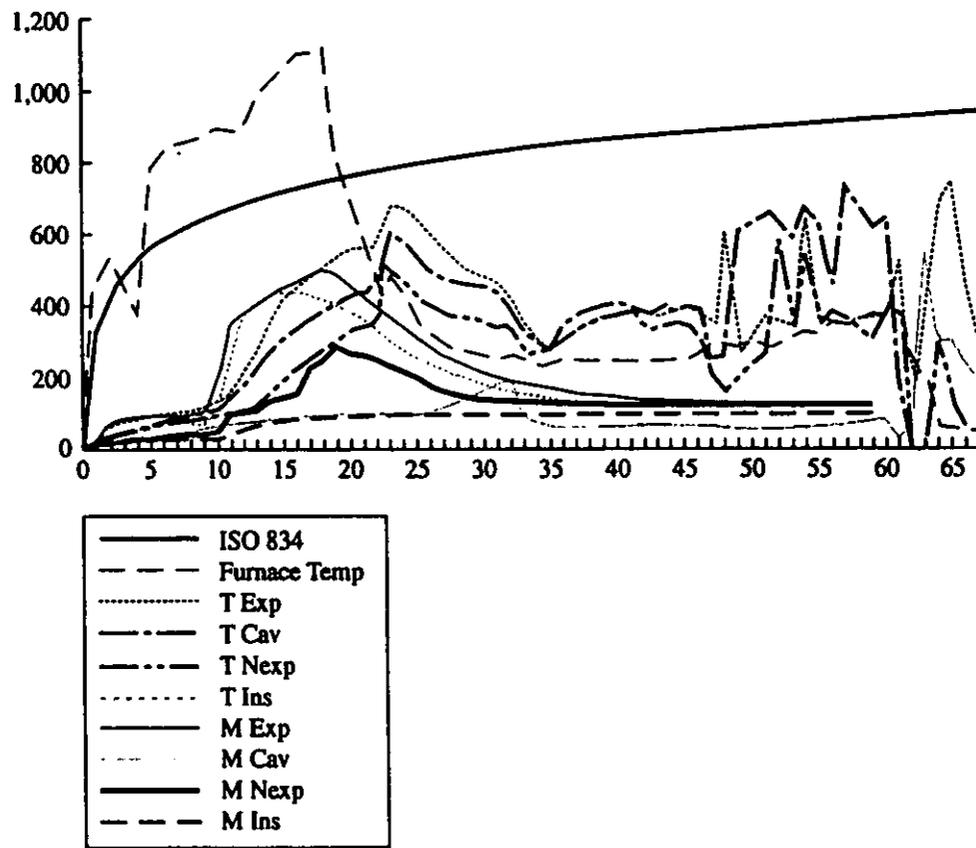
Figure 7. Test FP1970 comparison with model.
