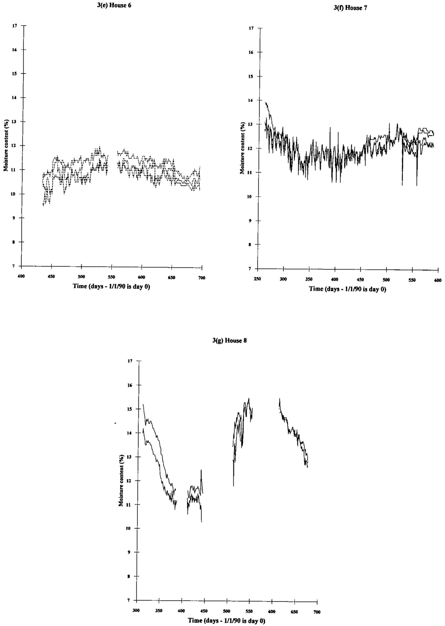
Fig. 3. Twenty-four hour mean of mid-timber moisture contents.
