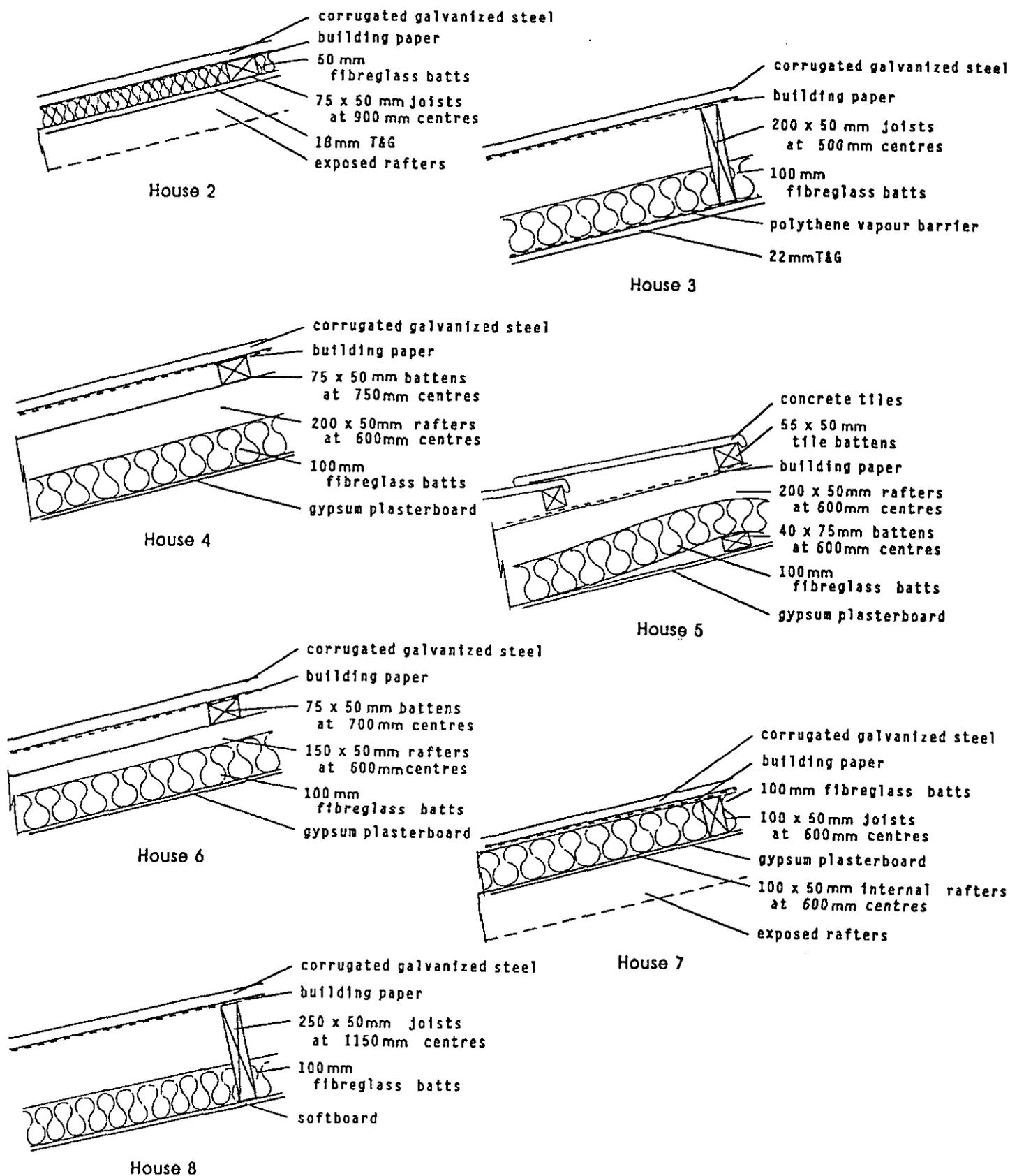
Fig. 2. Roofing details of the houses studied.
