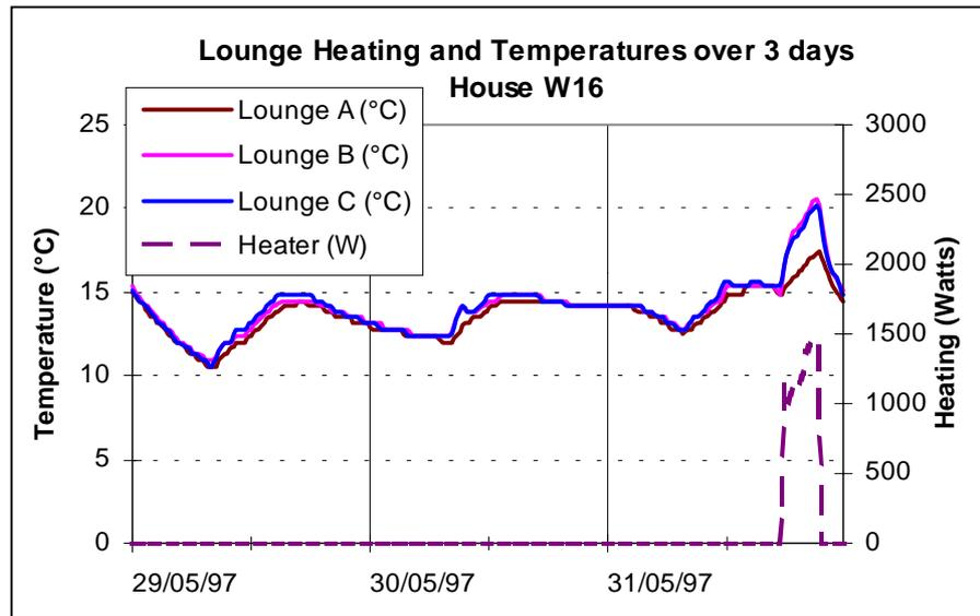
Figure 1 Three day temperature and heating profile for house 16.
