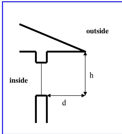
**Figure 4: Sizing eaves to protect summertime overheating**
