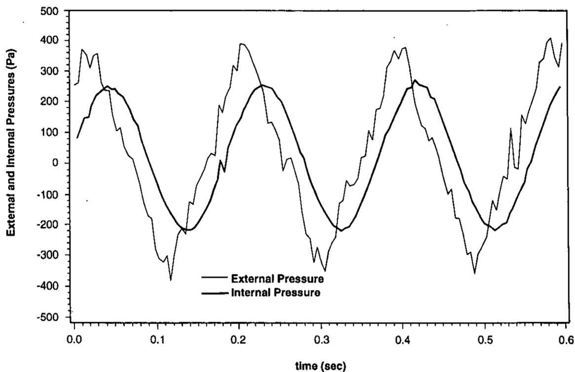
Fig. 3. Air pressures logged for a single experimental run, where the sinusoidal fluctuations in the external air pressure drive the sinusoidal air pressure fluctuations in the cavity.
