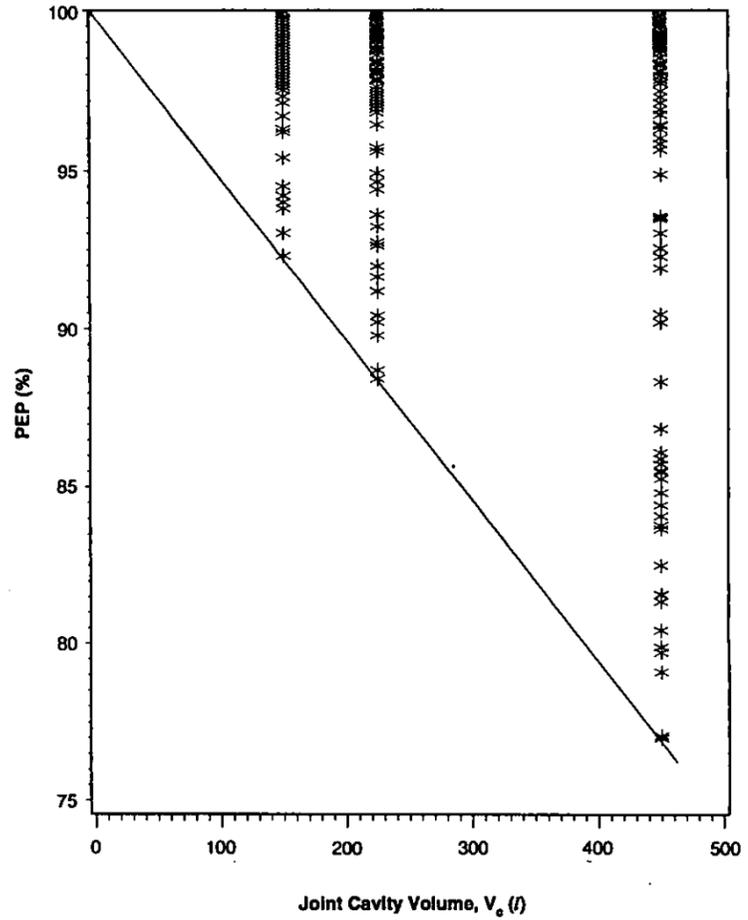
Fig. 6. Effect of variation in the joint cavity volume. One member of a family of curves for all the tested frequency values and joint opening area values is shown. Volume varies from 150 l to 450 l.
