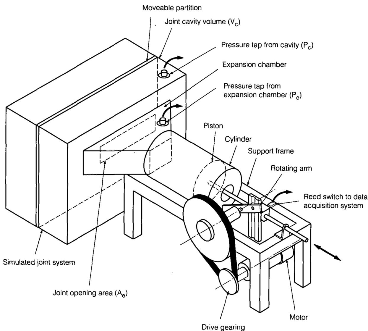
Fig. 2. Sinusoidal air pressure generation equipment and joint simulation.
