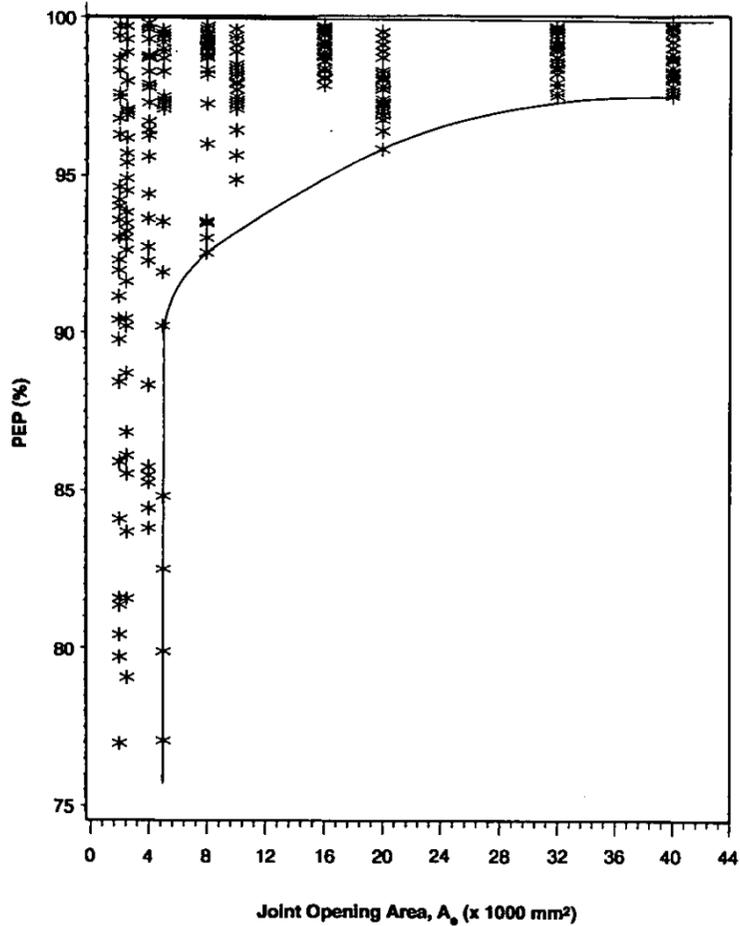
Fig. 5. Effect of variation in the external joint opening area. Two of a family of curves for all values of frequency and joint cavity volume are shown. Joint opening area varies from 2000 mm<sup>2</sup> to 40,000 mm<sup>2</sup>.
