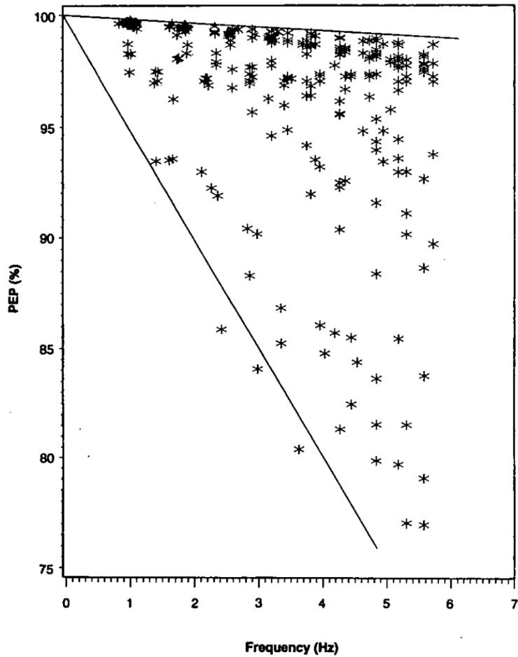
Fig. 4. Variation in the air pressure equalization percentage with frequency of the external air pressure fluctuation. Two of a family of curves for all values of the joint opening area and cavity volume are shown. Frequency varies from 0.96 to 5.6 Hz.
