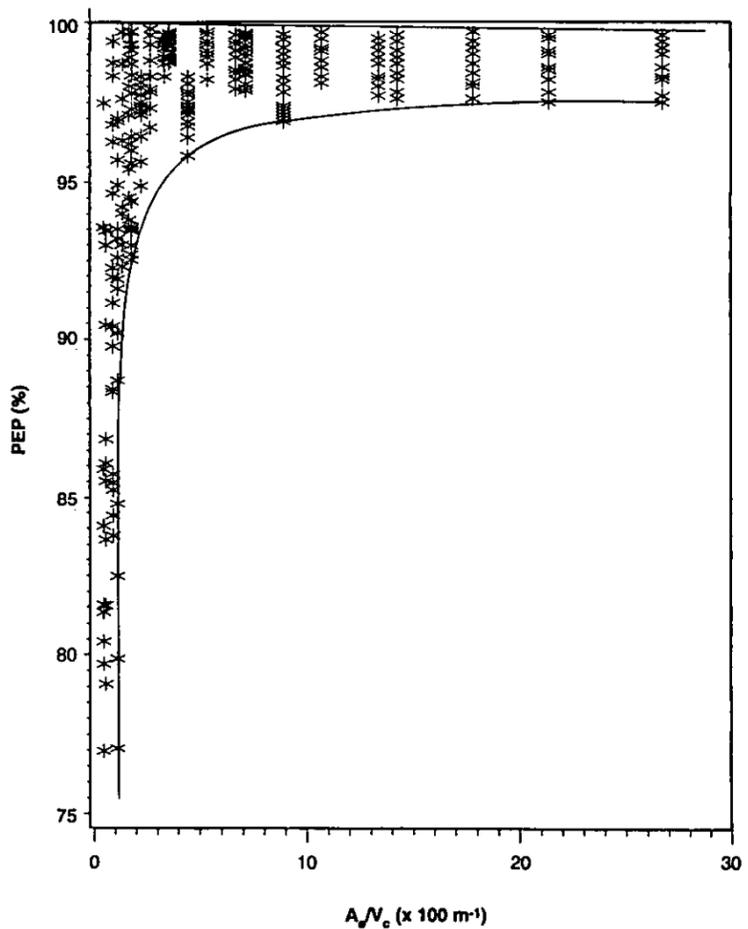
Fig. 7. Pressure equalization percentage versus joint opening area/cavity volume. Two of a family of curves for all values of frequency are shown. The ratio varies from 0.005 m<sup>-1</sup> to 0.26 m<sup>-1</sup>.
