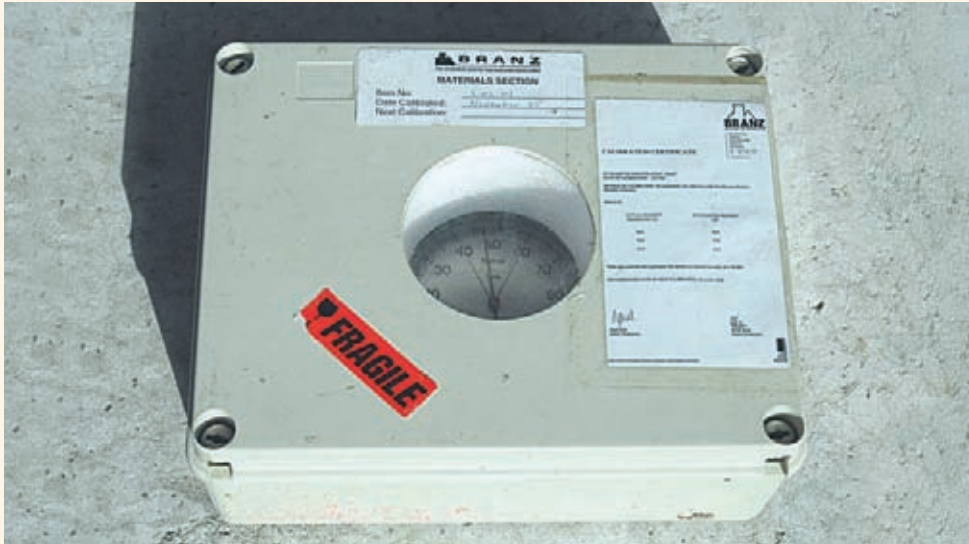
The Edney hygrometer measures relative humidity in slabs.
