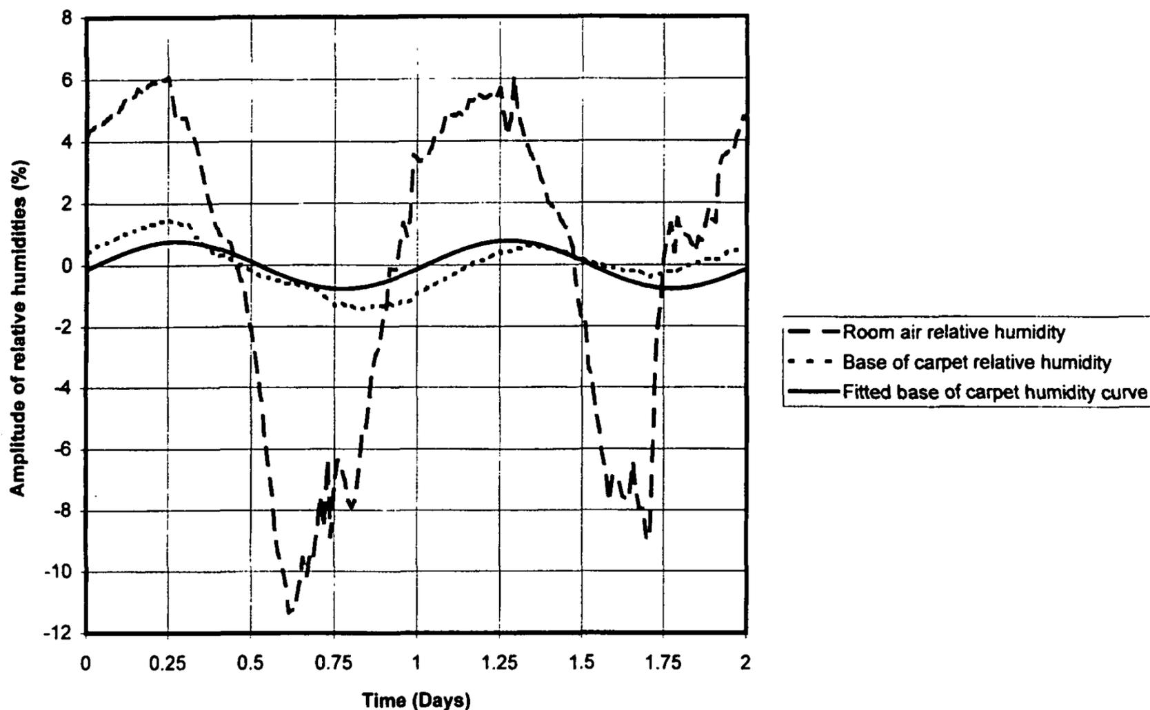
Fig. 6. Comparison between experimental and modelled relative humidities in the base of a carpet.
