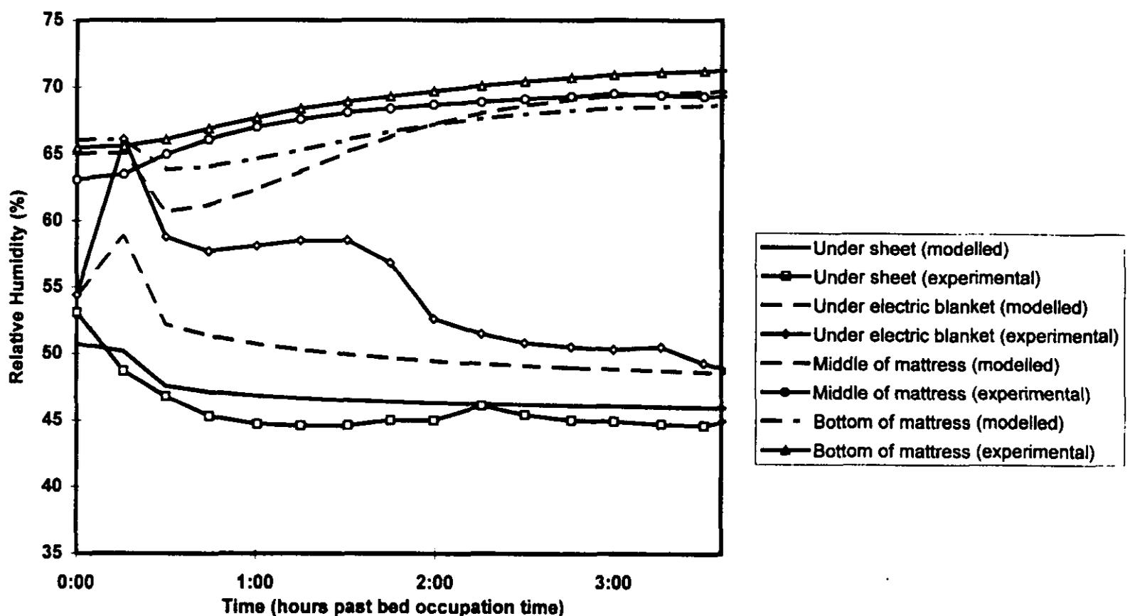
Fig. 5. Comparison between experimental and modelled relative humidities, temperatures and vapour pressures in a mattress when the bed is occupied.
