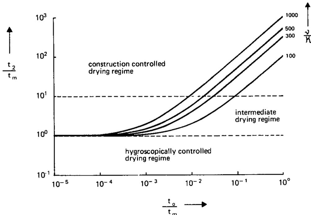
Fig. 4. Normalised plot of the drying time constant,  $t_2$ , against the cavity tightness time constant,  $t_o$ .
