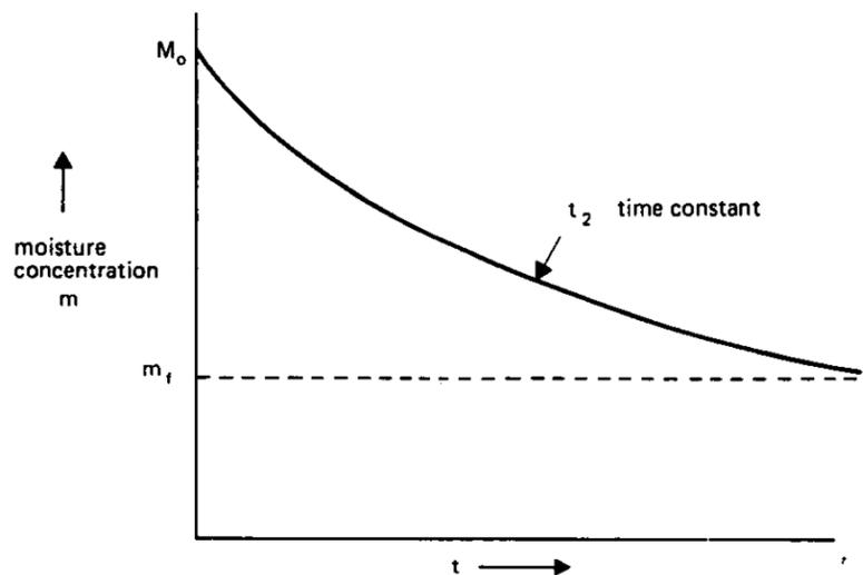
Fig. 2. General shape of hygroscopic material drying curve.
