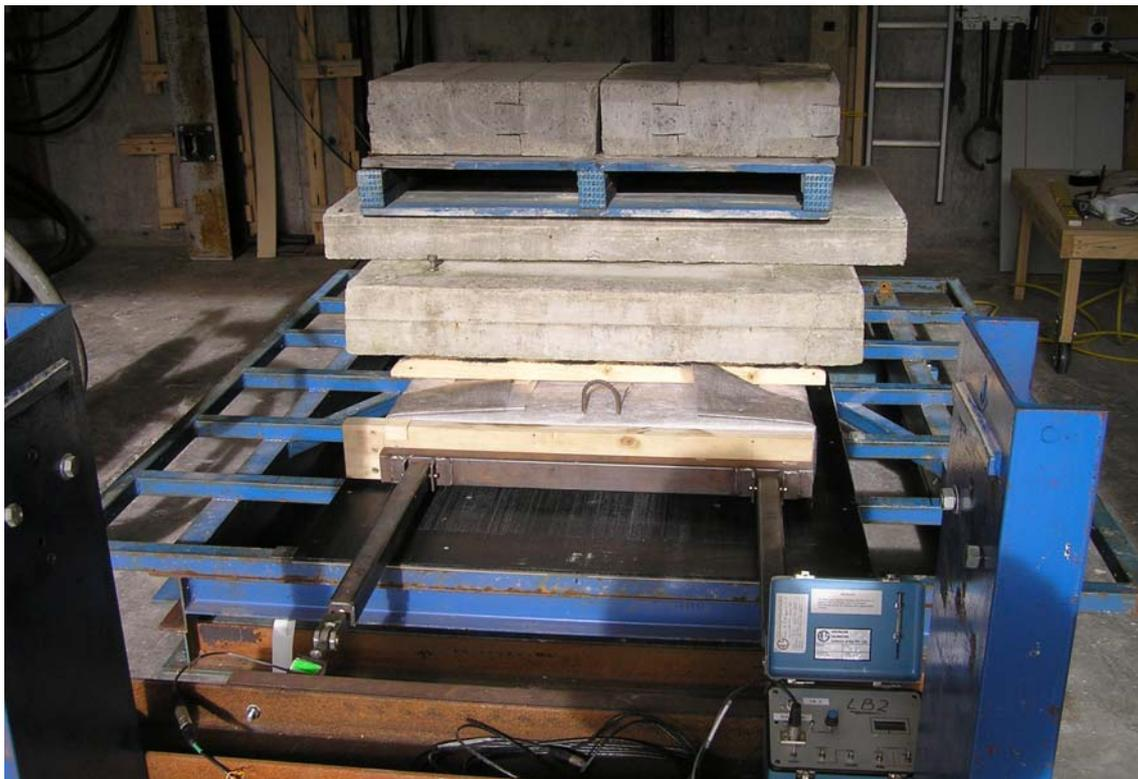
**Figure 16. Mass added to the shake table**
