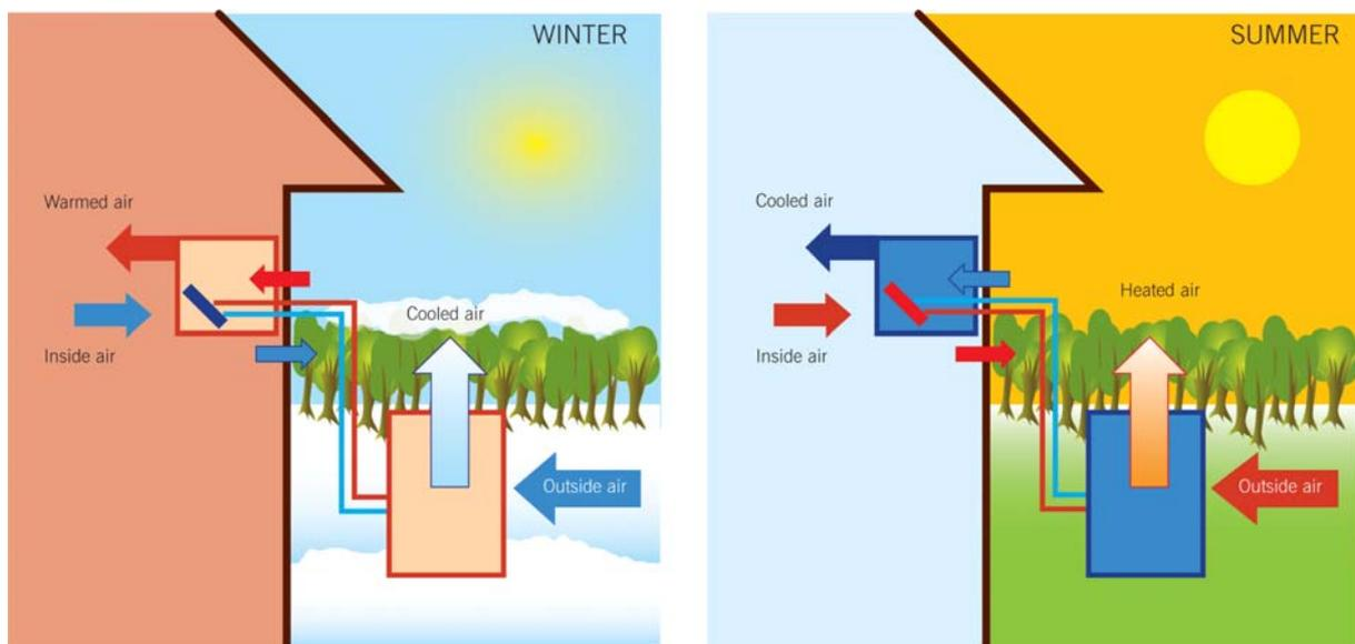
Figure 1: How air source heat pumps work
