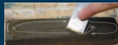
Oil the coarse side of the oilstone and tilt the chisel to 30°. This action will lift the back of it just off the stone slightly. Now move the chisel in a long ellipse stroke, a figure of eight or an "X" pattern, maintaining the same 30° angle throughout the motion while keeping the blade at an angle to the direction the chisel is being moved.
