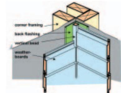
Figure 3. Internal corner weatherboard back flashing
