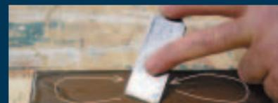
Similarly, oil the fine side of the oilstone and repeat the sharpening procedure you used on the coarse side, this time applying only light pressure so the chisel just skims across the surface.
