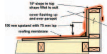
Figure 4. Membrane parapet flashing
