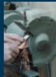
Grind the front of a very blunt chisel to about 25°. Using a grinding wheel creates a slightly concave effect, which is okay. Don't grind for more than a few seconds at a time,
