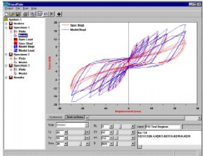
**Figure 4.** Fitting the bar-spring model to a test record using the BraceRate software.
