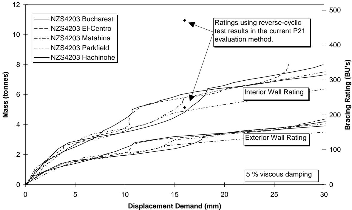
**Figure 9.** Mass-Displacement ratings for NZS 3604 Zone A.
