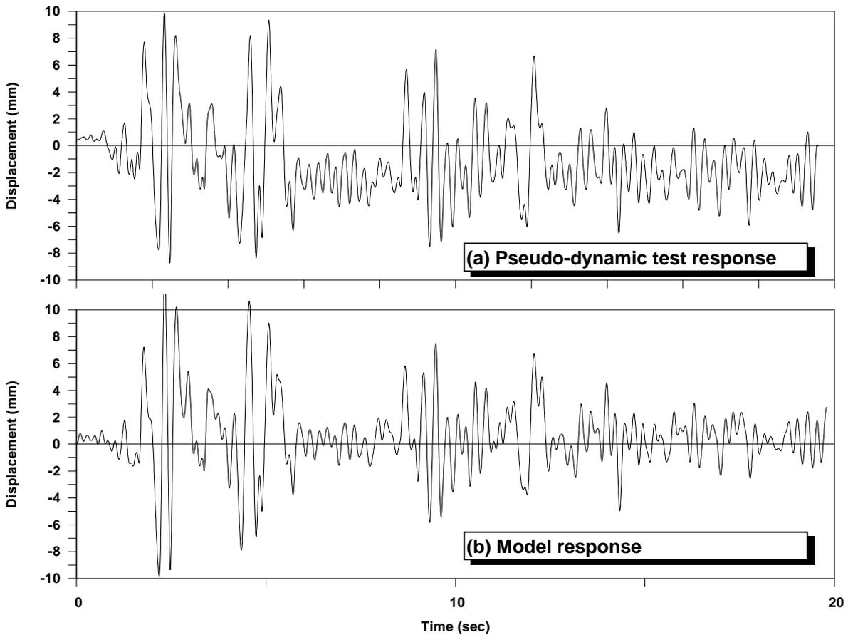
Figure 7. Interior wall responses with a mass of 5000 kg and subjected to  $1.25 \times$  El-Centro 1940 earthquake record (3.8 % damping).
