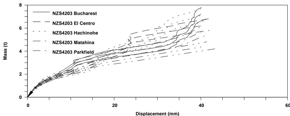
**Figure 5.** 'Displacement spectra' generated by the BraceRate software for the Figure 4 specimen.
