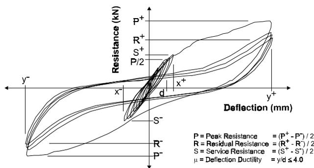
**Figure 1.** Test specimen response to the 'P21' test procedure [3].
