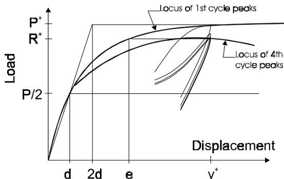
**Figure 10.** Definitions of yield for use with the current ‘P21’ rating procedure
