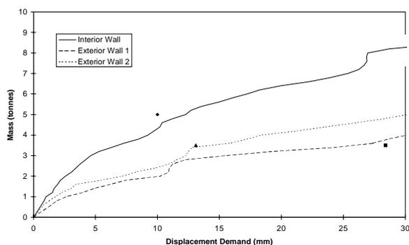
**Figure 8.** Mass-displacement demand plots for the three walls
