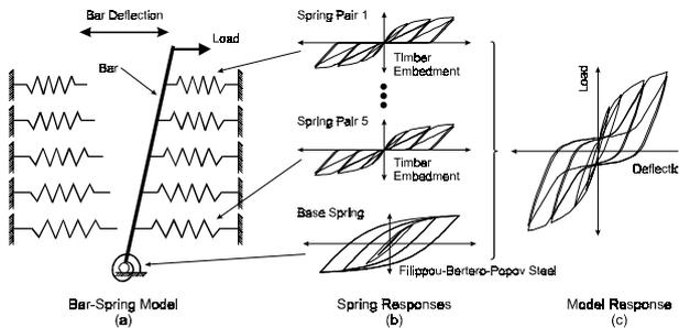
**Figure 3.** Revised bar-spring model.
