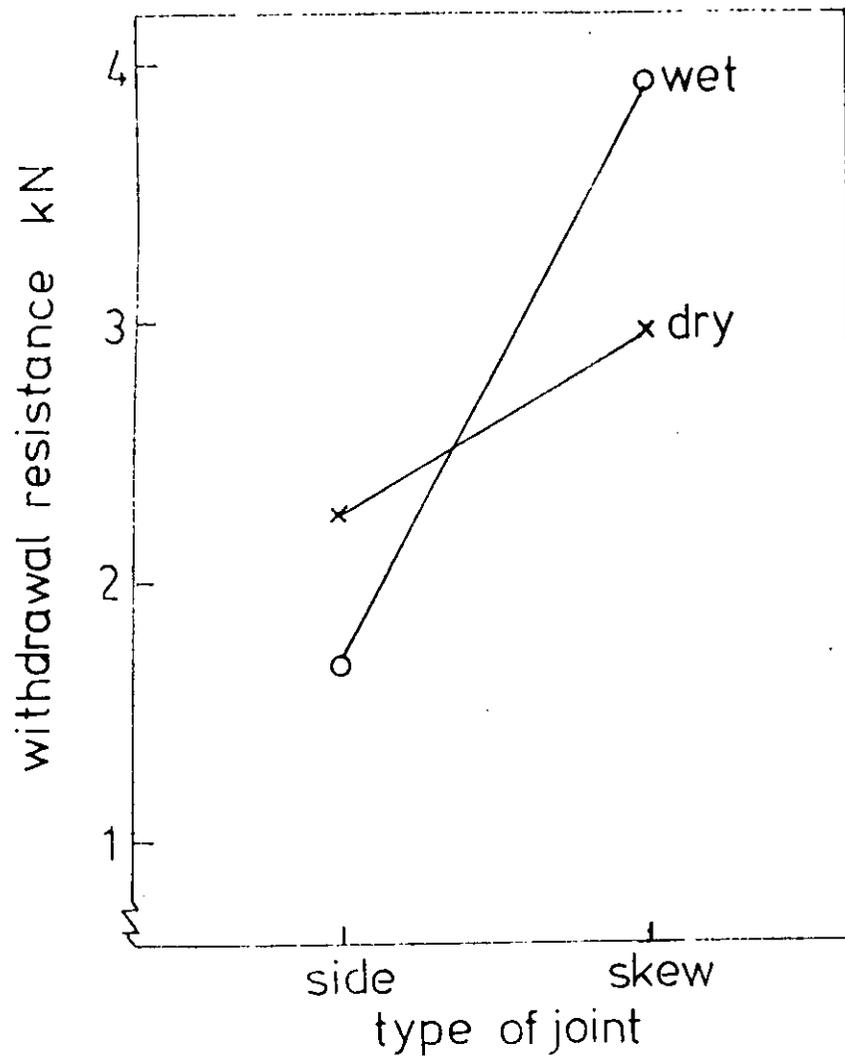
Fig. 9.- Variation in strength of joint with method of nailing.
