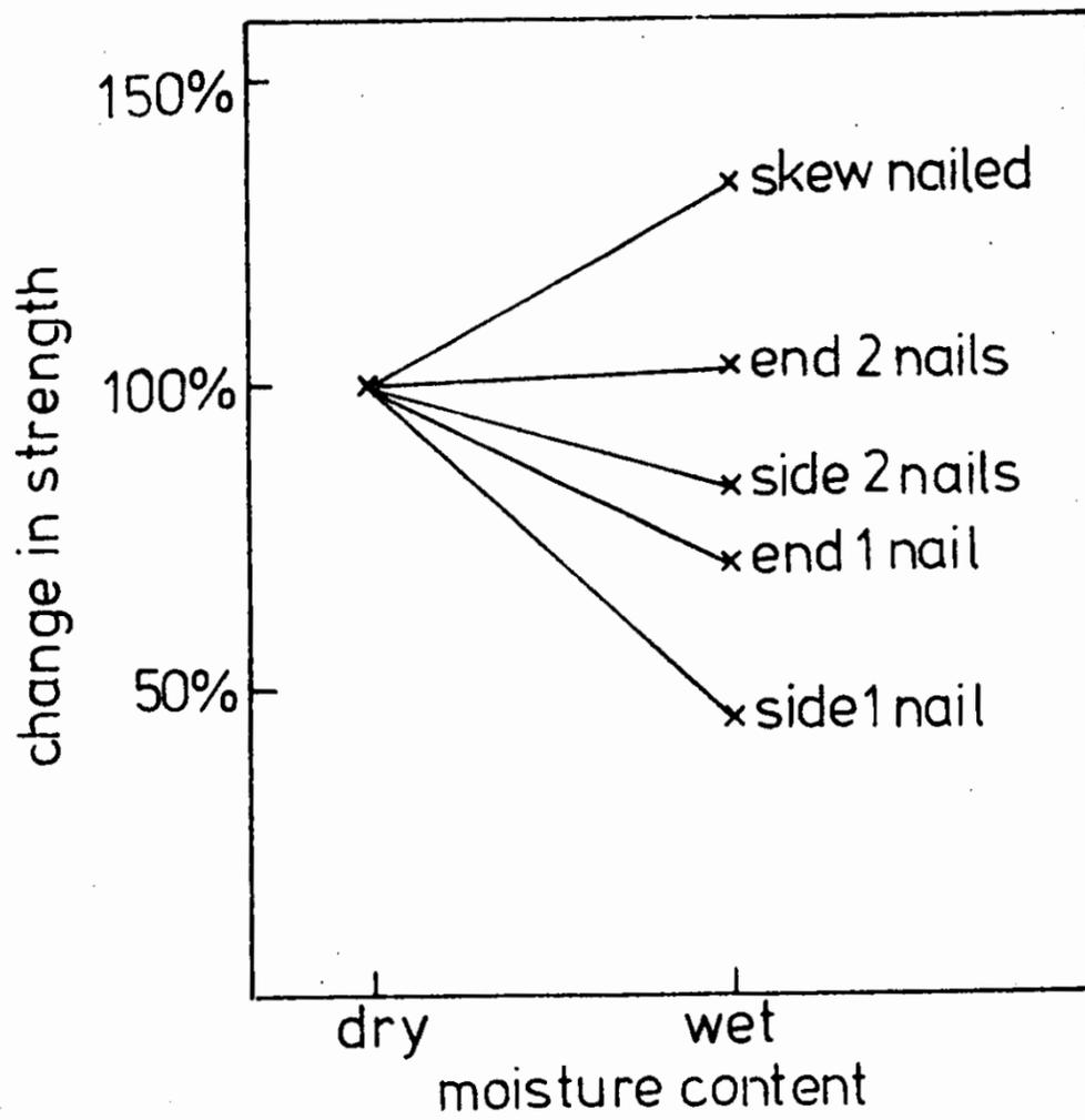
Fig. 7.- Variation in strength of joint with moisture content of wood during nailing.
