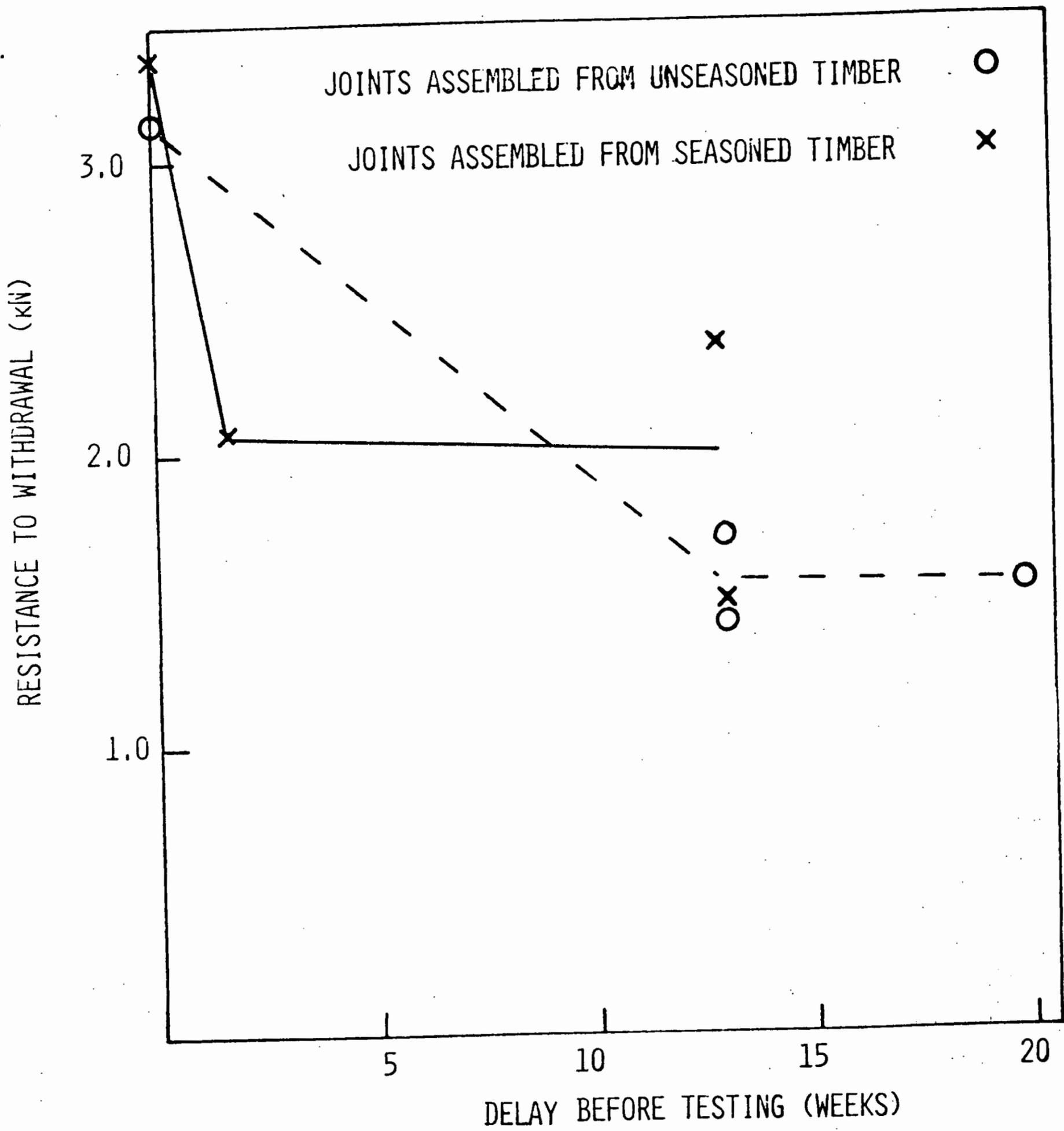
Fig. 4.- Effects of delay in testing on nail-withdrawal resistance.
