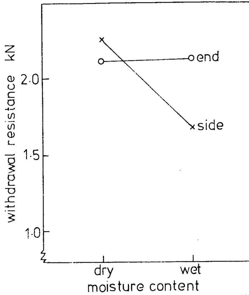
Fig. 8.- Variation in strength of joint with direction of grain of wood.
