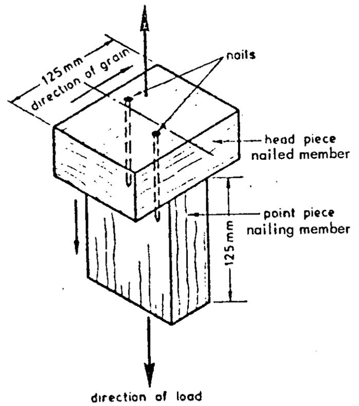
Fig. 2.- Straight-nailed into end grain:
