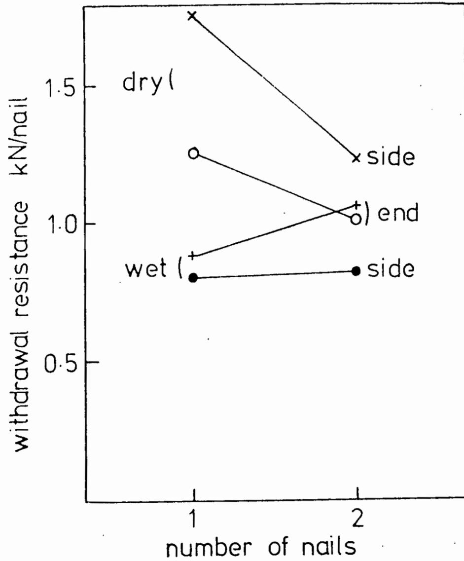
Fig. 6.- Variation in strength of joint with number of nails in joint.
