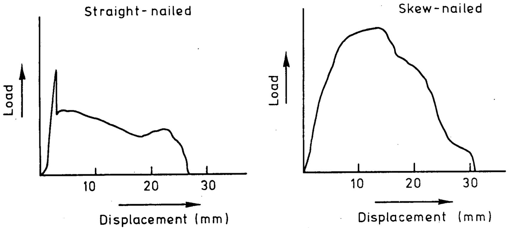
Fig. 5.- Typical load-deformation curves for straight-nailed and toe-nailed joints. The diagrams are tensometer traces and include deformations resulting from joint adjustments and wood compression.
