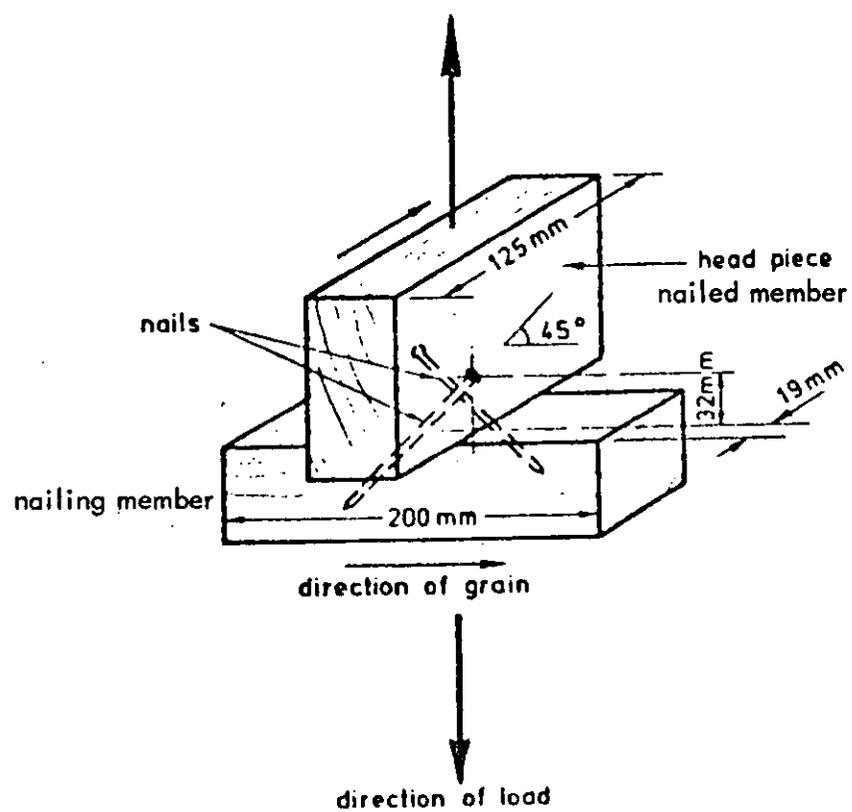
Fig. 3.- Toe-nailed into side grain:
