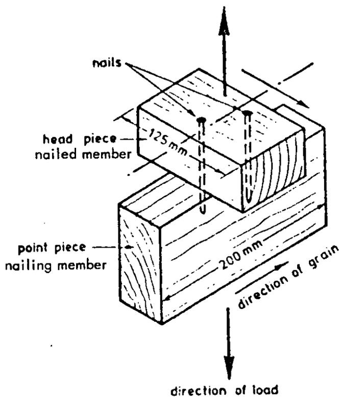
Fig. 1.- Straight-nailed into side grain:
