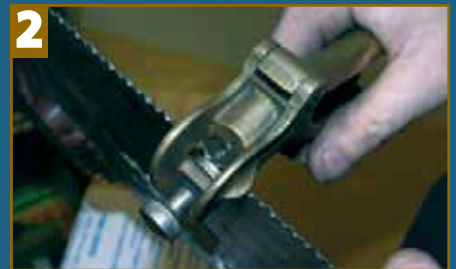
A setting tool has an anvil and a punch.
