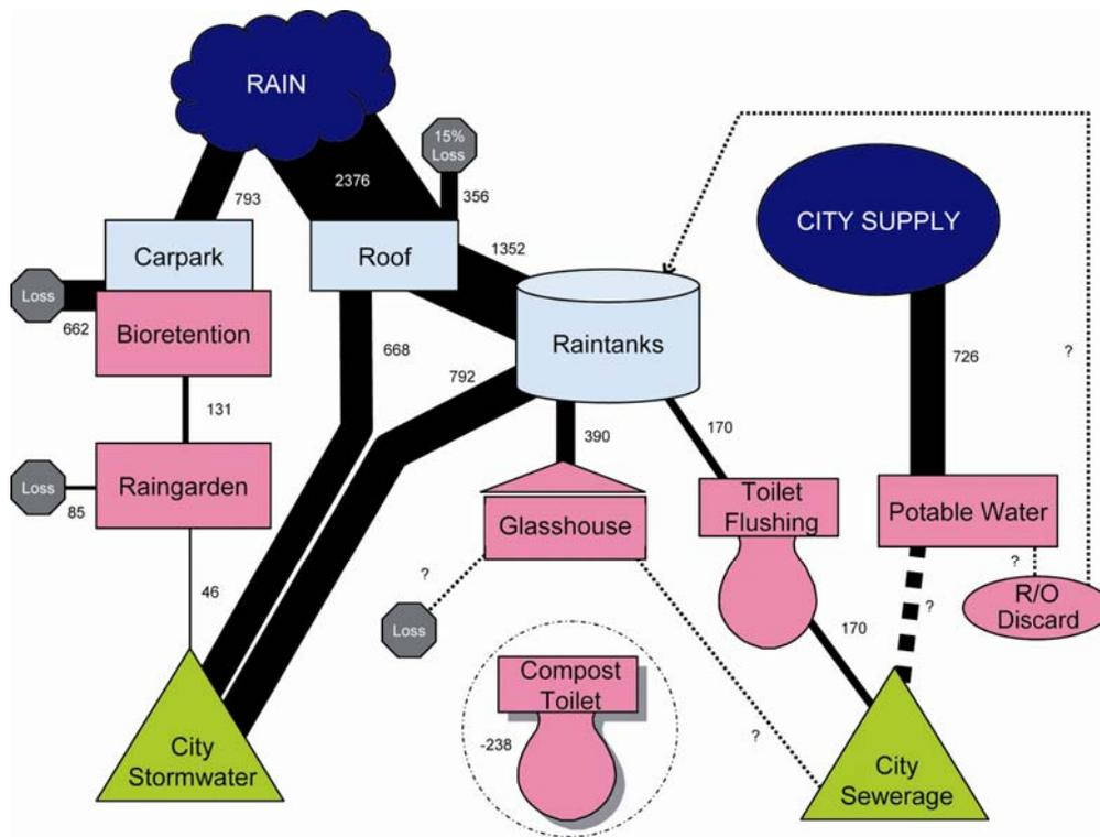
Figure 1 Water balance of the Landcare Research Tamaki Building. The thickness of the lines is proportional to the magnitude of flows, which are labelled and have the units  $m^3$ / year ending 25 July 2007.
