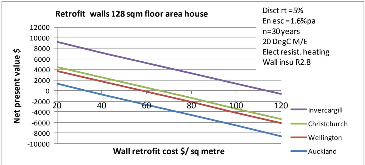
**Figure 10. Wall retrofit cost and NPV**
