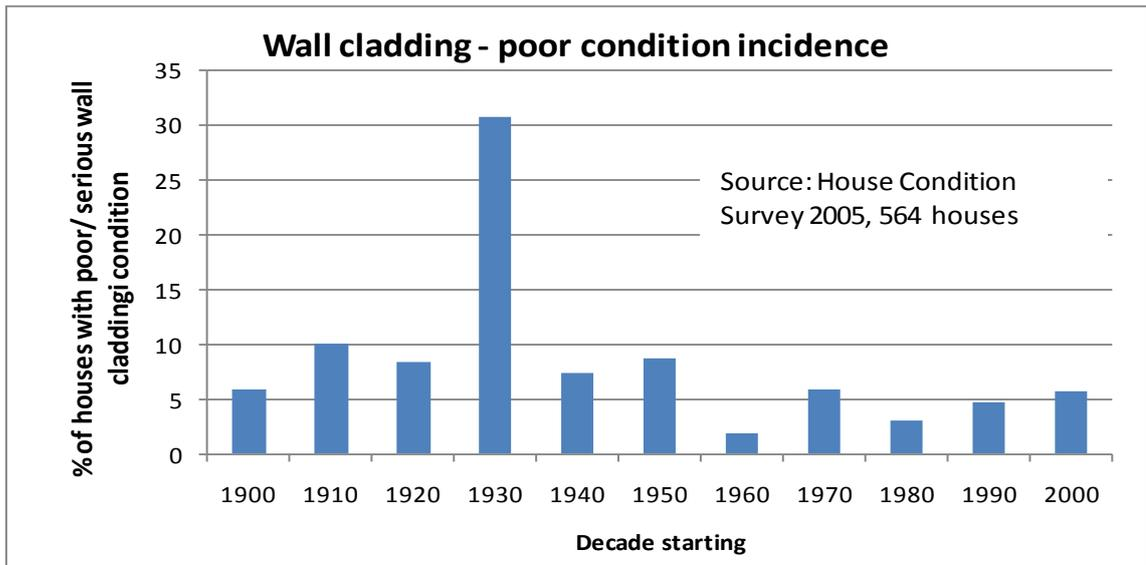
**Figure 2. Wall cladding condition by age of house**
