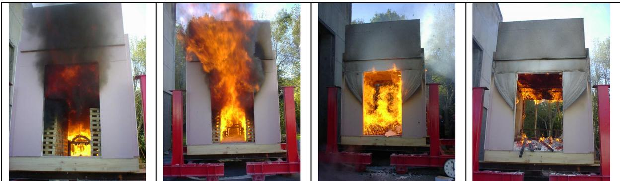
**Figure 10: Compartment fire to assess performance of 'fire-rated system' to non-furnace fires**
