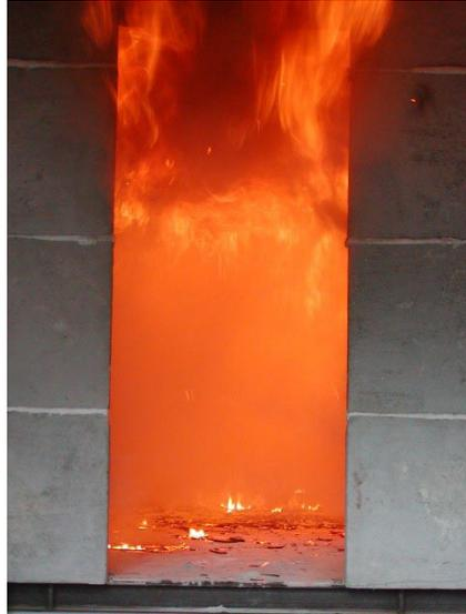
**Figure 3: Flashover in the ISO 9705 room/corner test**
