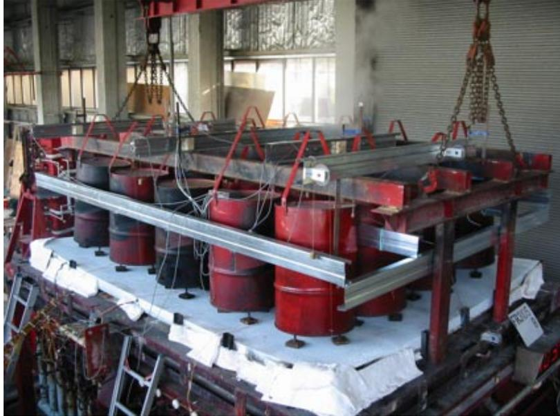
**Figure 9: Fire resistance test of a concrete floor using water-filled drums to simulate gravity loads on the floor**
