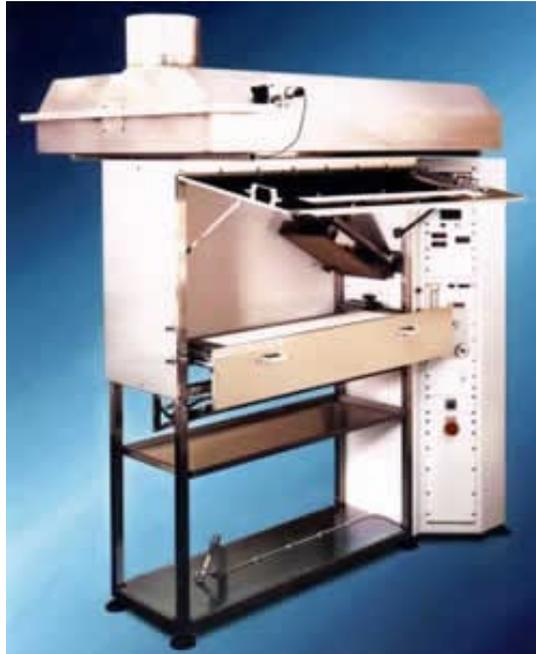
Figure 5: Floor radiant panel apparatus (courtesy, Fire Testing Technology Ltd)
