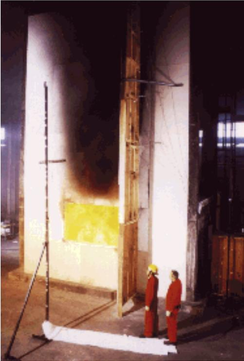
**Figure 6: Full-scale façade fire test at the National Research Council Canada**
