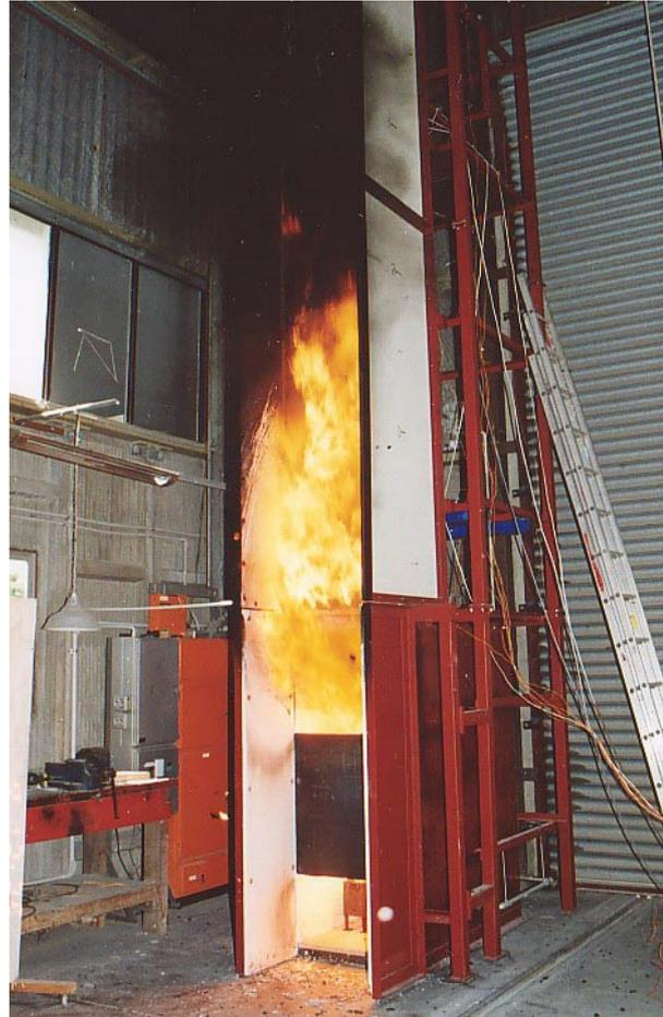
**Figure 7: Vertical Channel Apparatus at BRANZ**
