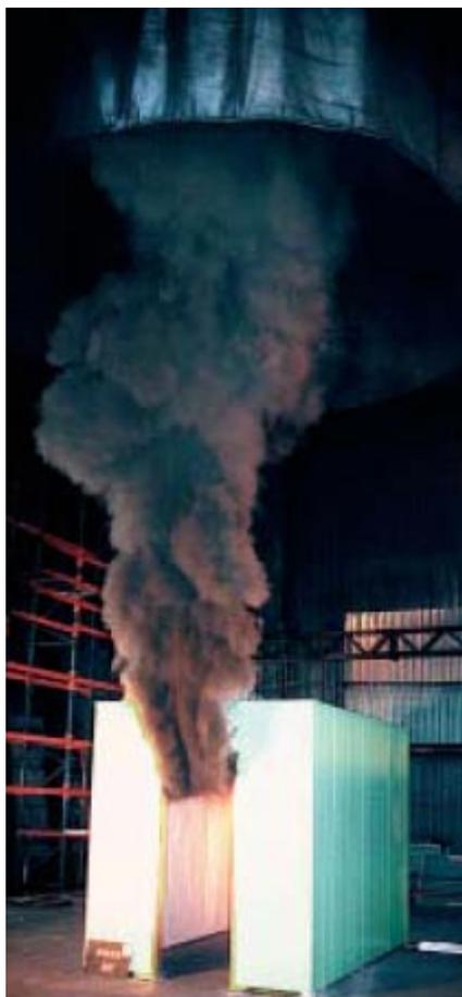
**Figure 8: Fire testing of free-standing room built from sandwich panel in accordance with ISO 13784 (photo SP, 2001)**
