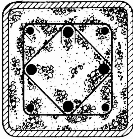
Figure 12 Concrete filled hollow columns
