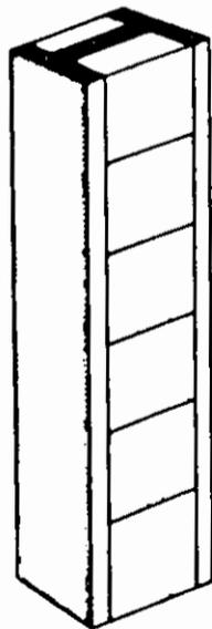
Figure 14 Lightweight masonry infill to universal columns
