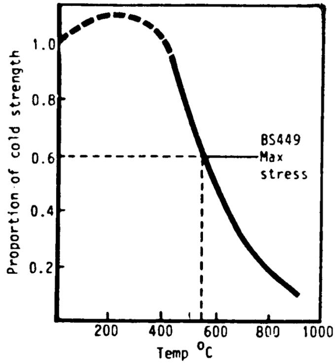
Figure 4 Variation of yield strength of structural steel with temperature
