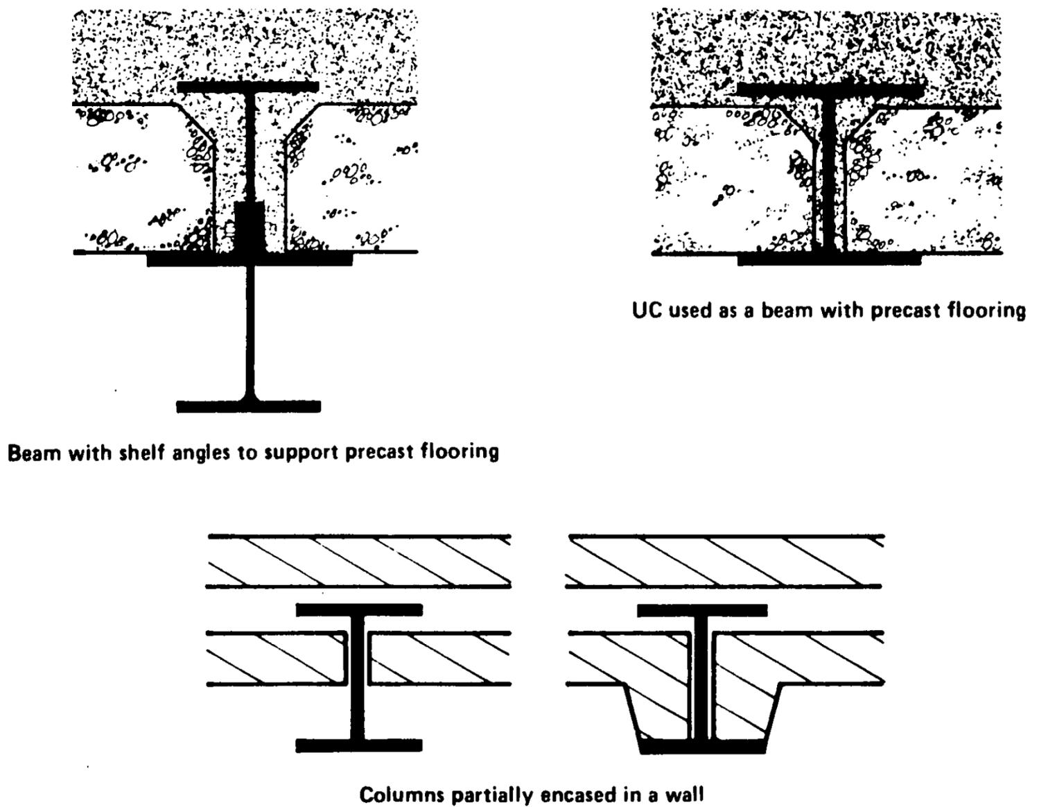
Figure 11 U.K. Construction details which extend fire resistance
