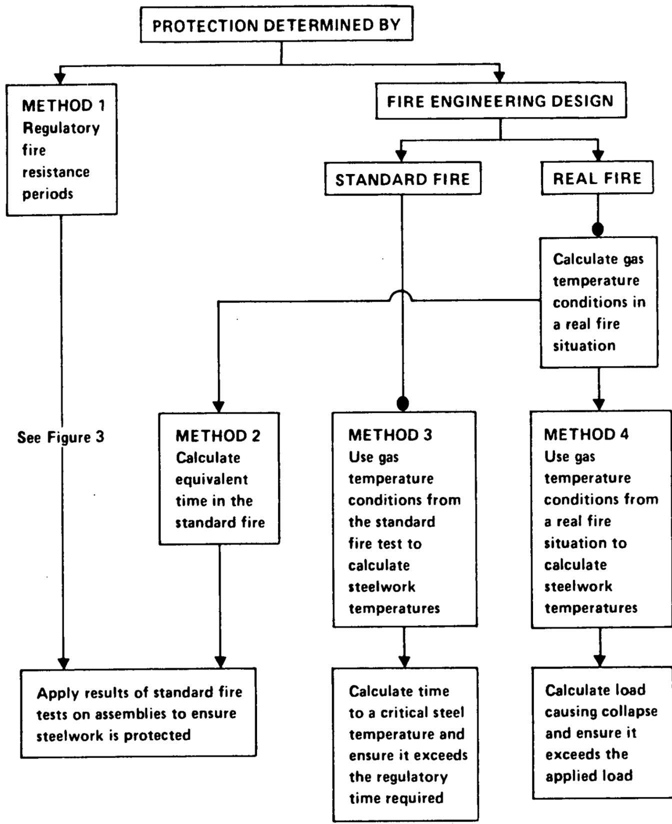
Figure 1 Alternatives available for determining fire protection of steelwork
