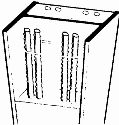
Figure 13 Concrete filled universal columns
