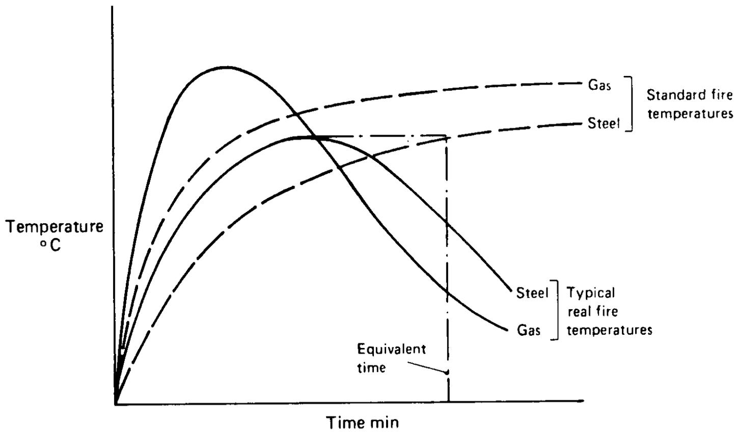
Figure 2 Standard and Real Fire Temperatures, and the Equivalent Time of Method 2.
