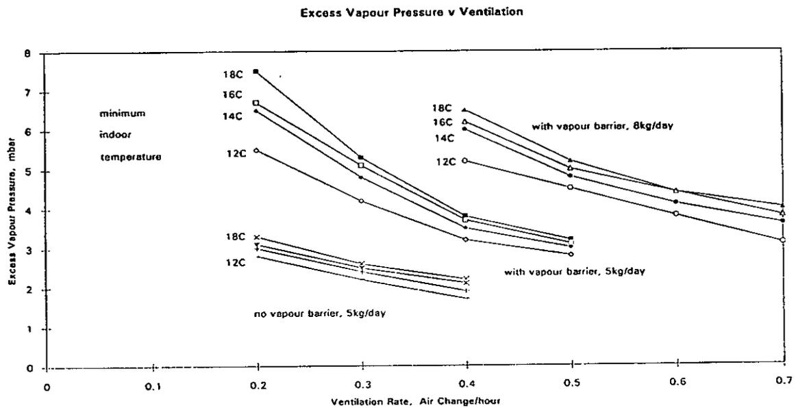
Figure 3. Predicted indoor vapour pressures, from stepwise simulation
