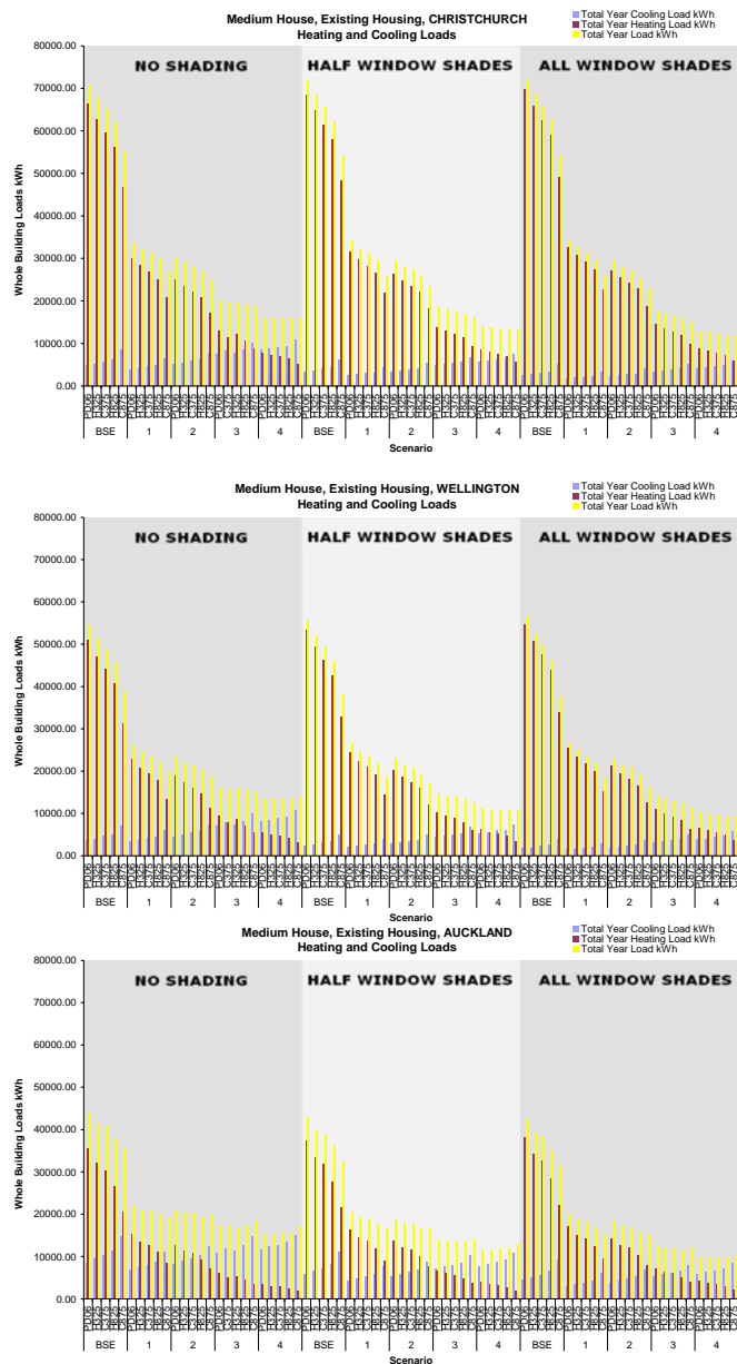
Figure 2: Sample of simulation output for cooling and heating energy consumption for five climate scenarios, three shading options and five insulation levels (No insulation, single glazing = BSE; Ceiling Insulation only, Double Glazing = 1; Ceiling and Floor Insulation only, Double Glazing = 2; Ceiling, Wall, Floor Insulation, Double Glazing = 3; and Best Ceiling, Wall and Floor Insulation, Double glazing with LowE argon filled, thermal break aluminium frame = 4).
