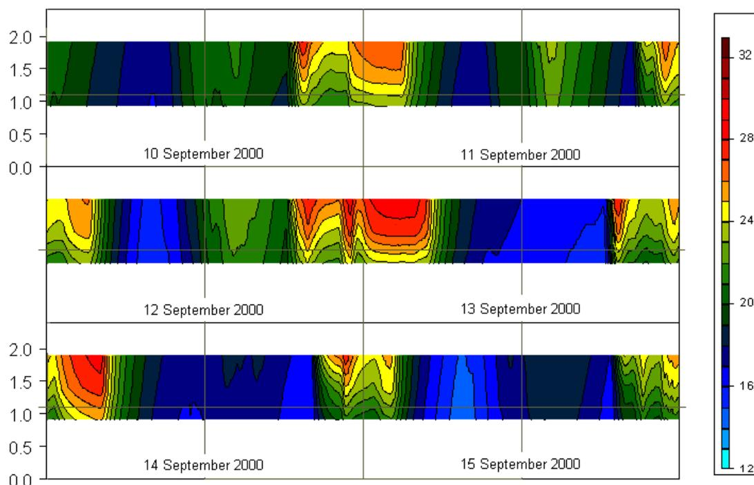
**Figure 5: Vertical temperature profile, living room southeast corner, 2000**
