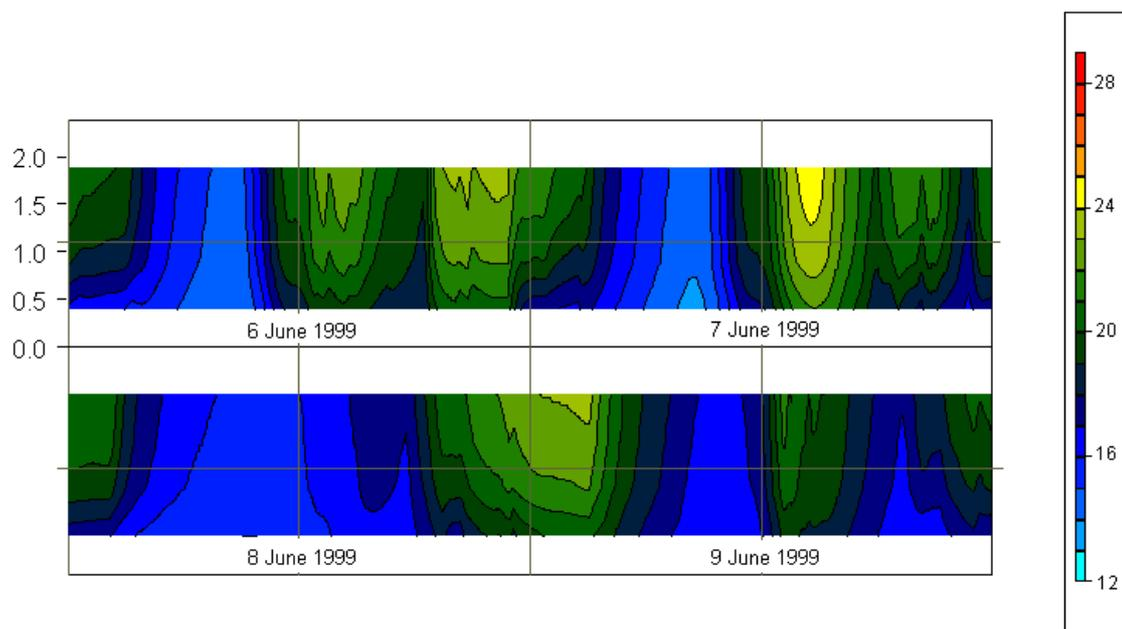
**Figure 4: Vertical temperature profile, living room southeast corner, 1999**
