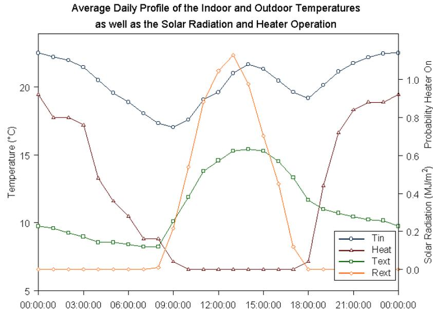
**Figure 3** Average daily profile of the measurements shown in Figure 2
