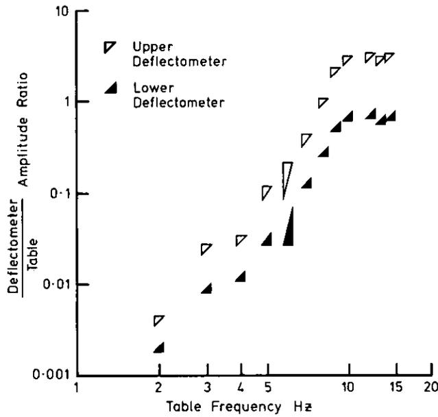
Fig.3 Frequency response for cylinder 50 F.
