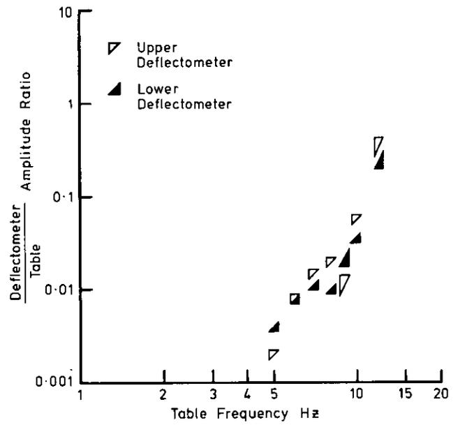
Fig.4 Frequency response for cylinder 50 P.
