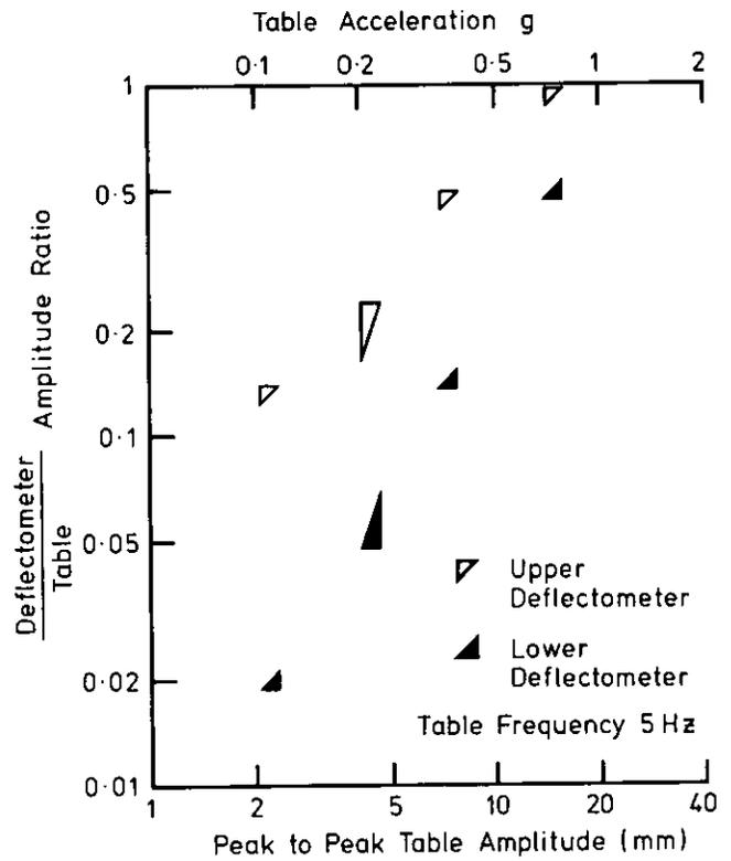
Fig.6 Amplitude response for cylinder 50 F.
