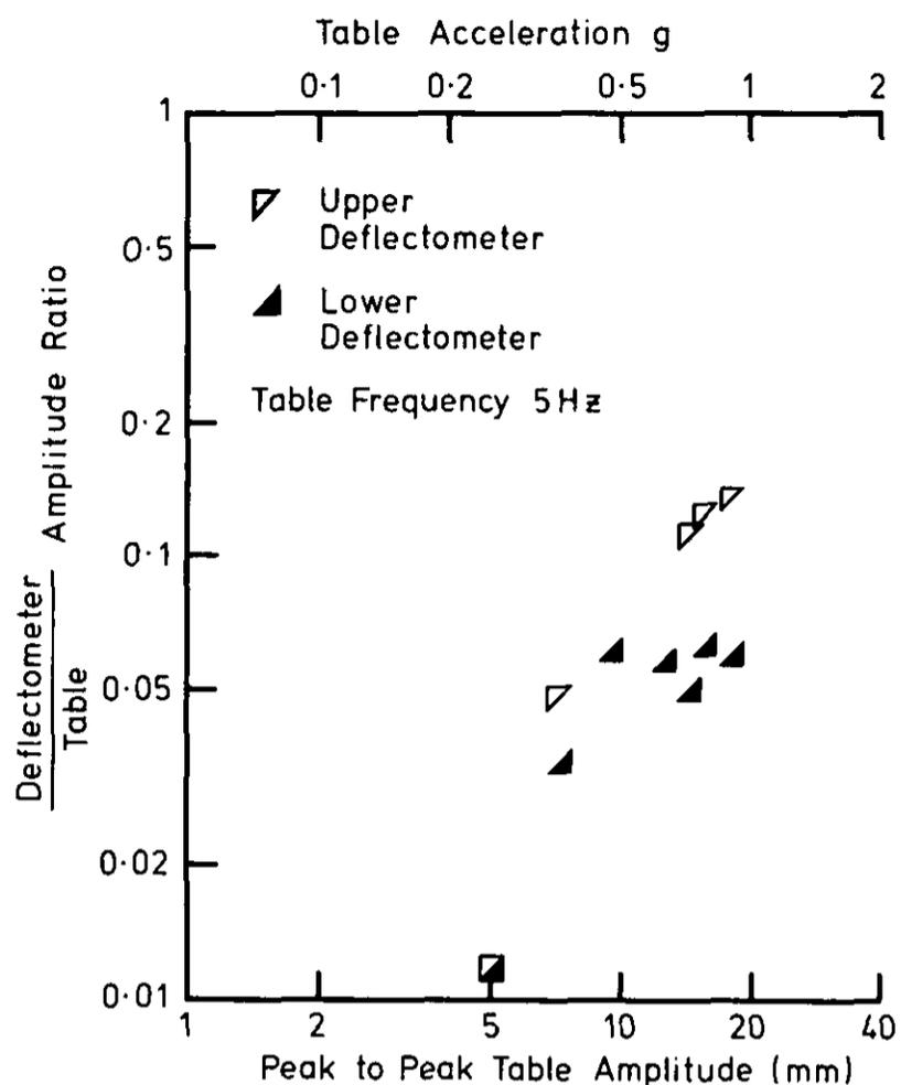
Fig. 7 Amplitude response for cylinder 50 P.
