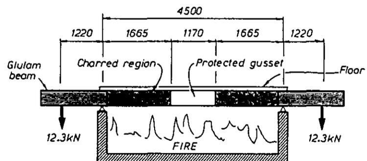
Figure 11. Test set-up for full-scale tests on loaded beams.
