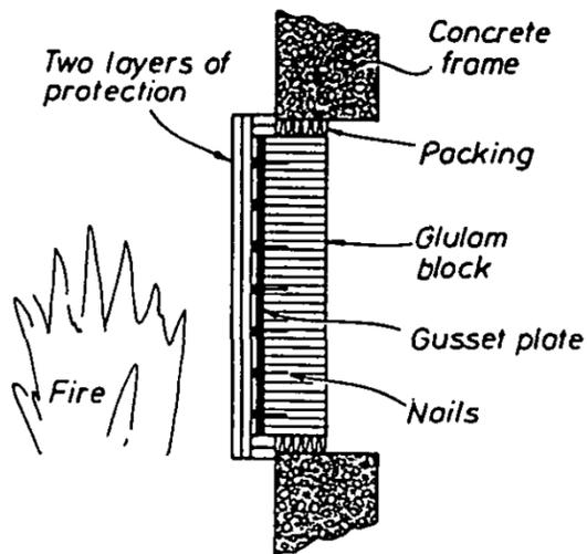
Figure 5. Cross-section through unloaded protected gusset specimen.
