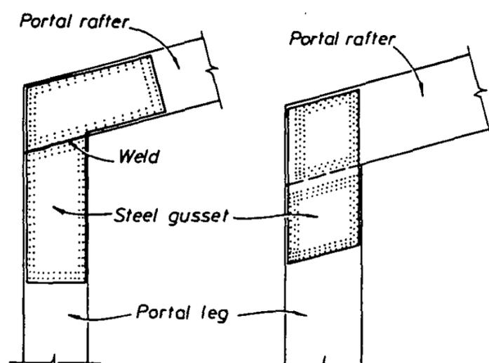
Figure 2. Steel gusset knee joints for portal frame buildings.
