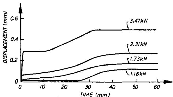
Figure 9. Displacement versus time for steel gusset with four load levels.
