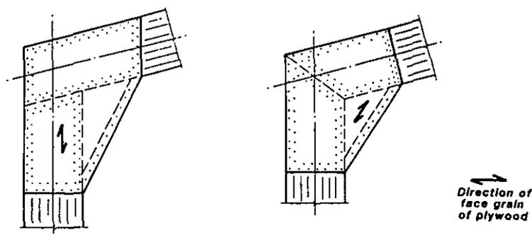
Figure 3. Plywood gusset knee joints for portal frame buildings.
