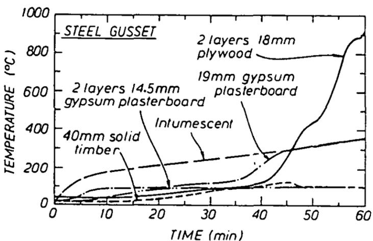
Figure 6. Temperatures measured behind the surface protection for plywood and steel gussets.
