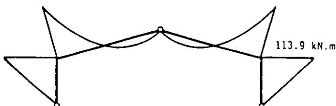
Figure 13. Bending moment diagram for portal frame.
