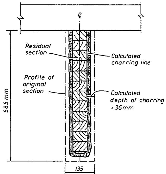
Figure 14. Cross-section of glulam beam before and after one hour of fire exposure.
