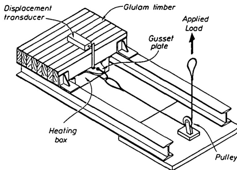
Figure 7. Testing arrangement showing steel gusset being tested.
