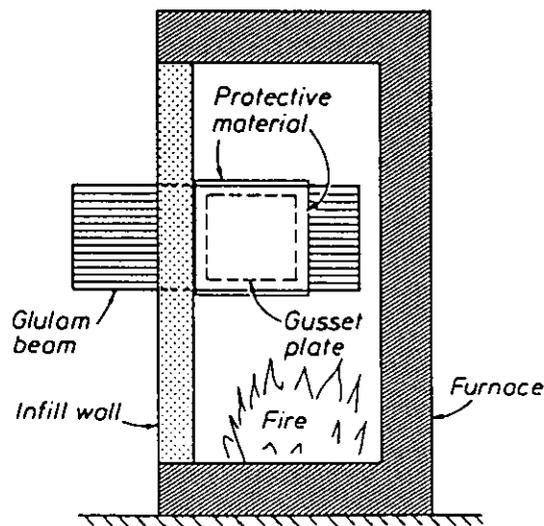
Figure 12. Cross-section through pilot furnace, showing revised detail for testing unloaded specimens.
