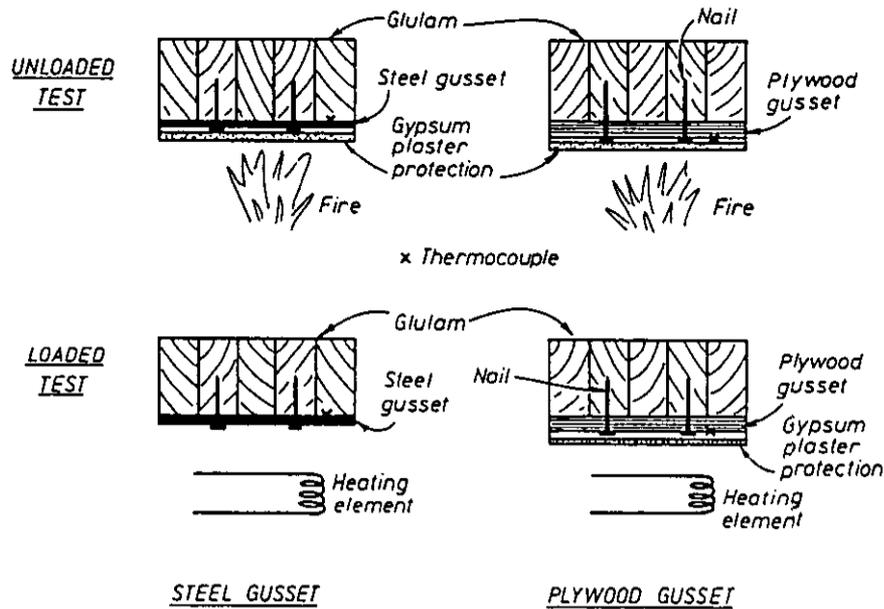
Figure 8. Comparison of heating conditions in unloaded and loaded tests.
